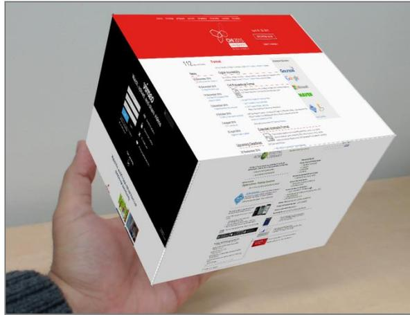
**Figure 9:** A physical cube-shaped object that is textured with web pages in each side (with AR). Users can physically rotate or manipulate the cube to view different webpages in every side.
