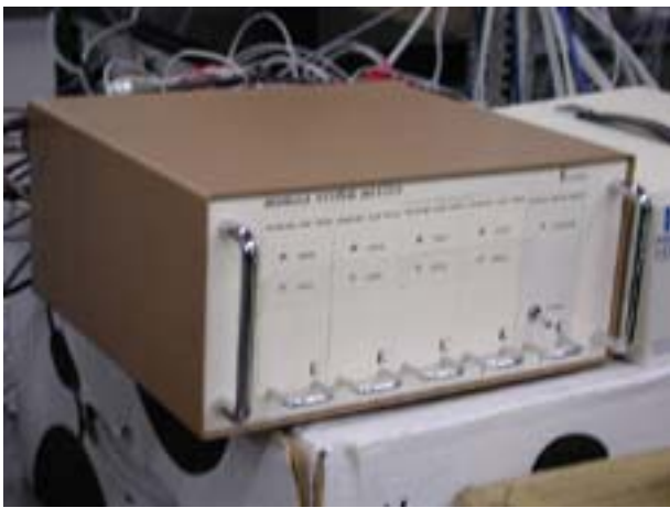
Fig. 3-7a Demodulator for analog output of pressure
