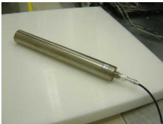
Figure 8.9: ^3\text{He} proportional counter.
