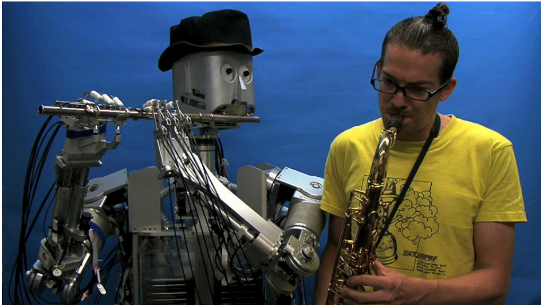
Figure 6.1: In this screenshot a passive performance between the flutist robot WF-4RV and a human musician is displayed. The robot does not react to the play of the human musician. It plays a static score that is being sent from a MIDI sequencer.
