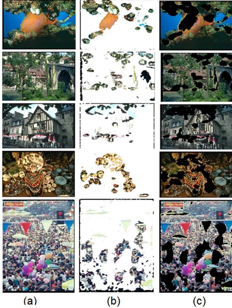
Figure 3.12: Example showing some complex images that result in failure in salient regions and background extraction: (a) the original image, (b) the extracted salient regions and (c) the extracted background.
