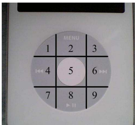
Figure 8-1. Keypad layout of iPod clickwheel
