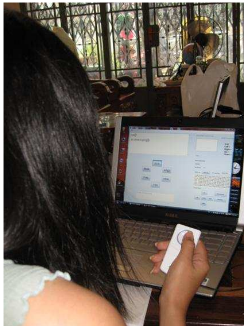
Figure 8-6 User study with PP_Clickwheel prototype
