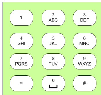
Figure 3-2. Standard ISO 12-key keypad layout
