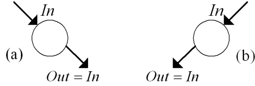
Figure 4.4: Additional data-store cells. (a) move right, (b) move left.
