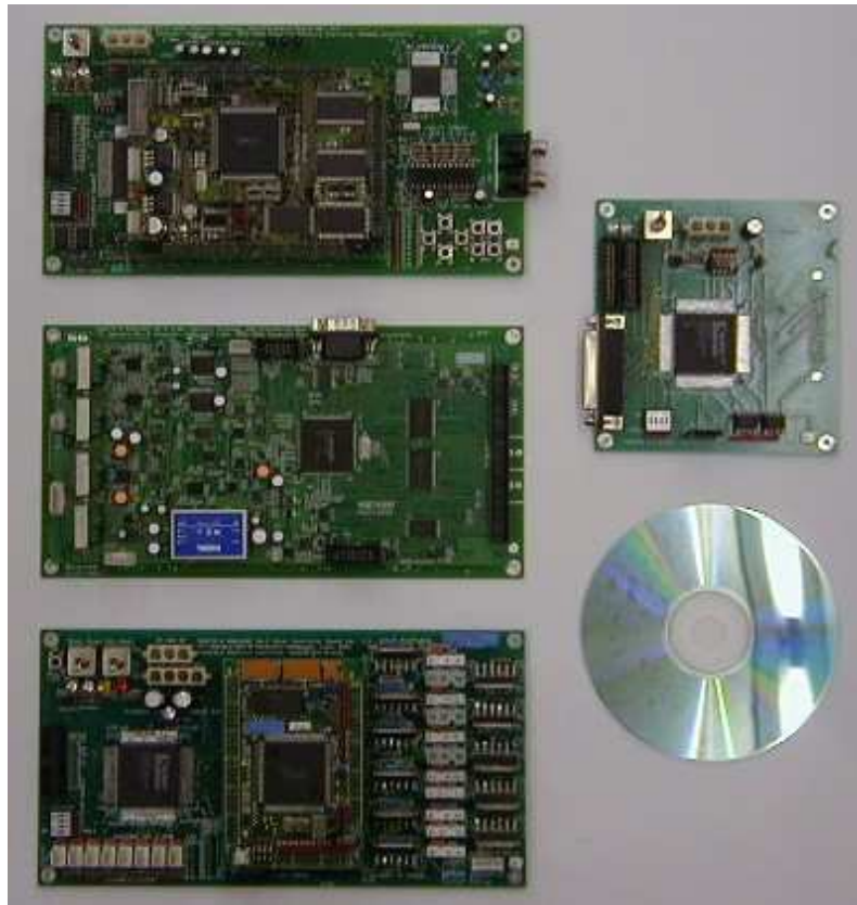
(b) Embedded processor boards and bus bridge.
