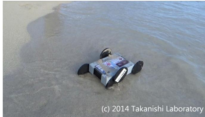
Figure 2.18 WAMOT on sand surface with sea water in seaside
