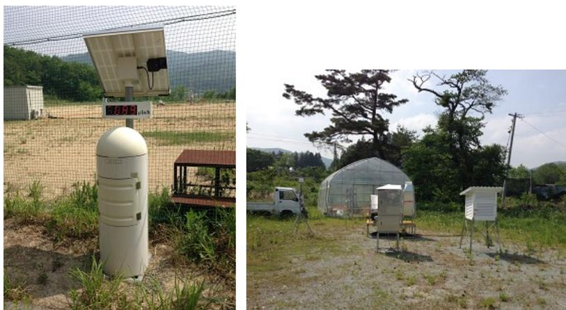
(a) Monitoring post (Radiation level)      (b) Monitoring post (Temperature and humidity)
