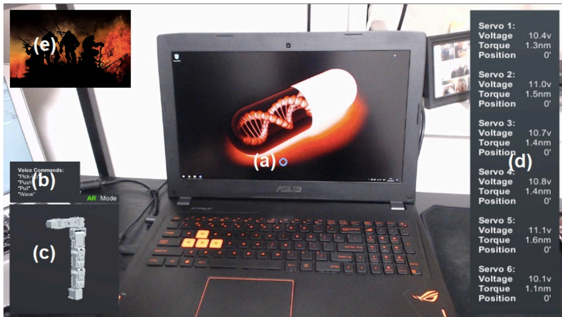
Figure 10 : Interface display showing all available Head-Up Display contents enabled.
