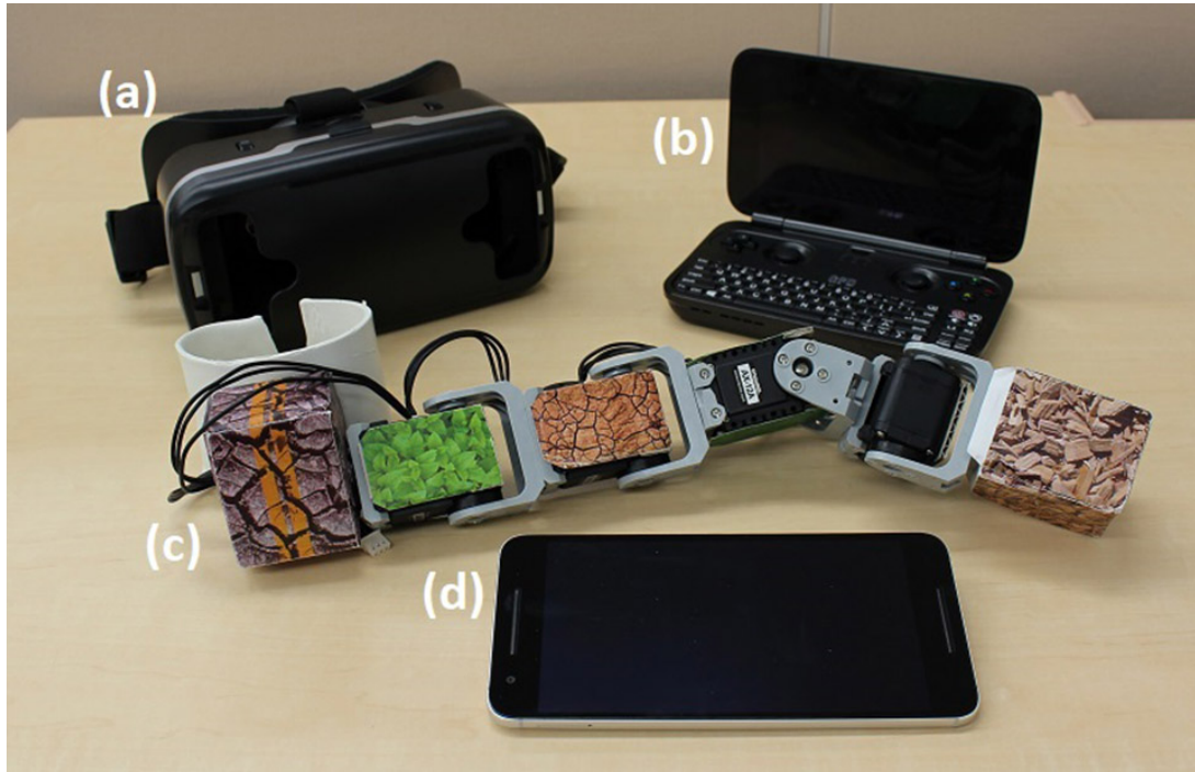
Figure 2 : Fundamental components for our solution: (a) AR enclosure, (b) GPD WIN robot controller, (c) wearable robot with embedded AR markers, and (d) Android smartphone.
