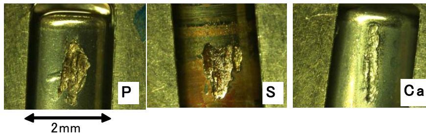
Fig.4-19 Optical photographs on needle tested with oil P, S and Ca
