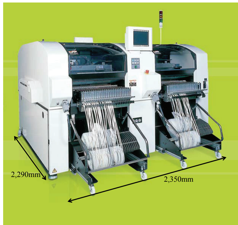
Fig.1-9 Example of the placement machine (CM-402L)
