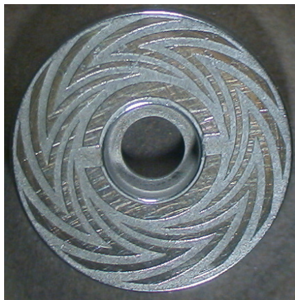
Fig.5-14 Example of the thrust plate with the herringbone type groove
