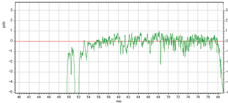
Fig.4-25 Surface profile of the carriage raceway of the A3-Zn+Mo grease
