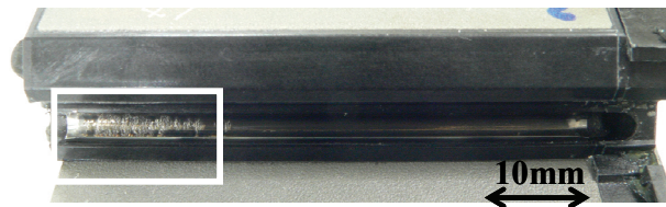
Fig.4-24 Photograph of the carriage after the run of the A3-Zn+Mo grease( 1.9 \times 10^3 km)
