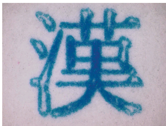
Fig.1-3 Photograph of hollow defects in character image of electrophotography.
