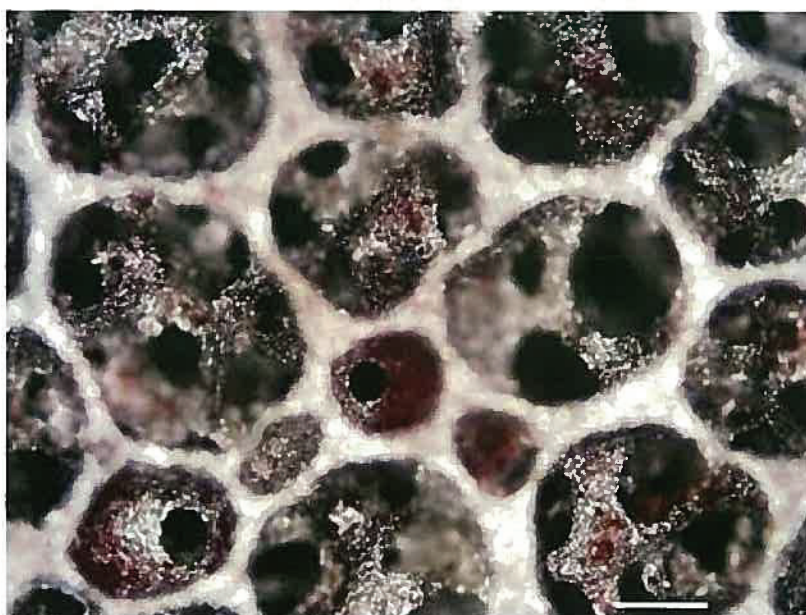
Fig. 4.9. Calcification of SaOS-2 on a single SS foam sheet with open pore size of 270 \mu\text{m} . The calcified area was stained by Alizarin red S (4) . Bar; 200 \mu\text{m} .
