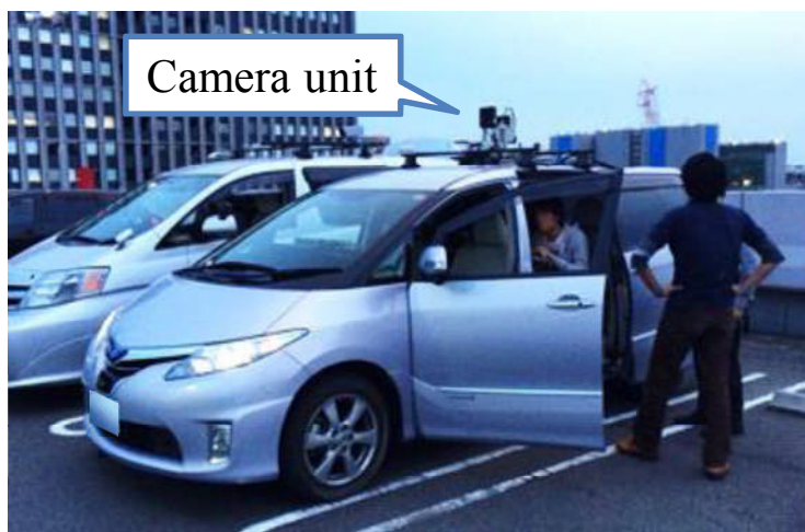
Fig. 3.11 Fish-eye camera and IR-ODV on evaluation test car.
