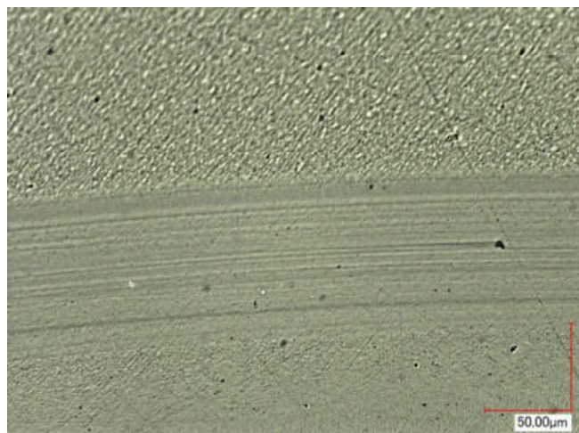
Fig 6.15 Wear track of nitrogen graduated DLC film: Load 19.6N Line speed 100mm/s Sliding distance 200 m
