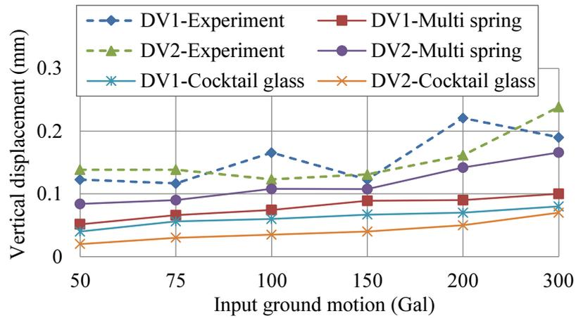
**Fig.5.31** Maximum vertical displacement of the pile cap at DV1 and DV2 in the flat model from 50 to 300 Gal
