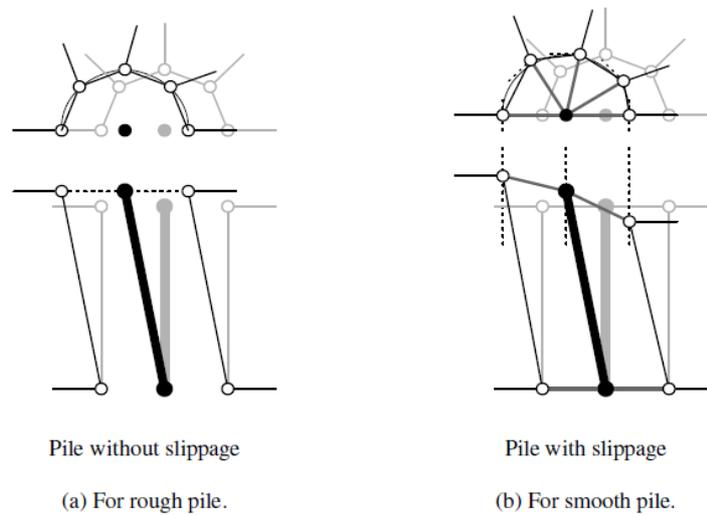
**Fig.2.22** Displacements of nodes of solid elements for soil adjacent to beam element for piles
