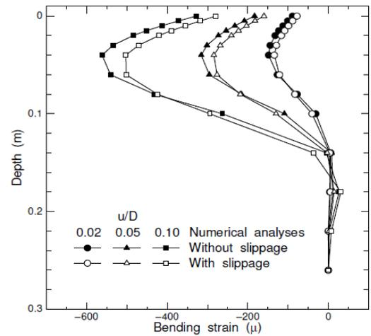
(b) Comparison between the pile with and without slippage.
