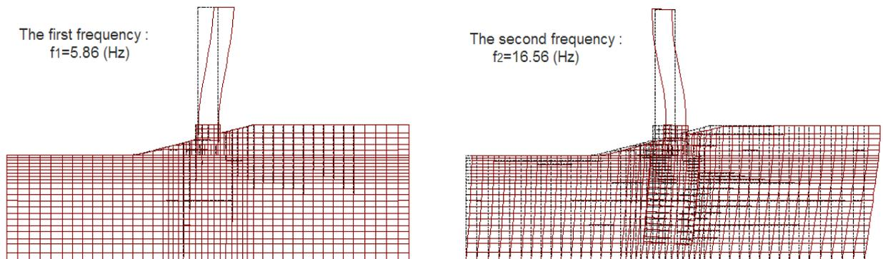
**Fig.4.4** Fundamental natural frequencies of the slope model TSA.
