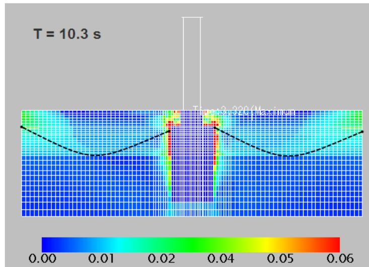
**Fig.5.37** Maximum shear strain distribution in the flat model under 300 Gal
