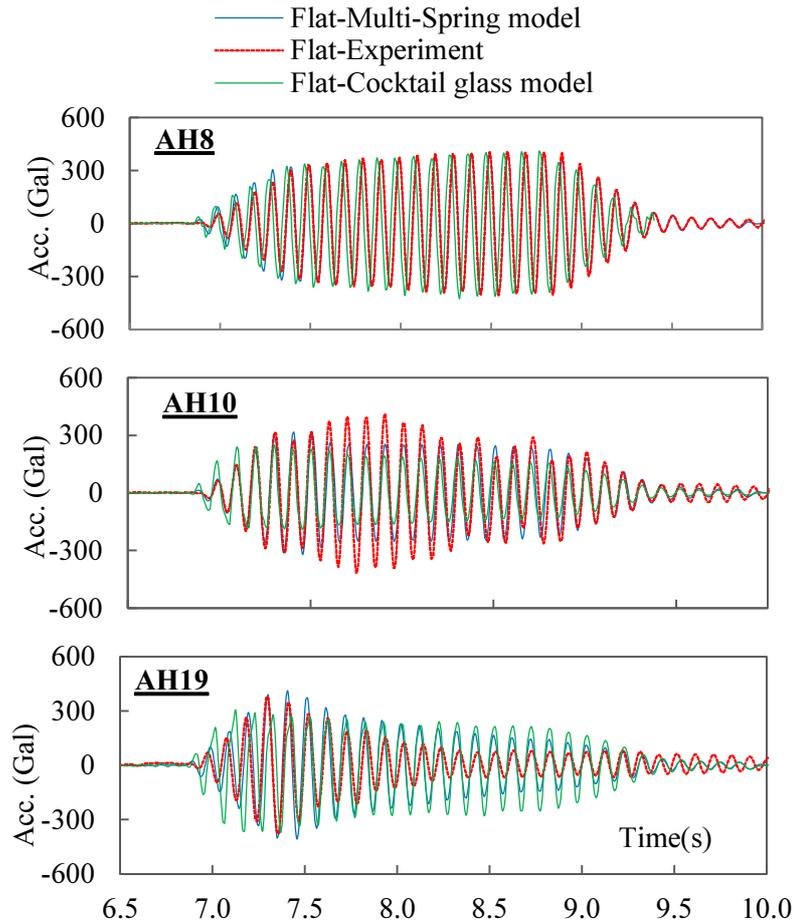
**Fig.5.34** Time history of acceleration at AH8, AH10, AH19 in flat model under 300 Gal. significantly starting at 7.5 s, and this amplitude gradually reduced between 7.5 and 10 s, as shown in **Fig.5.34**.
