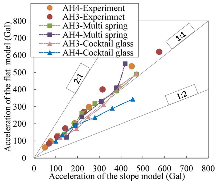
**Fig.5.23** Comparison of acceleration at AH3 and AH4 between the flat and slope models. Moreover, they were in the similar trends with the experiment: in the lower input ground motion the difference of acceleration between two models is minimal; however, in the higher input motion the acceleration response in the slope model was smaller.
