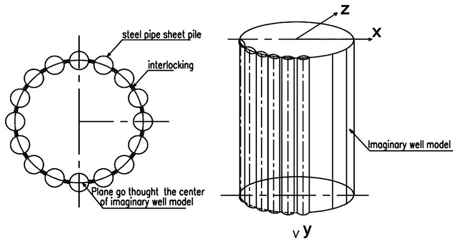
**Fig.2.5** Imaginary well model of SPSP foundation
