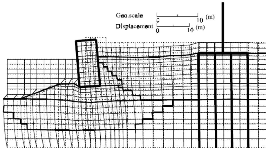
**Fig.1.10** Residual displacement of quay and pile foundation in the Flip program (Sawada and Iai et al. 2000)
