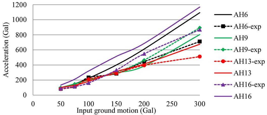
**Fig.4.16** Horizontal acceleration of ground in the slope model in case 300 Gal input motion
