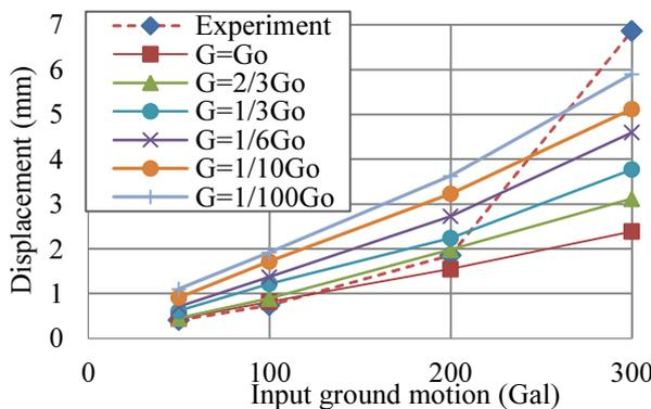
**Fig.4.12** Displacement of superstructure in the slope model.
