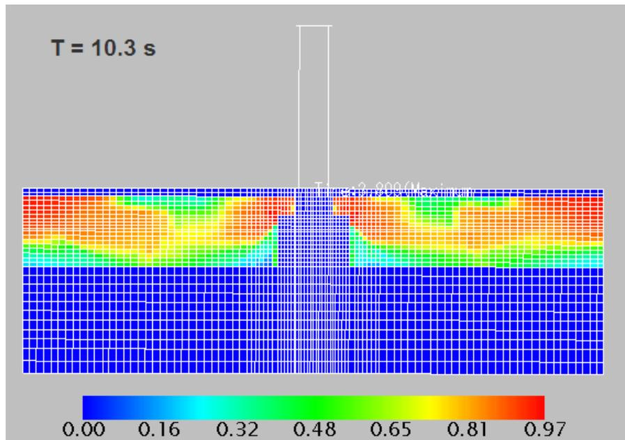
**Fig.5.13** EPWP ratio distribution in flat model under 300 Gal.
