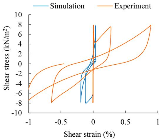
**Fig.5.10** Stress-strain curves from liquefaction parameters
