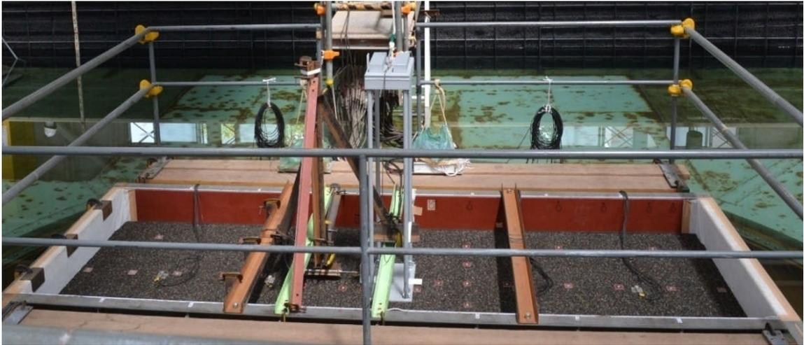
**Fig.3.4** 1-G shaking table test on the flat model
