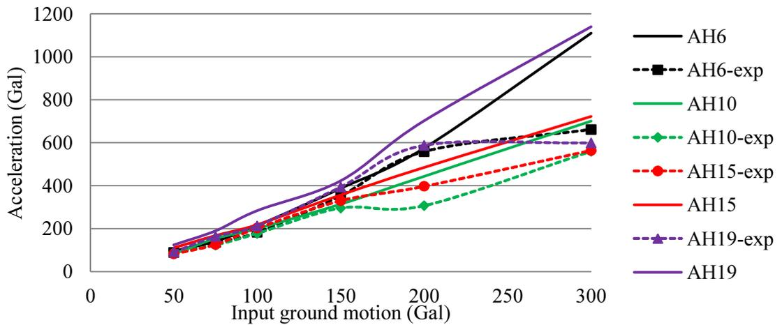
**Fig.4.17** Horizontal acceleration of ground in the flat model in case 300 Gal input ground motion
