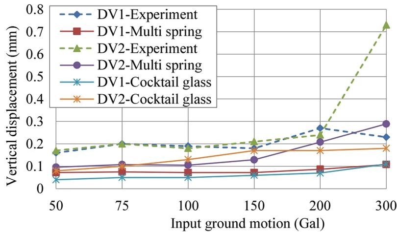
**Fig.5.32** Maximum vertical displacement of the pile cap at DV1 and DV2 in the slope model from 50 to 300 Gal
