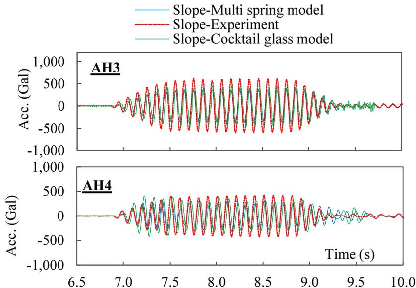
**Fig.5.20** Time history of acceleration at AH3 and AH4 in the slope model under 300 Gal
