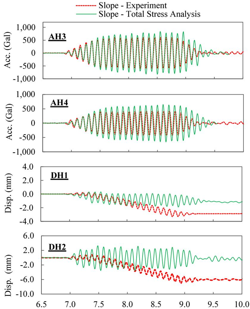
**Fig.4.7** Horizontal displacement and acceleration time histories of 300 Gal of superstructure in case of  $1/6G_0$  in the slope model
