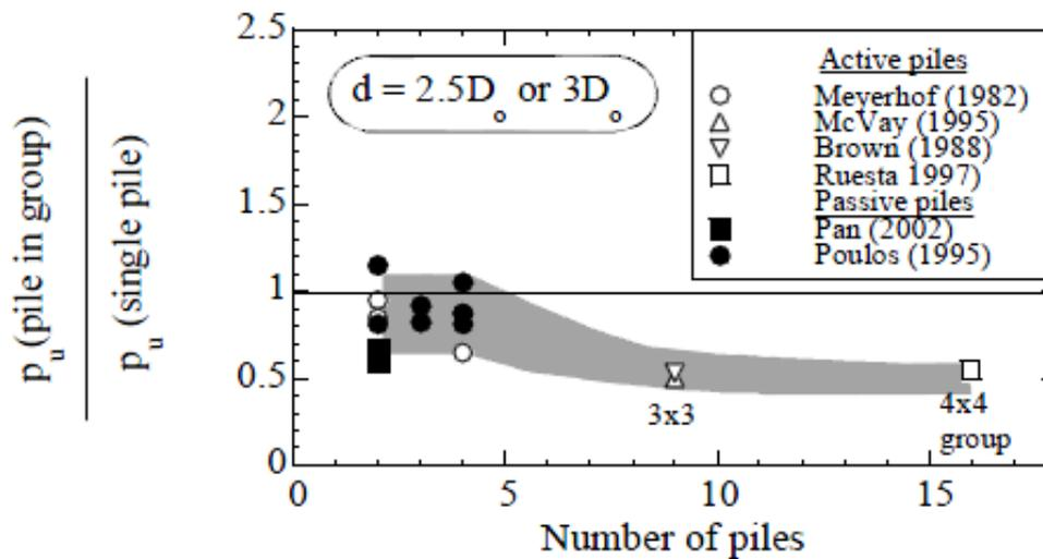
Fig.2.19 Reduction of lateral pressure depends on the number of piles
