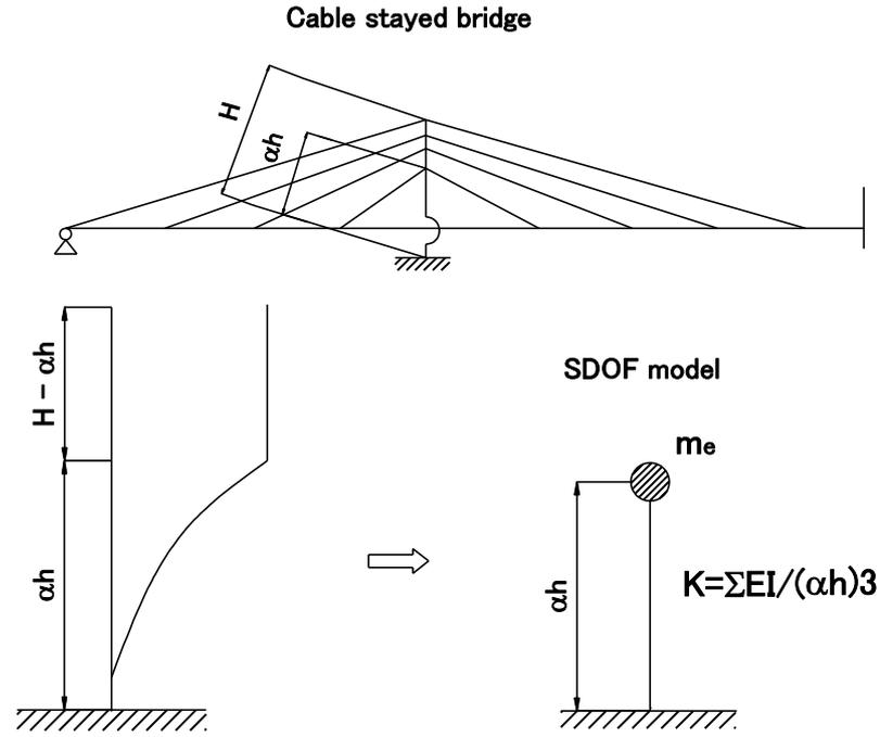
**Fig.3.3** SDOF model of superstructure tower system of a cable stayed bridge (Yoneda et al. 2009)
