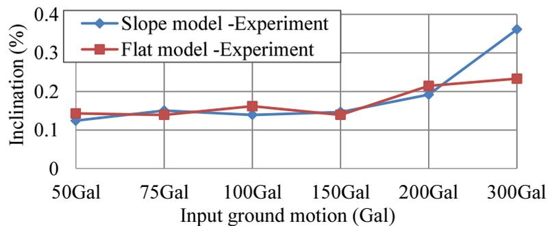
**Fig.3.32** Inclination of foundation in the flat and slope models
