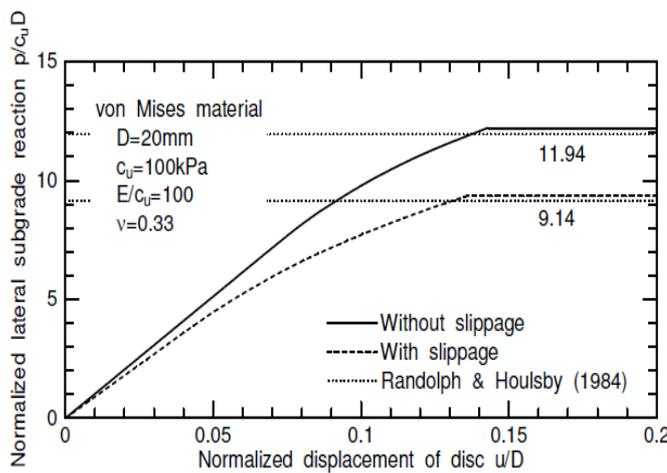
Figure 6.5: Normalized load-displacement relations of disc in von Mises material.
