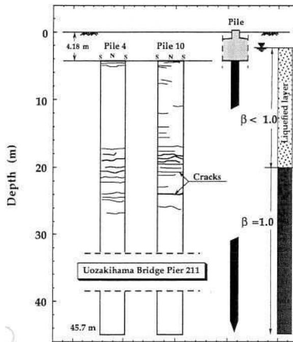
**Fig.1.6** Crack distribution of the large diameter bored piles of pier 211 (Ishihara and Cubrinovski 1998)
