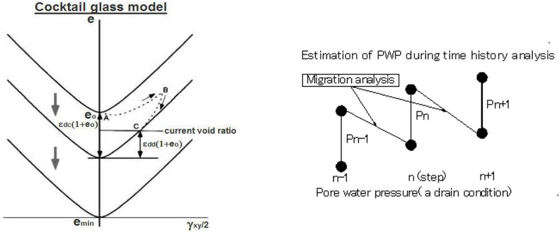
**Fig.5.3** Cocktail glass model in effective stress analysis
