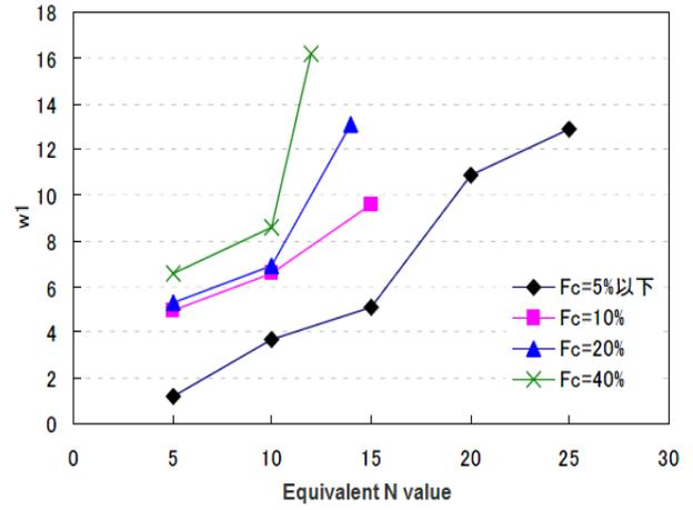
**Fig.5.9** Determination of initial phase of cumulative dilatancy
