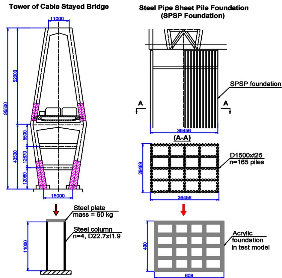
**Fig.3.2** Cable stayed bridge prototype
