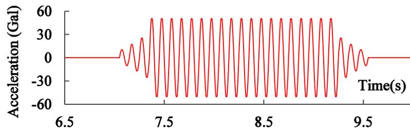
Fig.3.10 Acceleration wave input of 50 Gal at the base.
