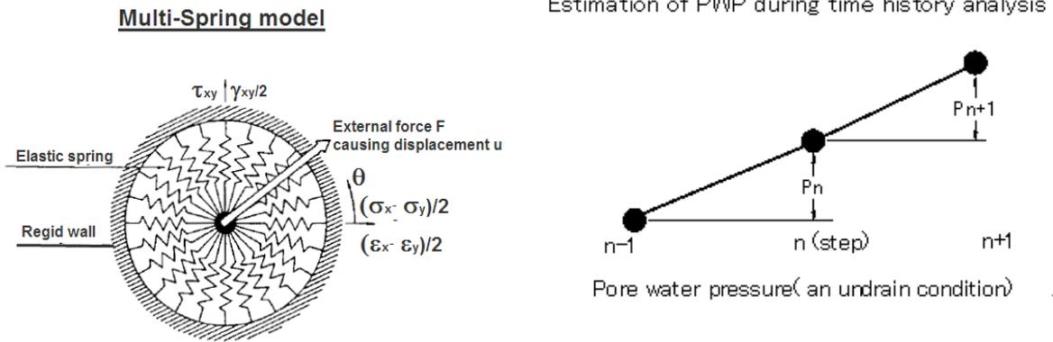
**Fig.5.1** Multi-spring model in effective stress analysis
