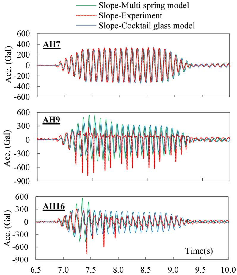
**Fig.5.35** Time history of acceleration at AH7, AH9, AH16 in slope model under 300 Gal.
