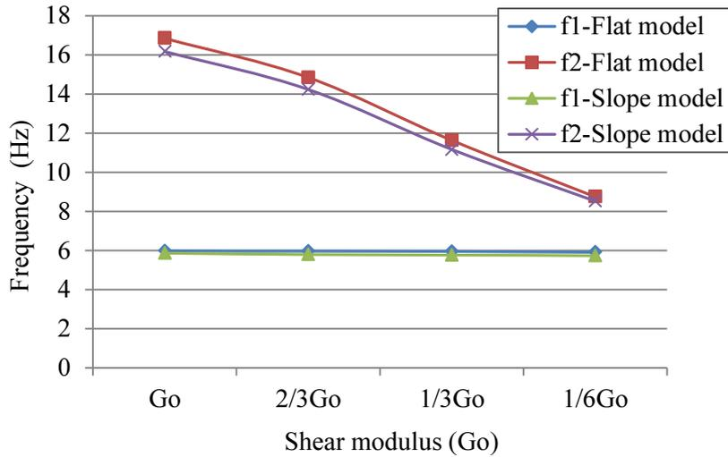
**Fig.4.5a** Fundamental natural frequencies of both models with a reduction of shear modulus
