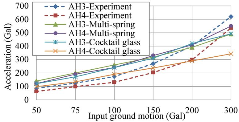
**Fig.5.21** Maximum acceleration of AH4 and AH3 in the flat model from 50 to 300 Gal
