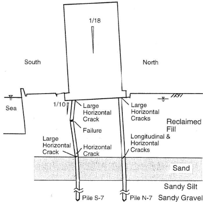
**Fig.1.1** Concept failure patterns of piles due to liquefaction (Tokimatsu et al. 1997)
