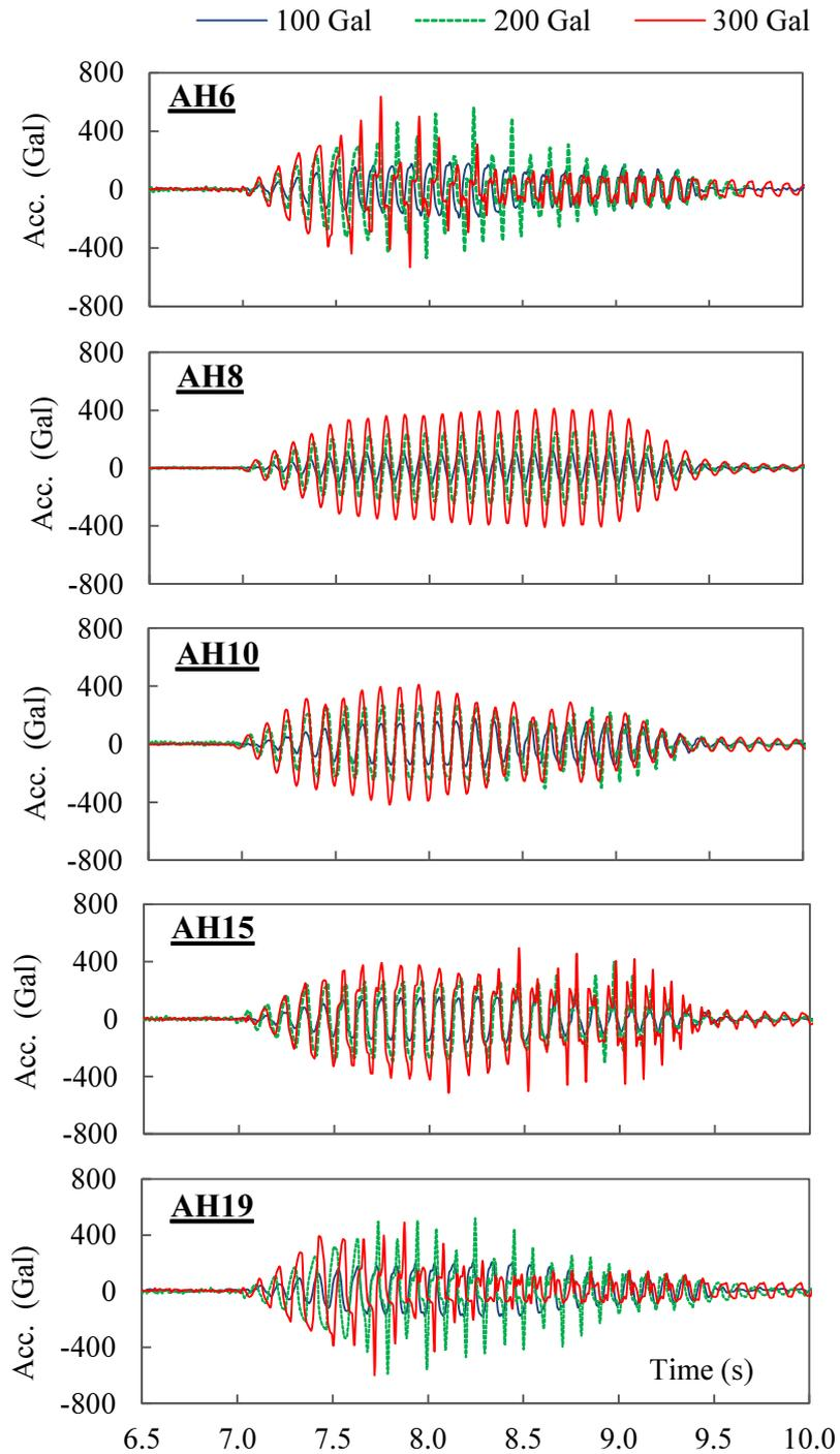
**Fig.3.14** Time histories of acceleration in the flat model from 100 to 300 Gal
