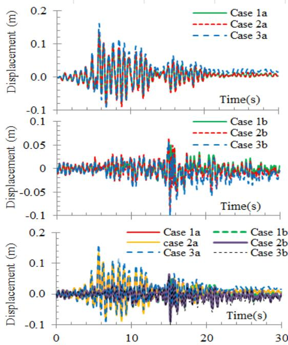
**Fig.2.13** Displacement response at top of pier
