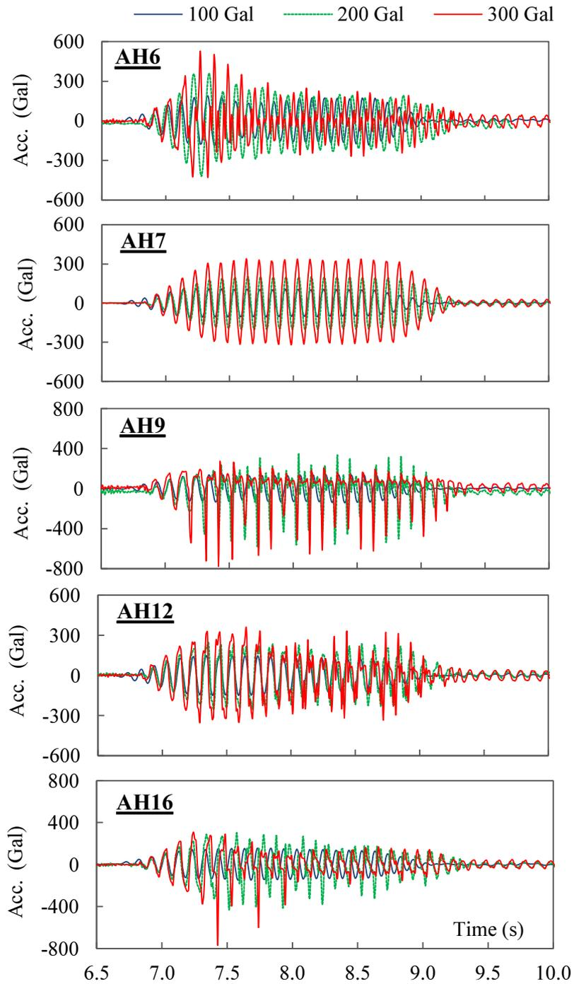
**Fig.3.15** Time histories of acceleration in the flat model from 100 to 300 Gal
