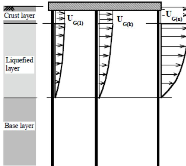
**Fig.2.20** Different lateral pressure on the piles in the group
