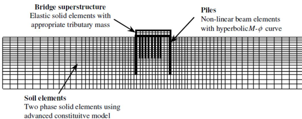
**Fig.1.11** Numerical model of pile foundation (Bowen and Cubrinovski et al. 2007)
