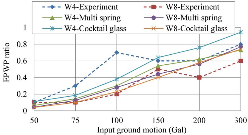
**Fig.5.17** EPWP ratio in the slope model from 50 to 300 Gal
