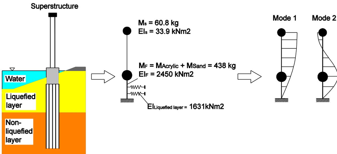
**Fig.4.5b** Double mass system of pier- SPSP foundation system and their modal modes
