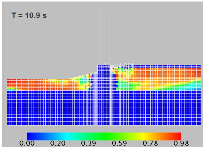
**Fig.5.15** EPWP ratio distribution in slope model under 300 Gal.
