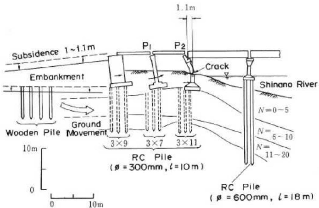
**Fig.1.4** Damage to Yachiyo Bridge due to lateral spreading
