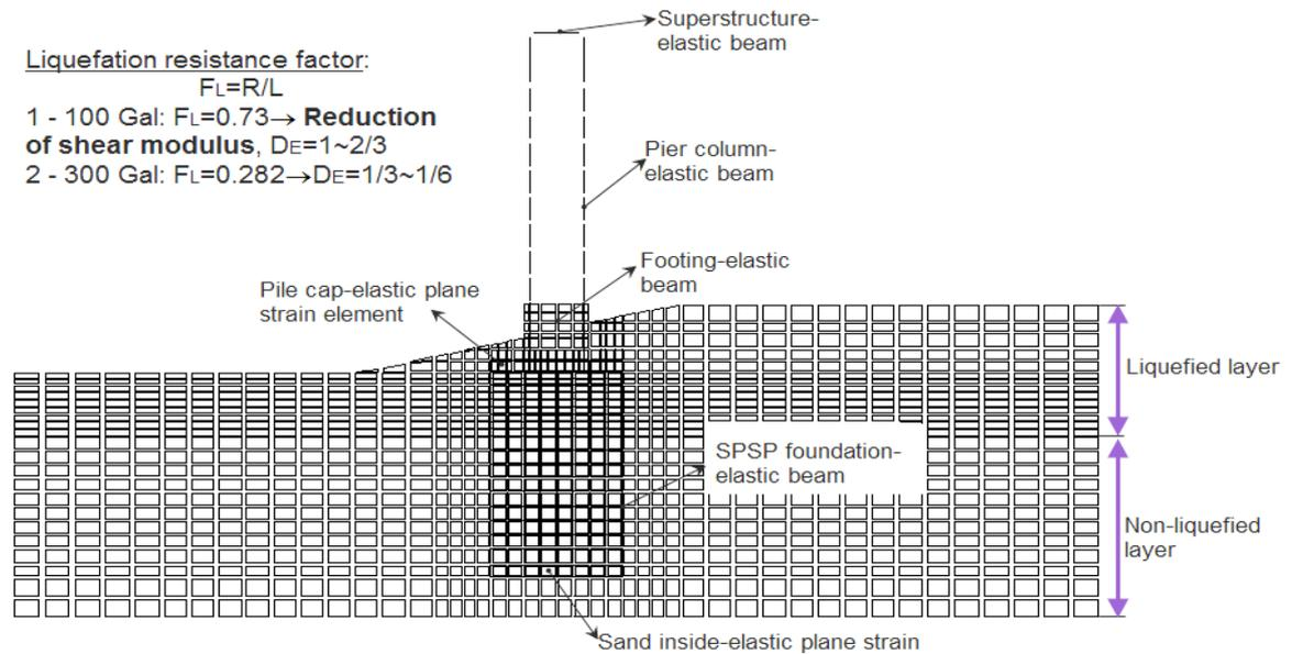
**Fig.4.1** Numerical slope model in Total Stress Analysis (TSA).
