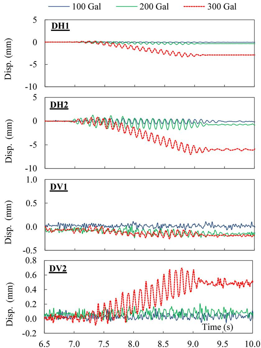
**Fig.3.27** Time histories of displacement of superstructure and pile cap in the slope model
