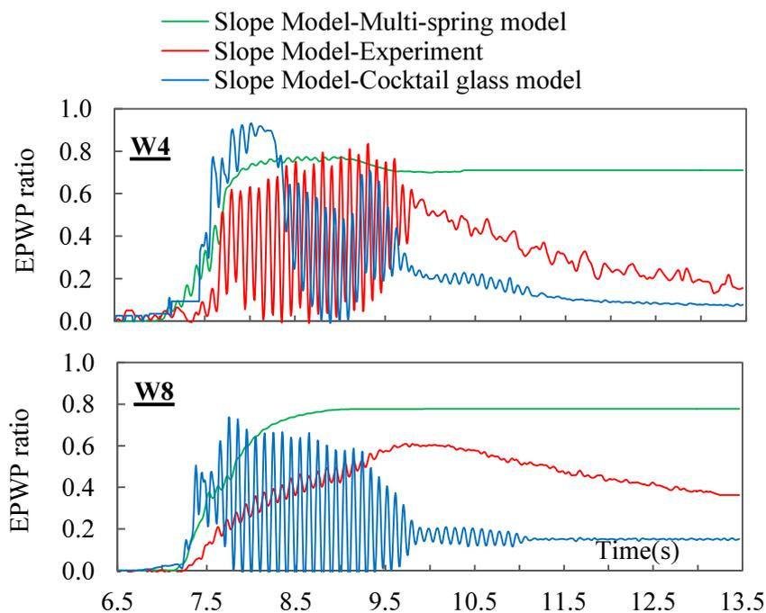
**Fig.5.14** Time history of EPWP ratio at W4 and W8 in the slope model under 300 Gal
