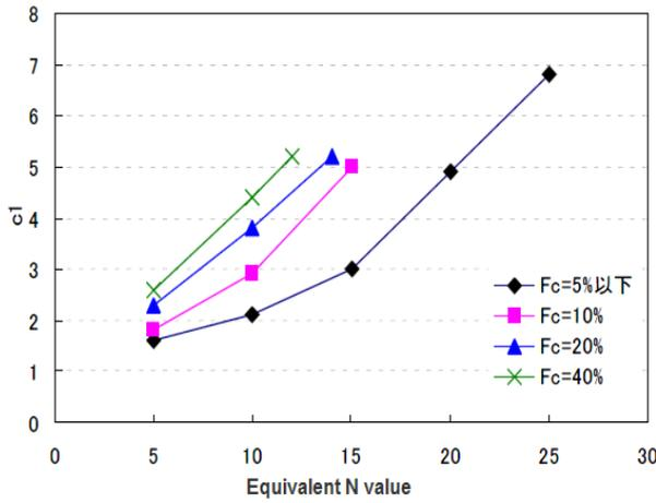
**Fig.5.8** Determination of threshold limit of dilatancy
