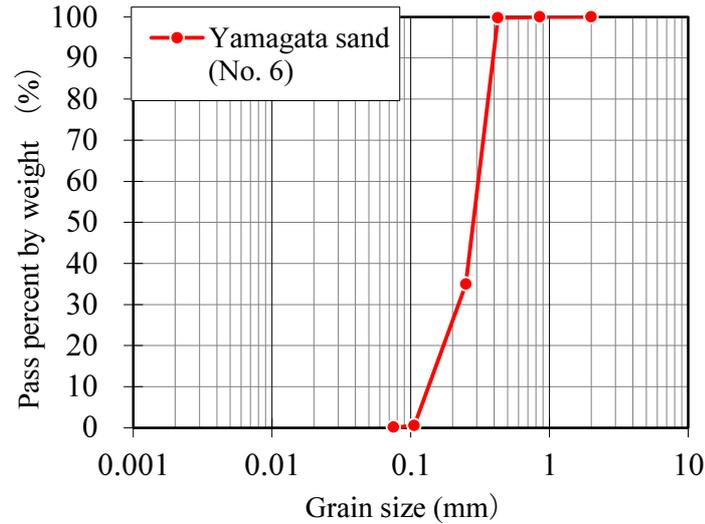
**Fig.3.5** Grain size distribution of Yamagata sand
