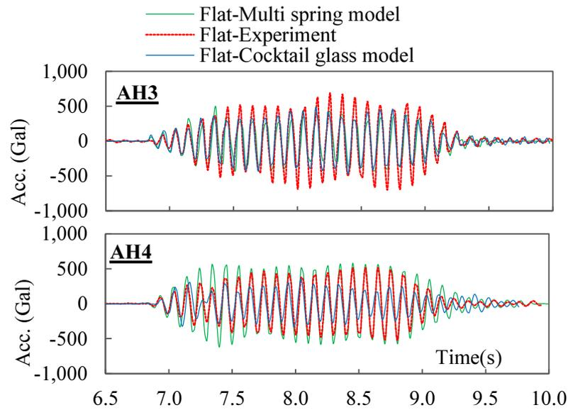
**Fig.5.19** Time history of acceleration at AH3 and AH4 in the flat model under 300 Gal
