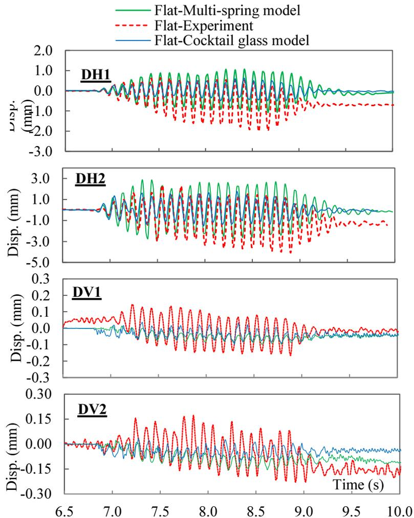
**Fig.5.24** Displacement of superstructure and pile cap in the flat model under 300 Gal
