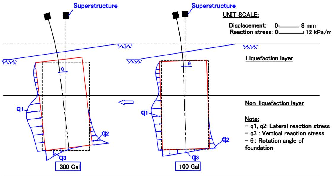
**Fig.5.39** Ground reaction stress distribution of the SPSP foundation in the slope model
