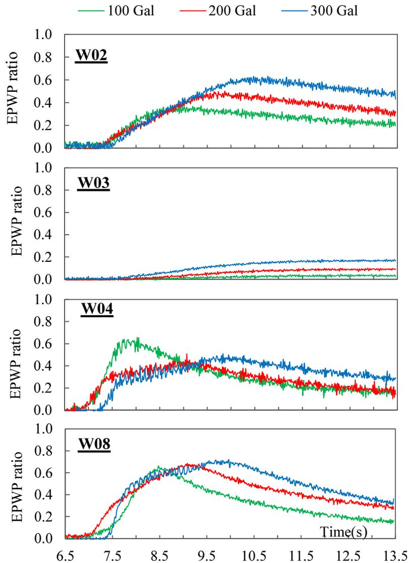
**Fig.3.11** Time histories of pore water pressure in the flat model from 100 to 300 Gal
