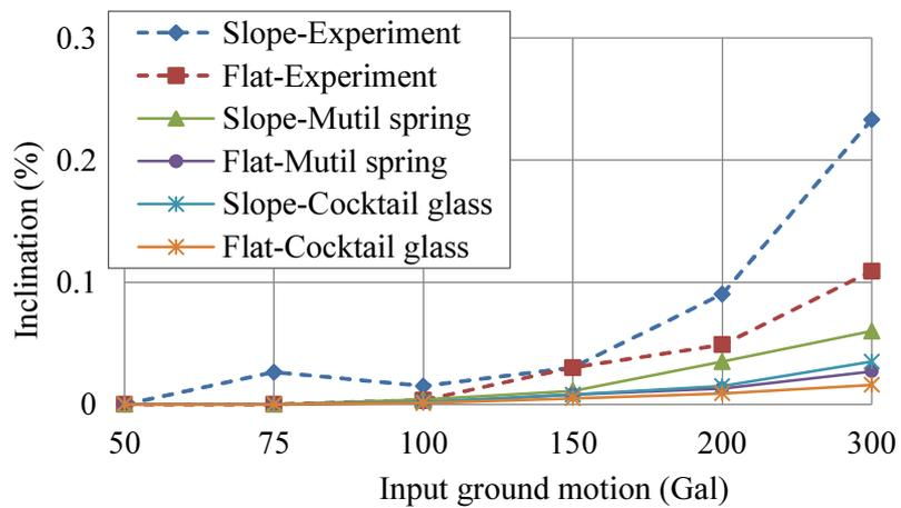
**Fig.5.33** Comparison of the inclination of foundation between the flat and slope models from 50 to 300 Gal
