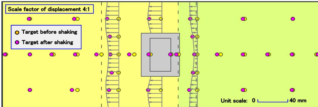
Fig.3.17 The measured displacement distribution of the ground surface movement in the slope model under 300 Gal
