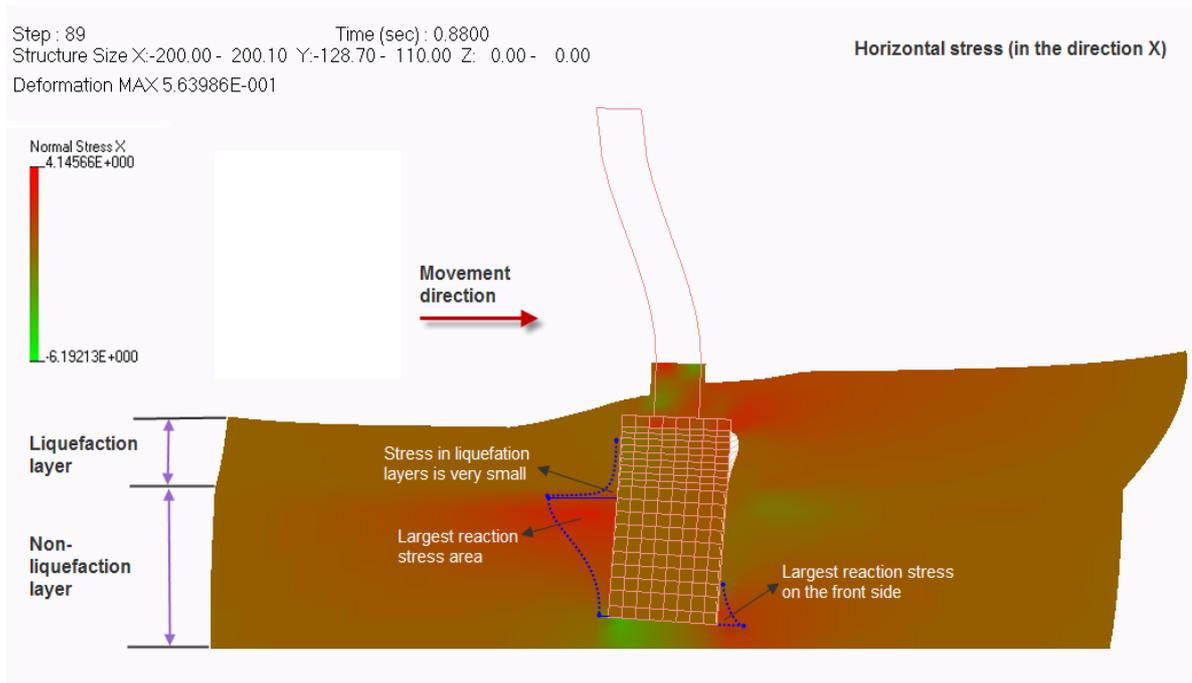
**Fig.4.18** Distribution of horizontal reaction stress in the slope model in case of  $1/6G_0$
