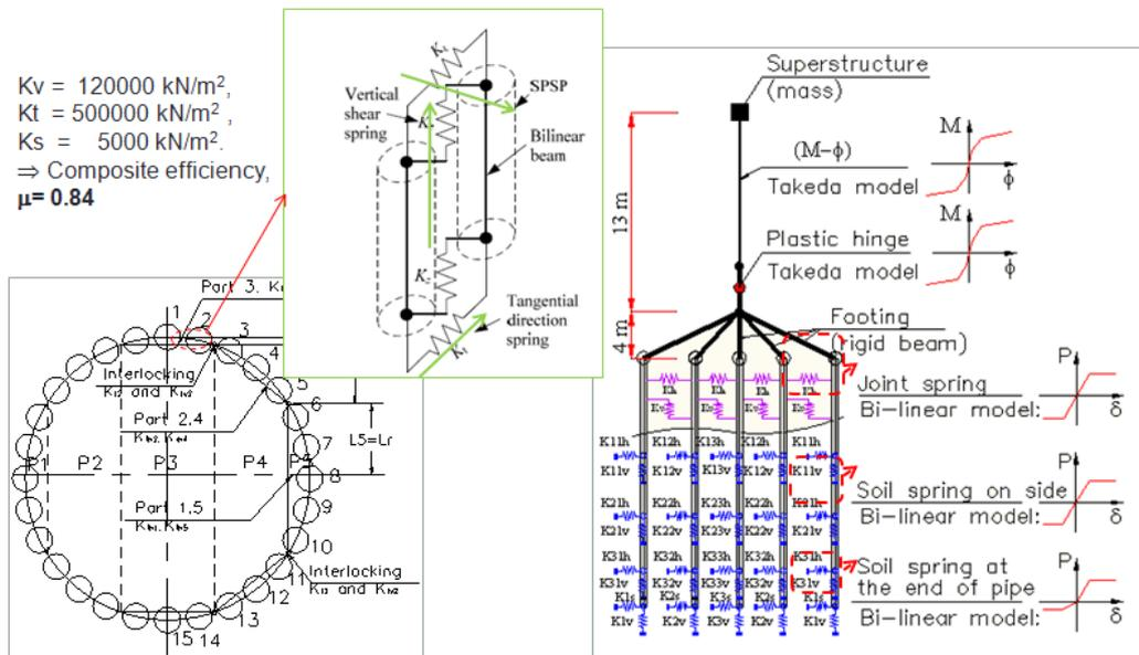
**Fig.2.10** A column model with soil springs (SFSI model)
