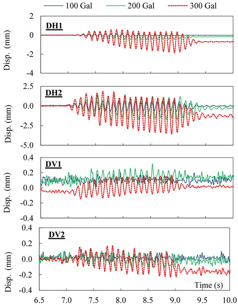
**Fig.3.25** Time histories of displacement of superstructure and pile cap in the flat model
