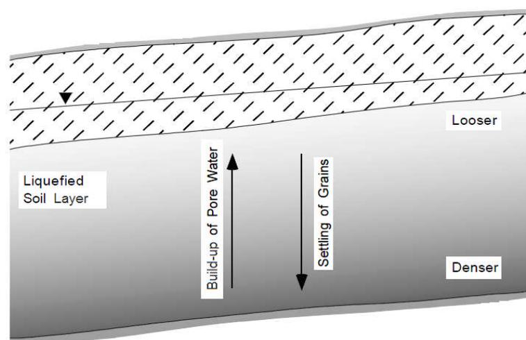
**Fig.2.18** Effect of liquefied thickness on the surface displacement due to the build-up of pore water pressure.
