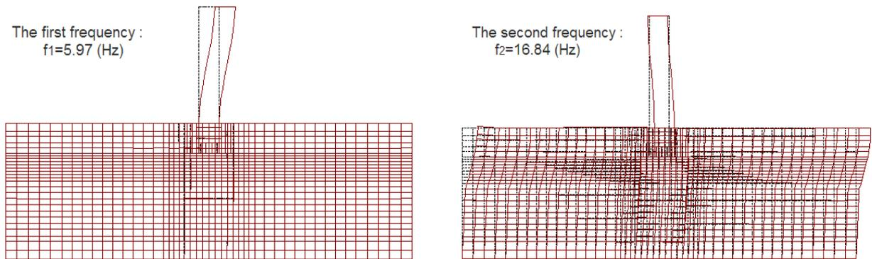
**Fig.4.3** Fundamental natural frequencies of the flat model TSA.
