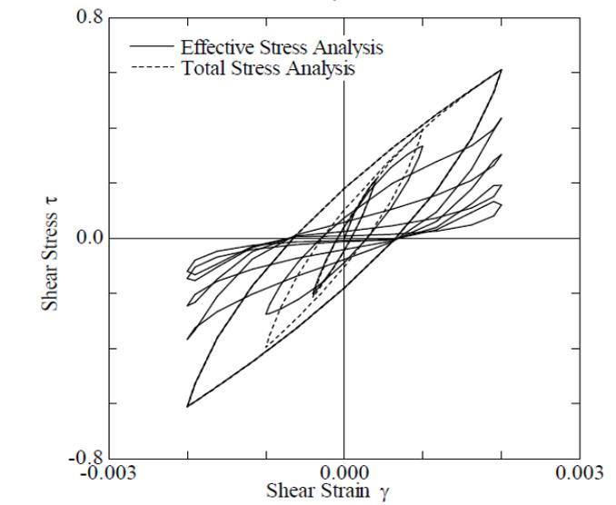
**Fig.2.26** Shear stress and strain relationship of total and effective stress analysis
