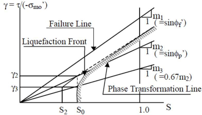
**Fig.5.7** Liquefaction front and relationship between shear stress ratio and shear work.
