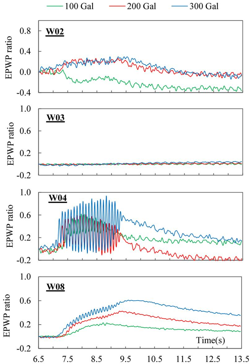
**Fig.3.12** Time histories of pore water pressure in the slope model from 100 to 300 Gal
