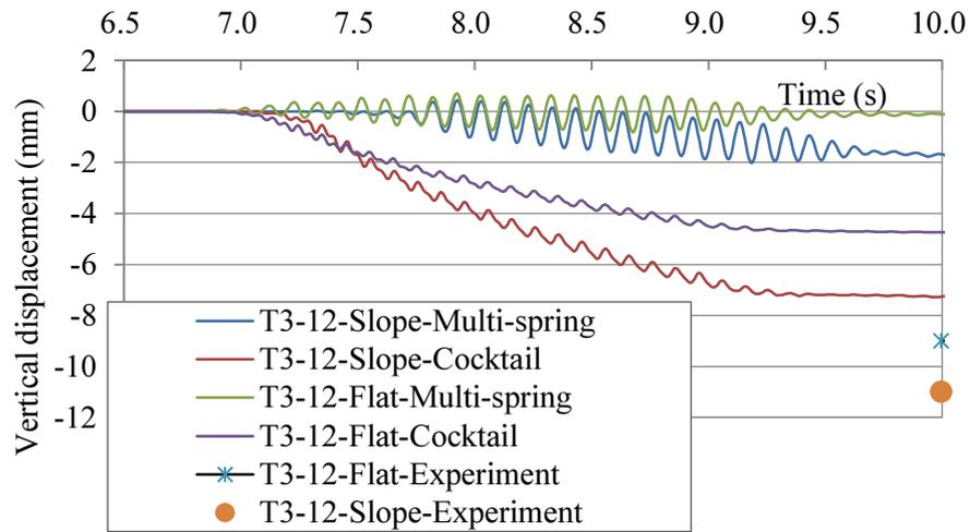
**Fig.5.40** Vertical displacement on ground in the slope and flat models under 300 Gal
