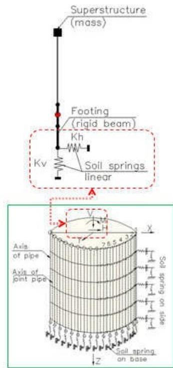
**Fig.2.8** A column model with concentrated spring (SSI model)
