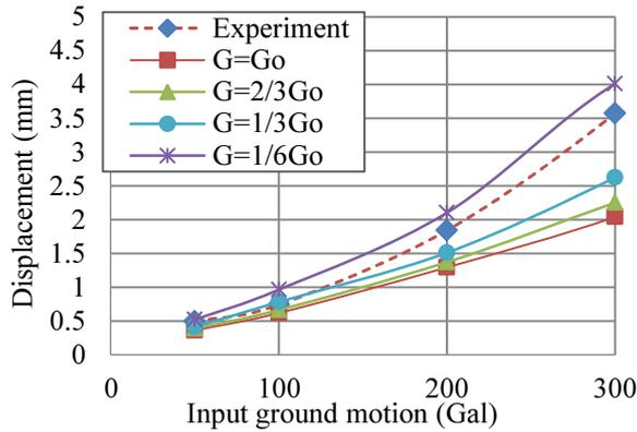
**Fig.4.10** Displacement of superstructure in the flat model.
