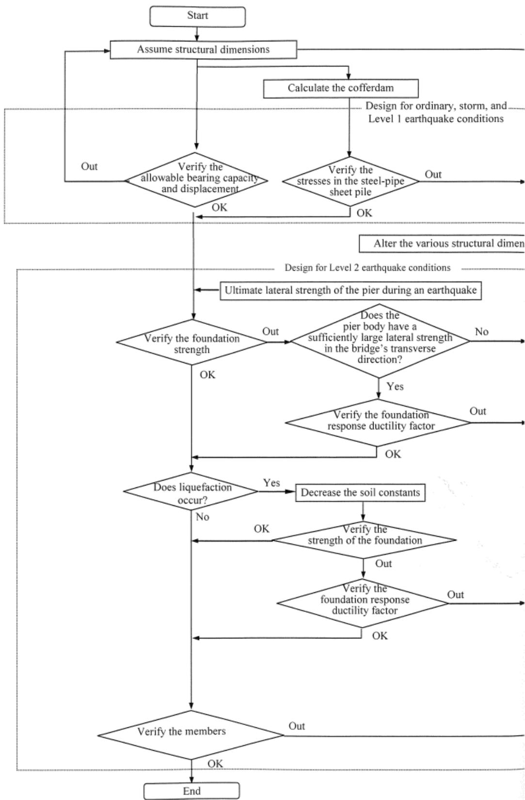
**Fig.2.3** Design and calculation flow of Steel Pipe Sheet Pile Foundation
