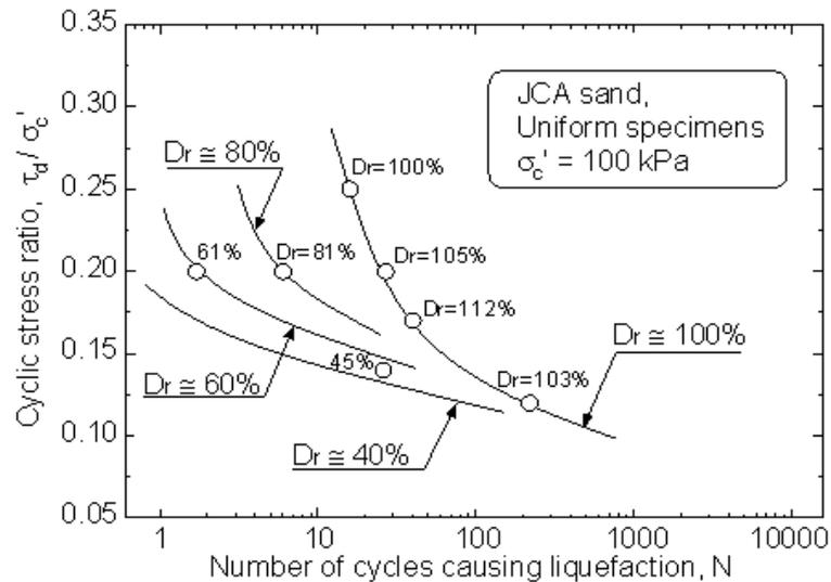
**Fig.2.21** The effect of JCA sand on the liquefaction strength (M. Yoshimine et al. 2005) lateral soil pressure is on the each pile. Cubrinovski and Ishihara et al. (2005) investigated the pile-group effects can be captured by a simple method of analysis using a single pile model.
