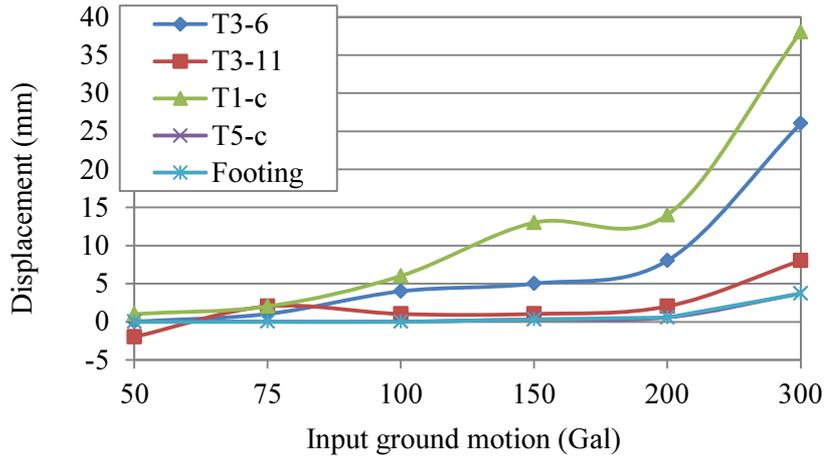
**Fig.3.19** Measured residual displacement at T1-c, T3-6, T3-11, T5-c and the footing in the slope model from 50 to 300 Gal
