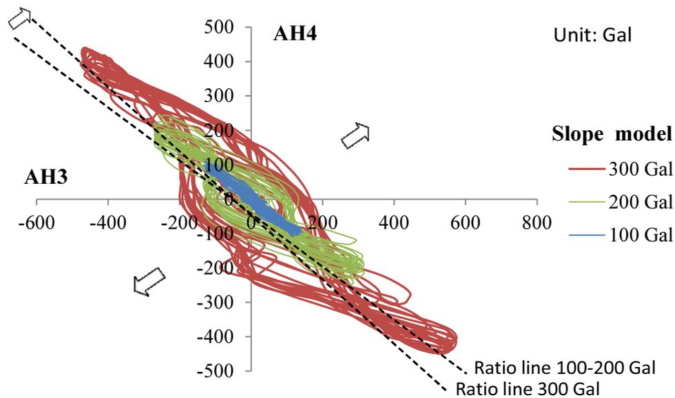
**Fig.3.24** Comparison of acceleration time histories between AH03 of pile cap and AH04 of superstructure in the slope model
