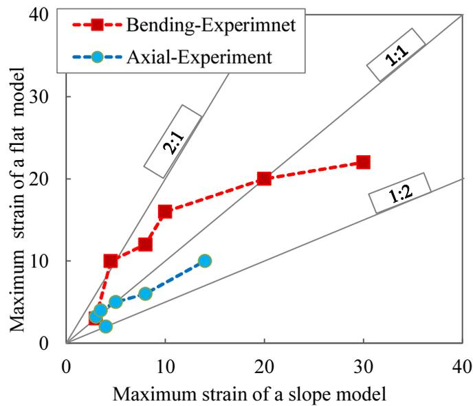
**Fig.3.35** Comparison of bending strain along the front and back sides between the flat and slope models
