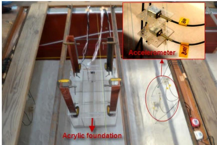
Fig.3.7 Acrylic foundation and accelerometers arrangement in the ground
