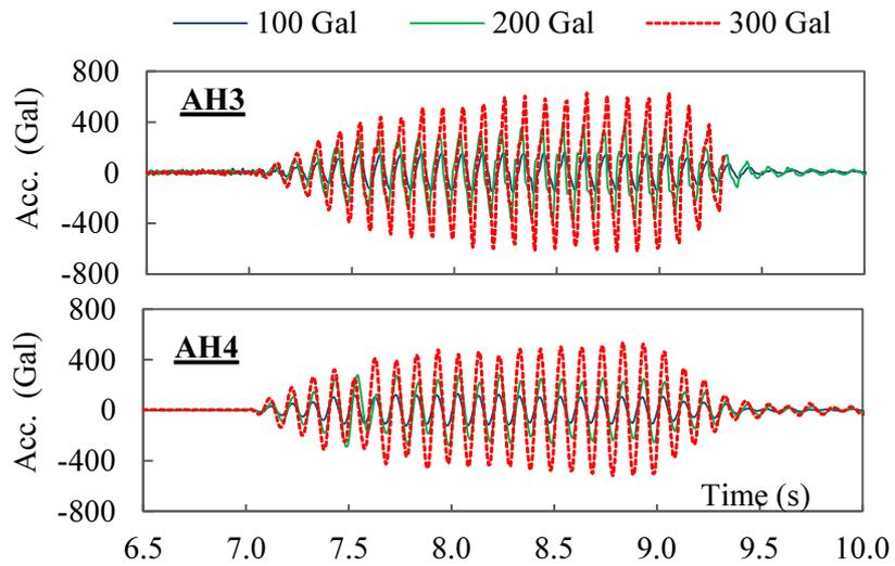
**Fig.3.21** Time histories of acceleration of pile cap and superstructure from 100 to 300 Gal
