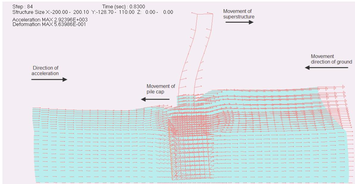
**Fig.4.15** Behavior of ground in the slope model in case 300 Gal input ground motion
