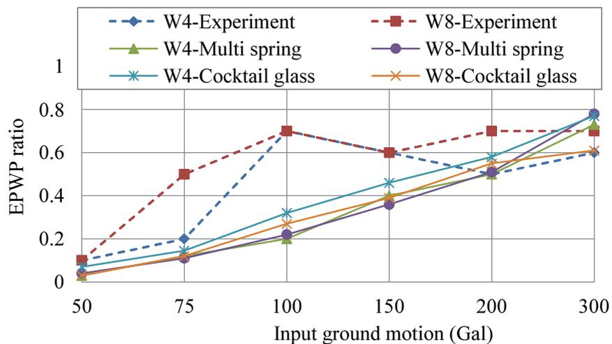
**Fig.5.16** EPWP ratio in the flat models from 50 to 300 Gal
