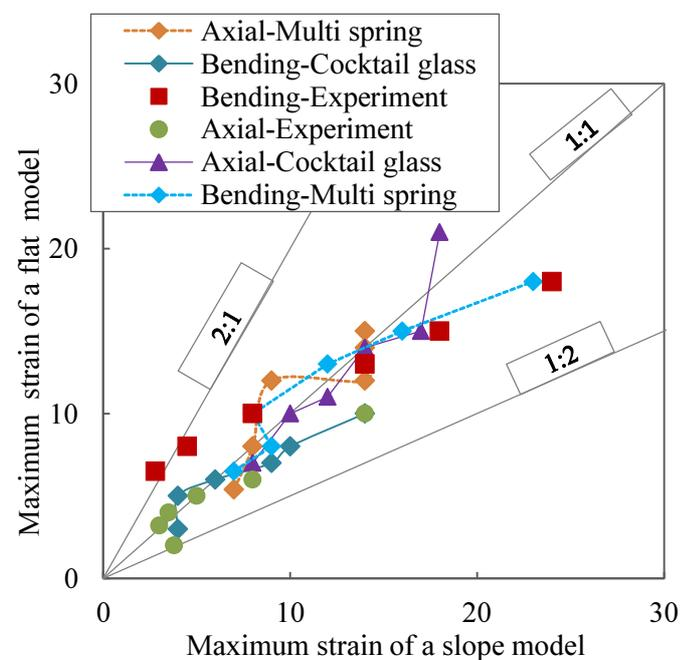
**Fig.5.43** Comparison of maximum strain along the front and back sides between the flat and slope models
