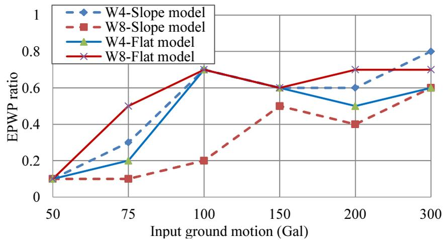
**Fig.3.13** Comparison of EPWP ratio between models from 50 to 300 Gal
