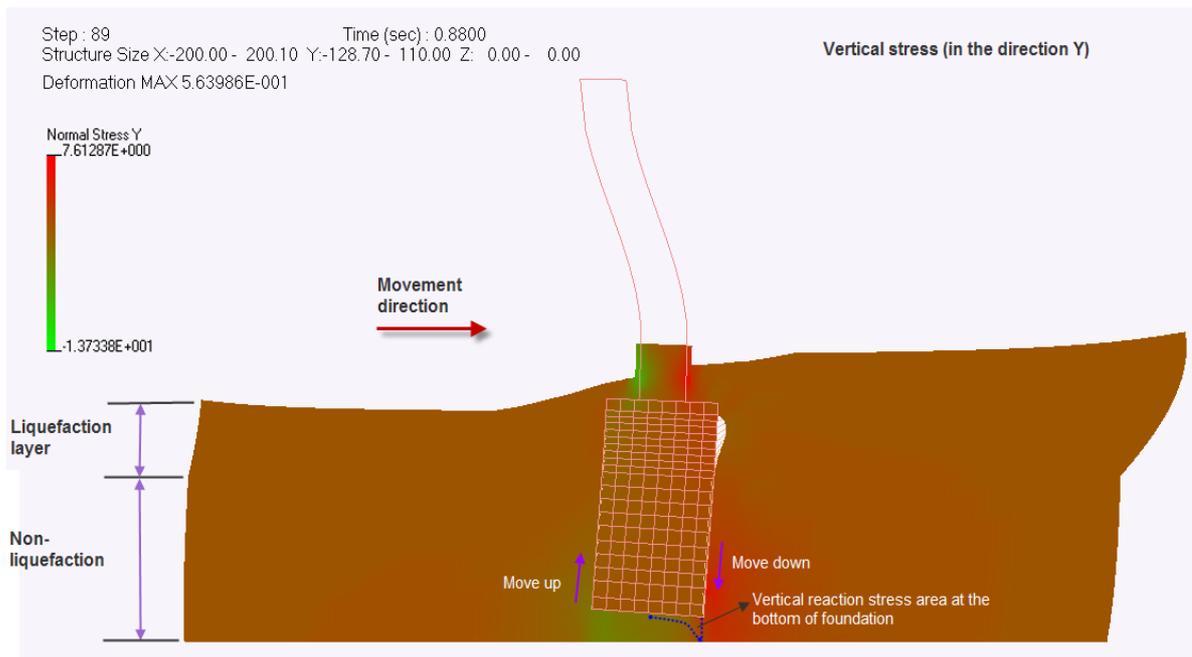
**Fig.4.19** Distribution of vertical reaction stress in the slope model in case of  $1/6G_0$
