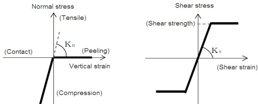
**Fig.5.4** Joint property of interface element between soil and the foundation
