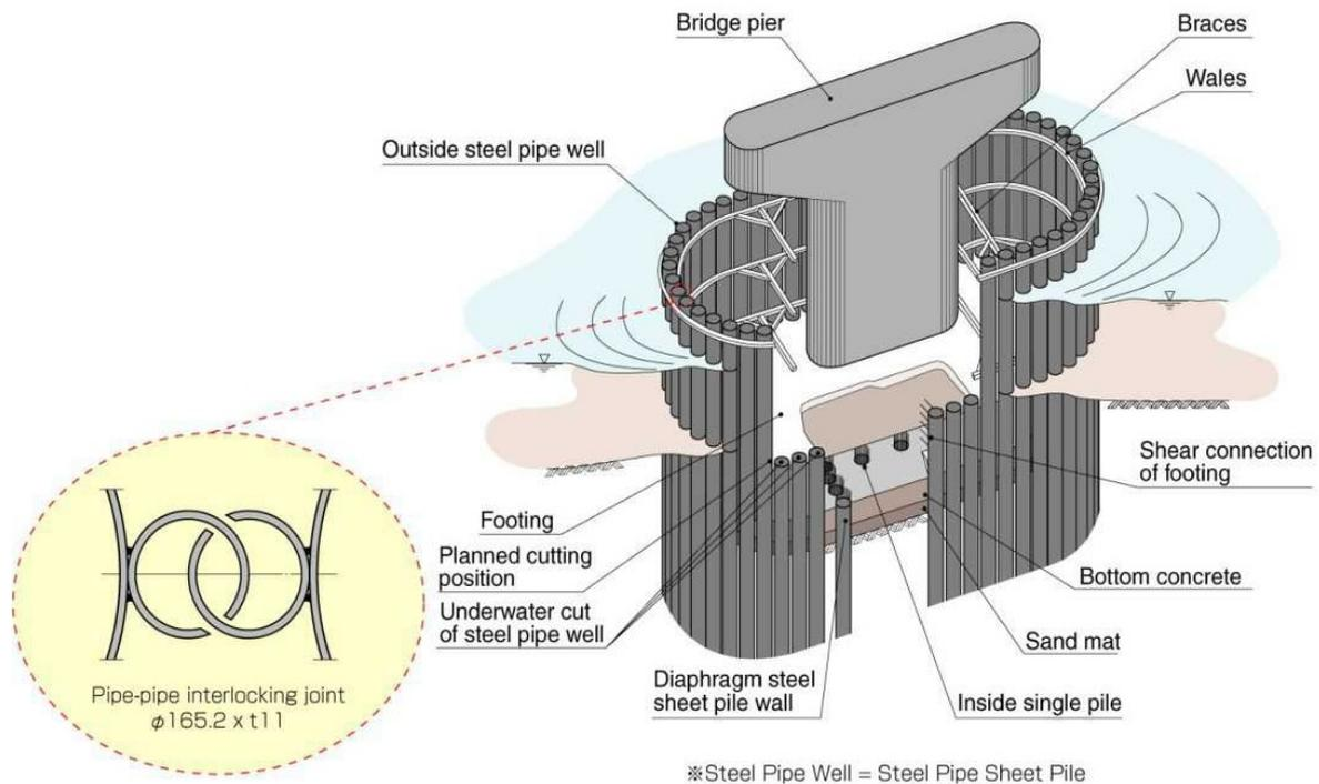
**Fig.2.1** Overview of Steel Pipe Sheet Pile foundation
