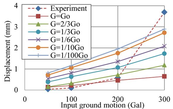
**Fig.4.13** Displacement of pile cap in the slope model.
