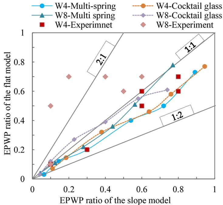
**Fig.5.18** Comparison of EPWP ratio at W4 and W8 between the flat and slope models.
