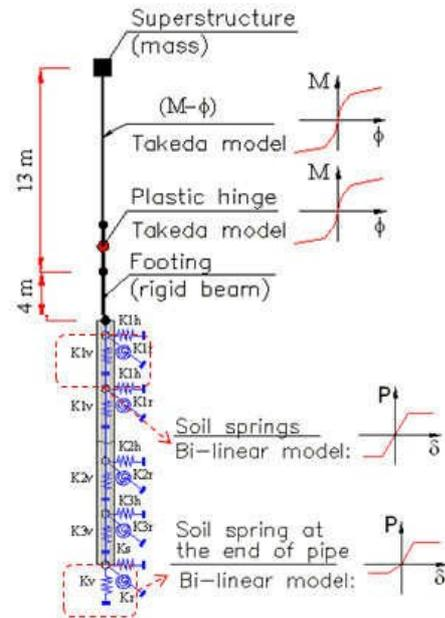
**Fig.2.9** 2D frame model with soil springs (SFSI model)
