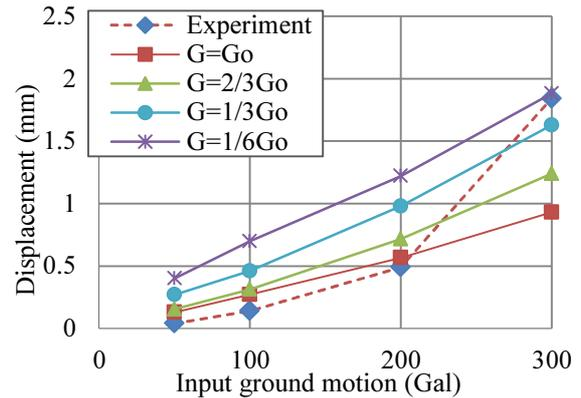
**Fig.4.11** Displacement of pile cap in the flat model.
