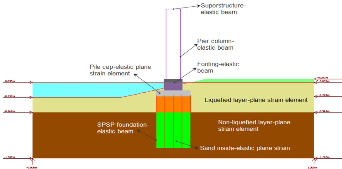
**Fig.5.5** Numerical slope model in Effective Stress Analysis (ESA)
