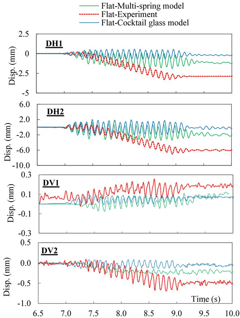
**Fig.5.25** Horizontal and vertical response of superstructure and pile cap in the slope model under 300 Gal
