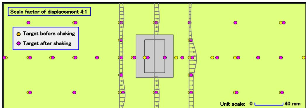
Fig.3.18 The measured displacement distribution of the ground surface movement in the flat model under 300 Gal
