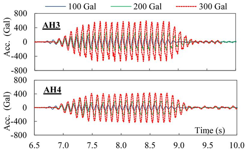
**Fig.3.23** Time histories of acceleration between AH03 and AH04 in the slope model
