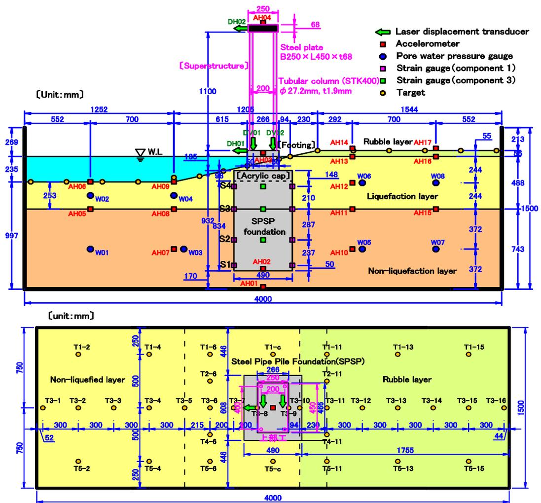
Fig.3.9 General view of the slope model and transducers arrangement.
