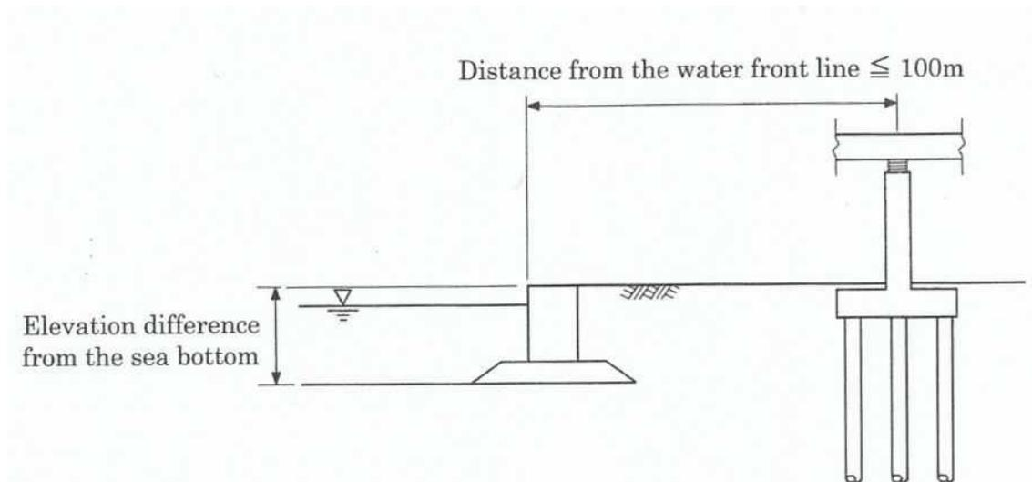
**Fig.1.12** Verification of liquefaction induced lateral spreading in JRA et al. (2002)
