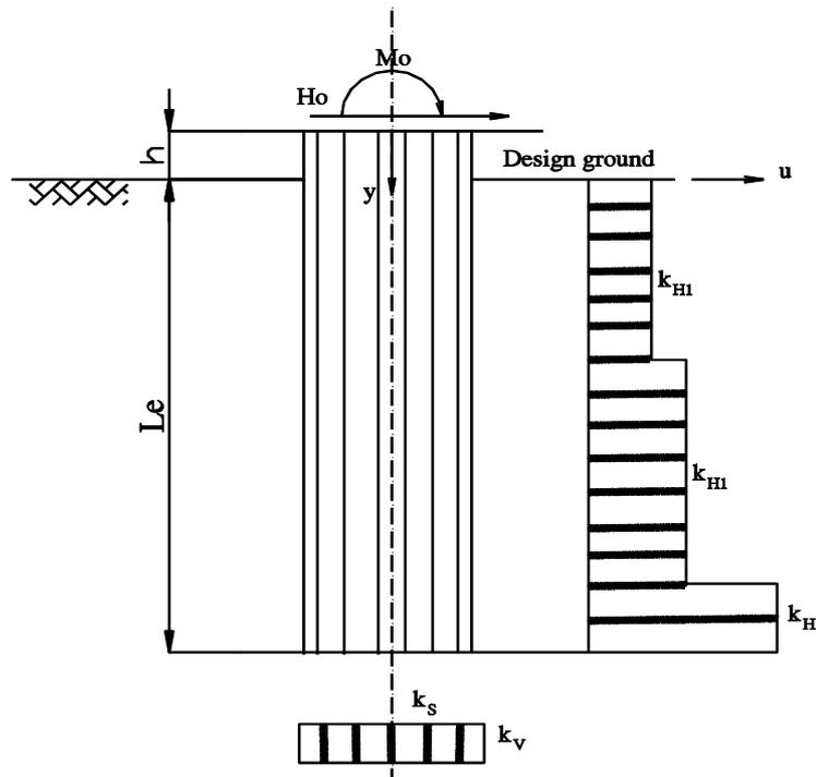
**Fig.2.4** The finite length beam on elastic foundation
