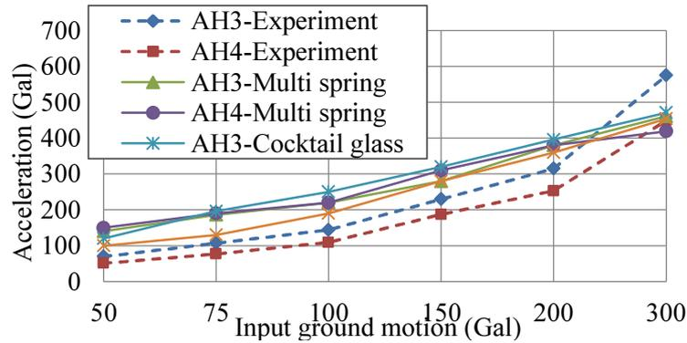
**Fig.5.22** Maximum horizontal acceleration of the superstructure at AH4 and pile cap at AH3 in the slope model from 50 to 300 Gal
