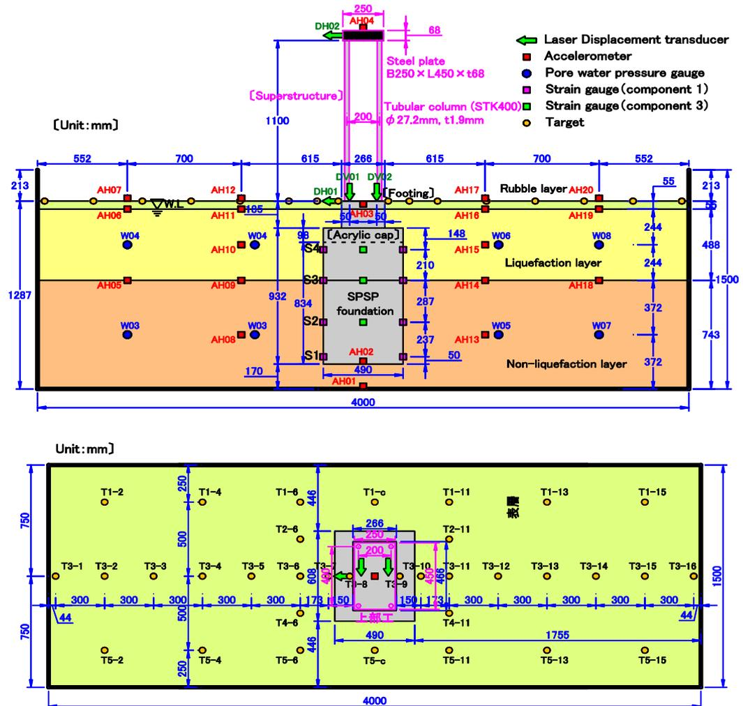
Fig.3.8 General view of the flat model and transducers arrangement.
