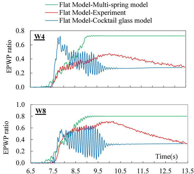
**Fig.5.12** Time history of EPWP ratio at W4 and W8 in the flat model under 300 Gal.
