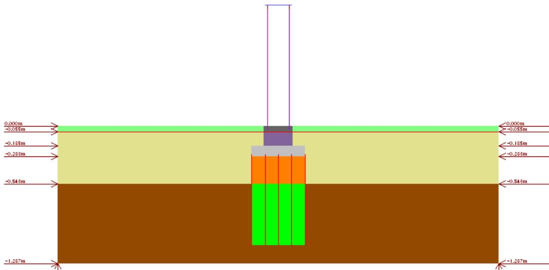
**Fig.5.6** Numerical flat model in Effective Stress Analysis (ESA)
