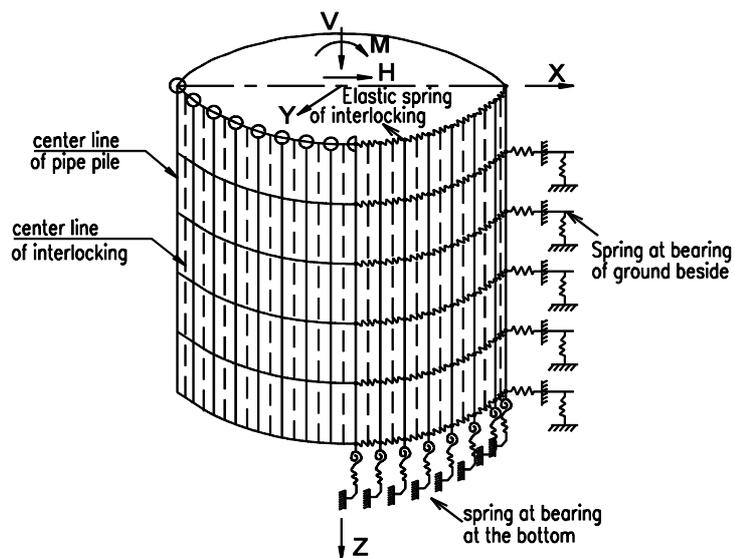
**Fig.2.6** Three dimension model of cofferdam foundation
