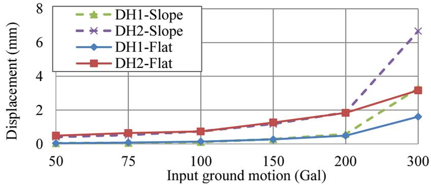
**Fig.3.29** Comparison of displacement at DH1 and DH2 between the flat and slope models
