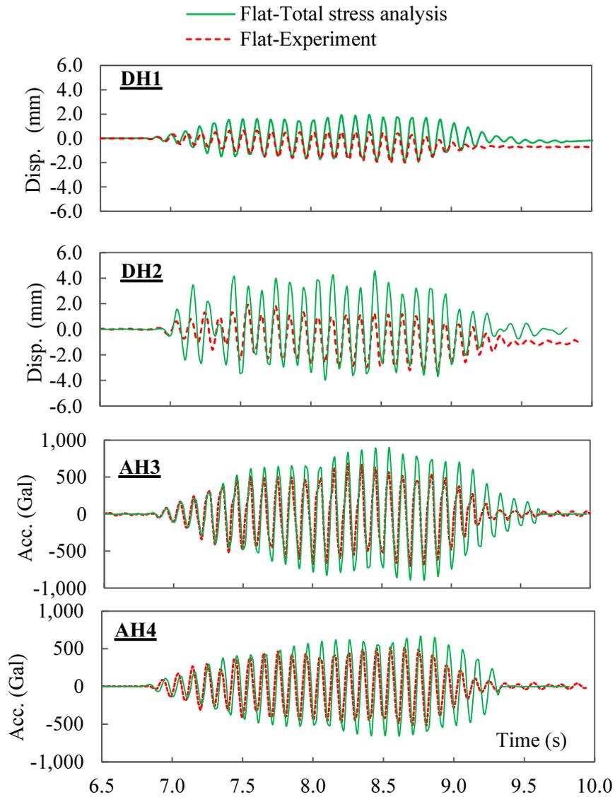
**Fig.4.6** Horizontal displacement and acceleration time histories of 300 Gal of superstructure in case of  $1/6G_0$  in the flat model
