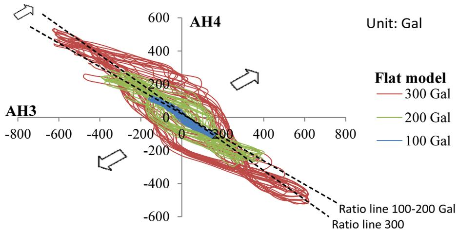
**Fig.3.22** Comparison of acceleration time histories between AH03 of pile cap and AH04 of superstructure in the flat model
