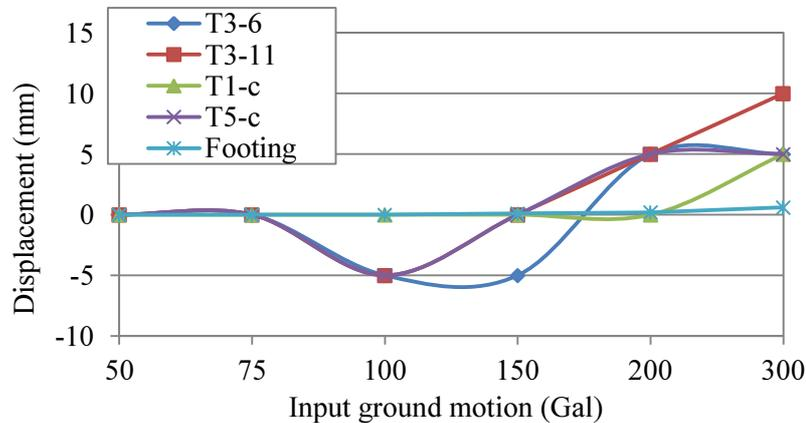
**Fig.3.20** Measured residual displacement at T1-c, T3-6, T3-11, T5-c and the footing in the flat model from 50 to 300 Gal.
