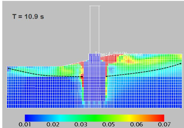
**Fig.5.38** Maximum shear strain distribution in the slope model under 300 Gal.
