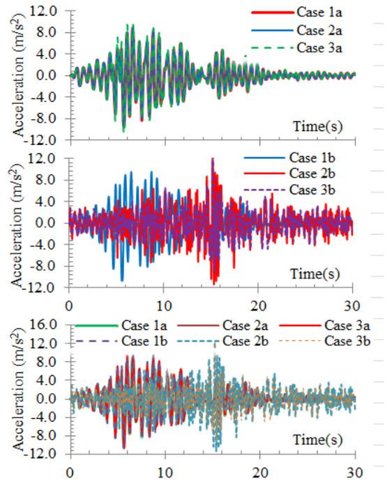
**Fig.2.14** Acceleration response at top of pier
