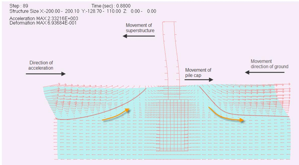
**Fig.4.14** Behavior of ground in the flat model in case 300 Gal input ground motion
