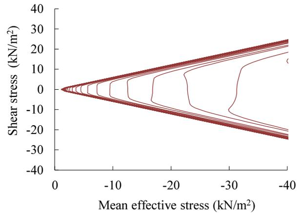
**Fig.5.11** Effective stress paths from liquefaction parameters
