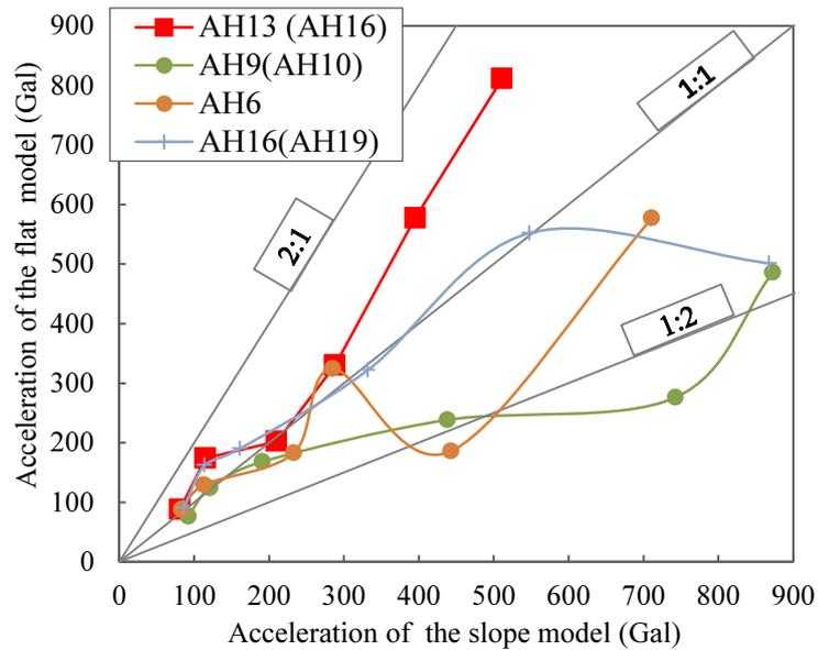
**Fig.3.16** Comparison of acceleration between two models from 100 to 300 Gal
