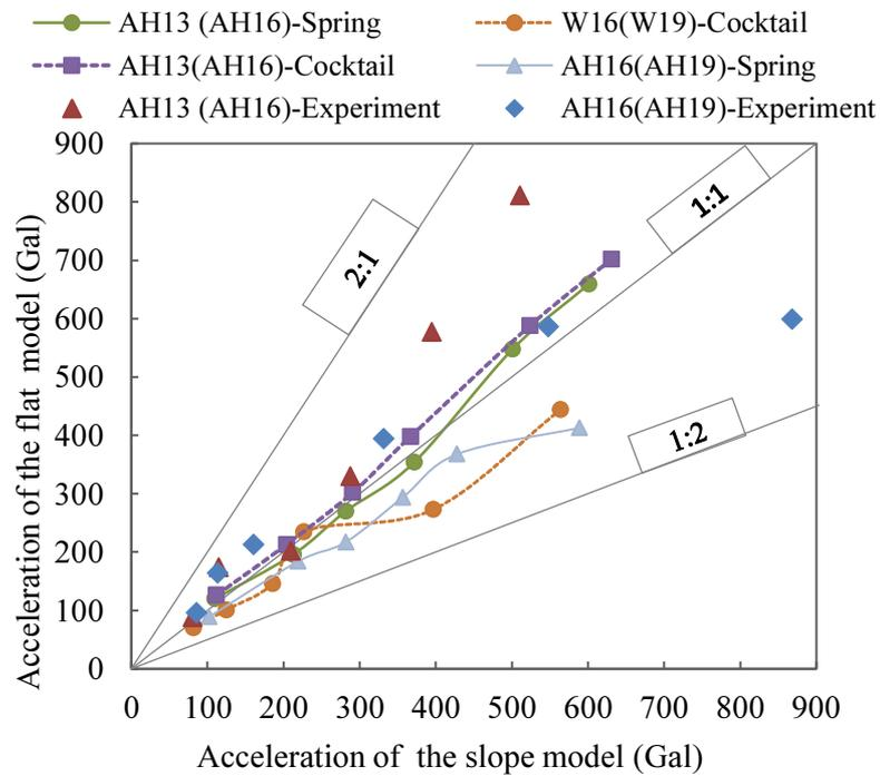
**Fig.5.36** Comparison of acceleration at AH13, 16 in the flat model and AH16, 19 in the slope model.
