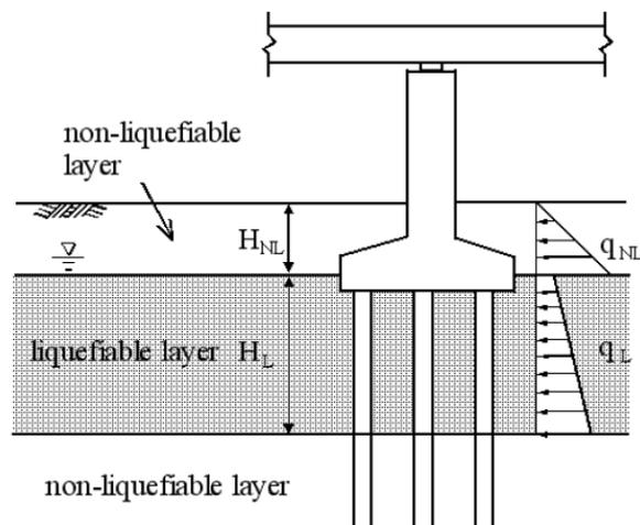
**Fig.1.13** Lateral spreading pressure in JRA 2002
