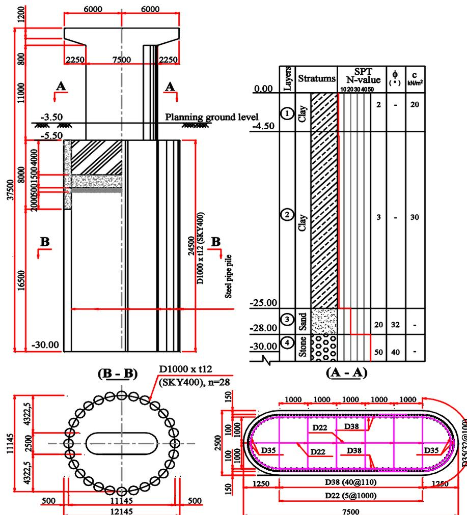
**Fig.2.7** Prototype bridge pier with Steel Pipe Sheet Pile, foundation and soil properties
