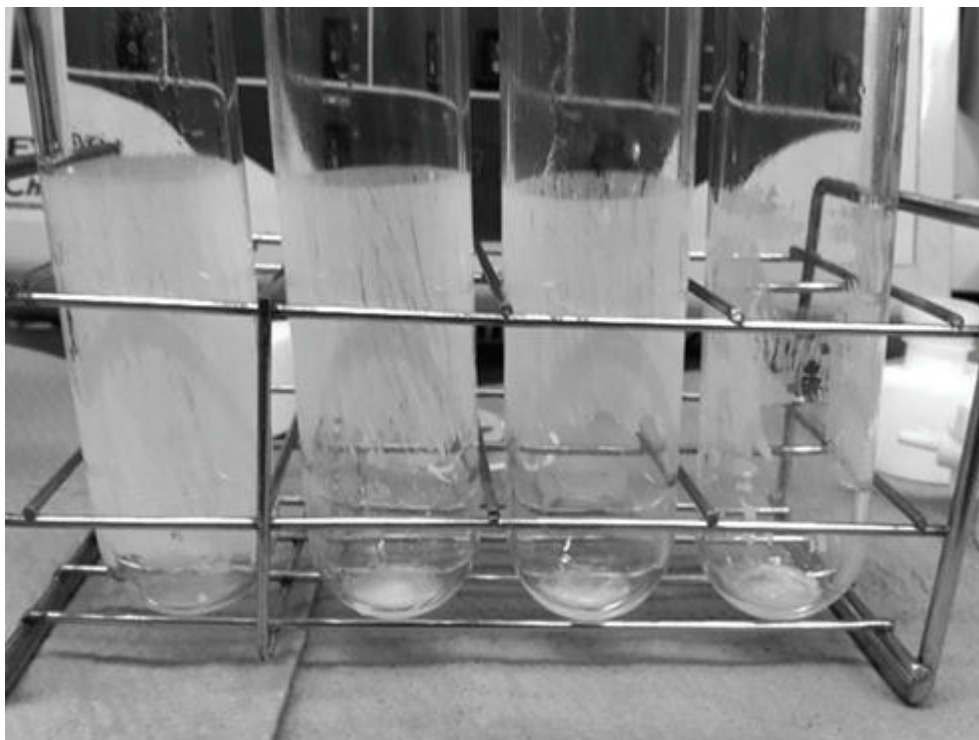
Figure 5.2 Observed white sticking on the crystallizers
