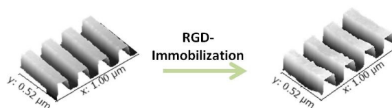
Figure 3-2: 3D AFM images of nanopattern before and after the immobilization of RGD with the fidelity of structures.
