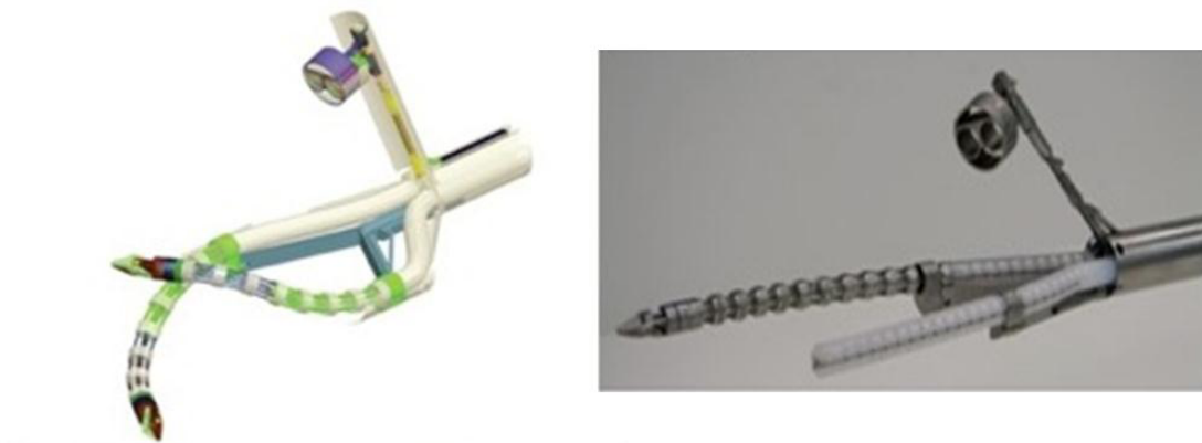
Figure 1. 6 Insettable robotic effector platform for single access surgery [32].
