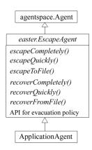
Figure 5. Class hierarchy of application in the EASTER.
