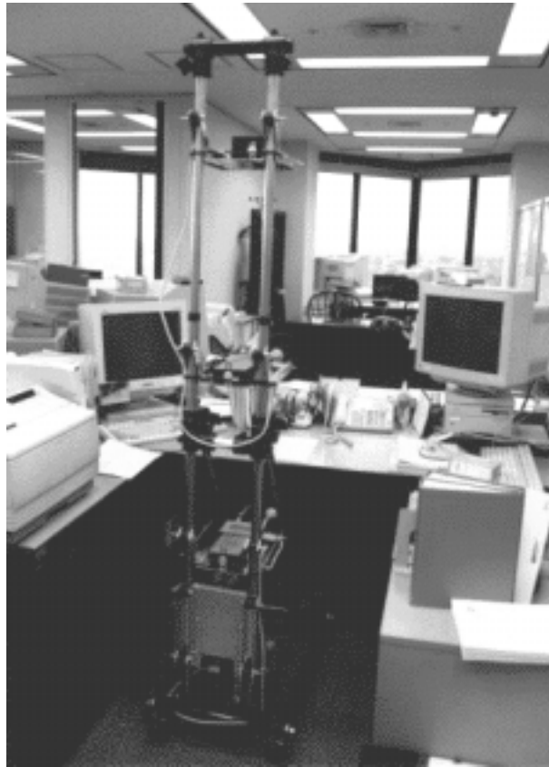
Figure 4-2. Measurement of workstation with mobile measurement cart
