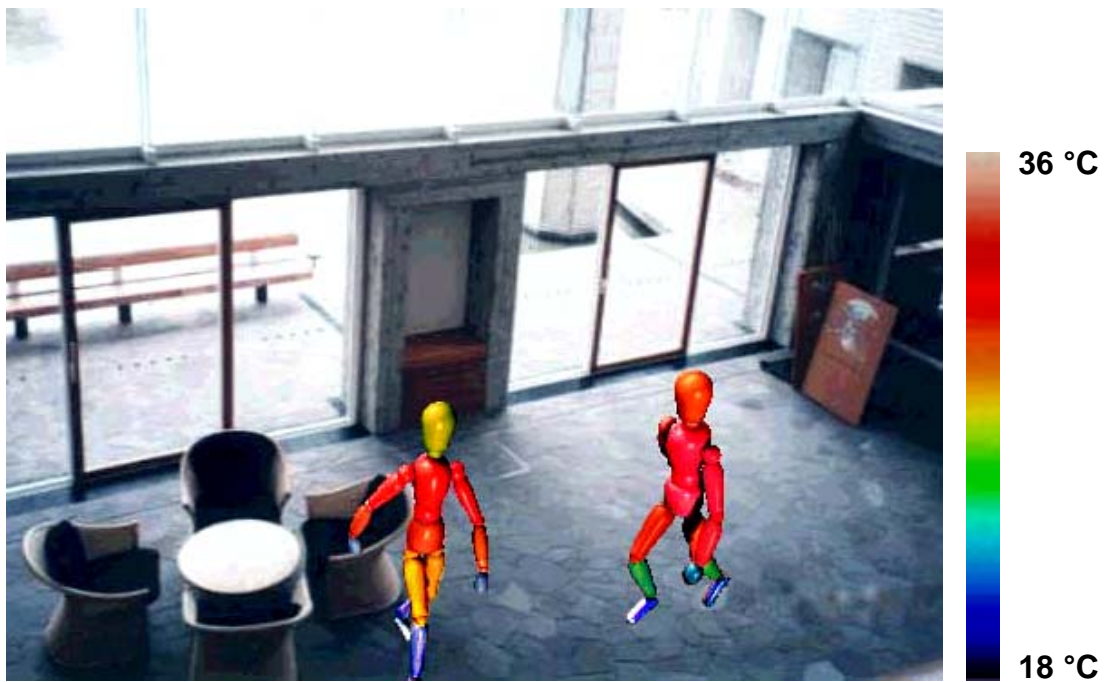
Figure 2-12. Skin temperature difference in Case 2. Short route passé-by on left and long route on right
