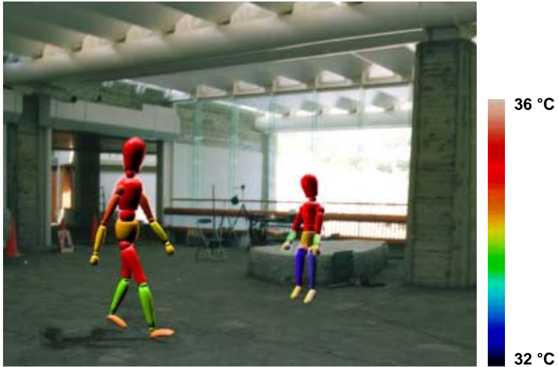
Figure 2-11. Skin temperature difference in Case 1. Passer-by (left) and occupant (right) in the 2F lobby.
