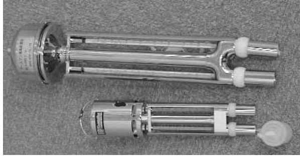
Figure 6-1. Mini-Assmann and normal size Assmann psychrometer
