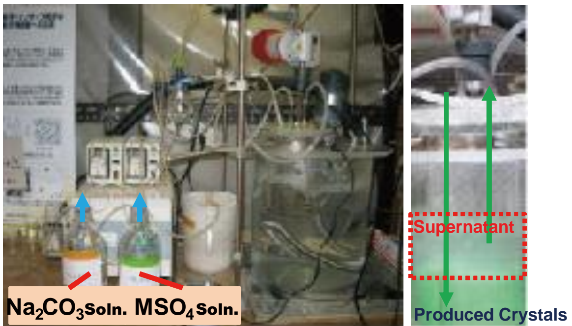
Fig. 3-1 The semi-batch crystallizer and the tank interior agitation.
