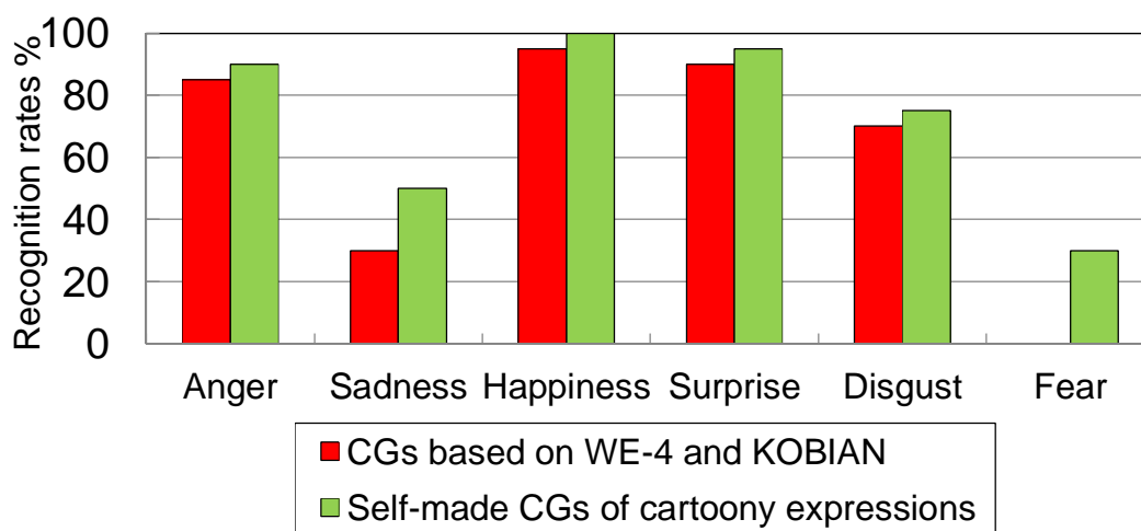
Fig. 2. 37 Recognition rates of the CGs based on WE-4 and KOBIAN, and the self-made CGs of cartoony expressions
