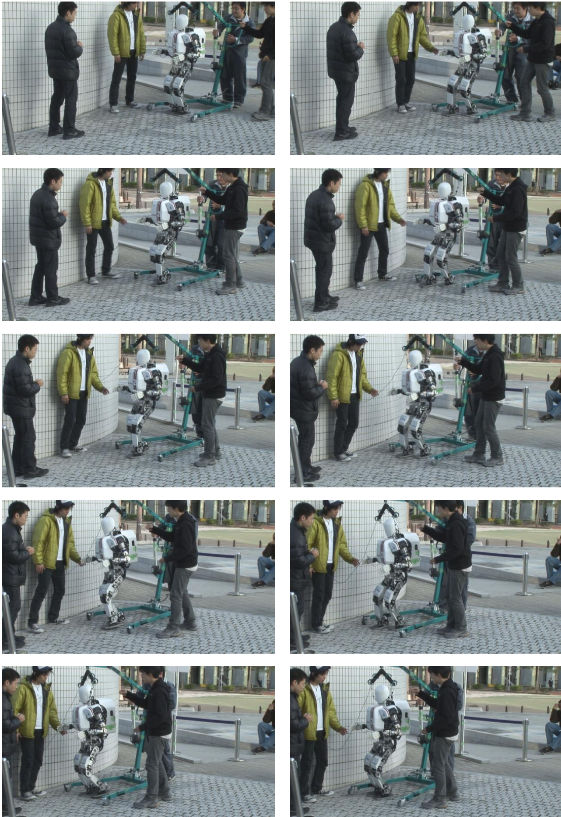
Figure 4.23 ⑦ Walking experiment on uneven and slope 5[deg] ground.
