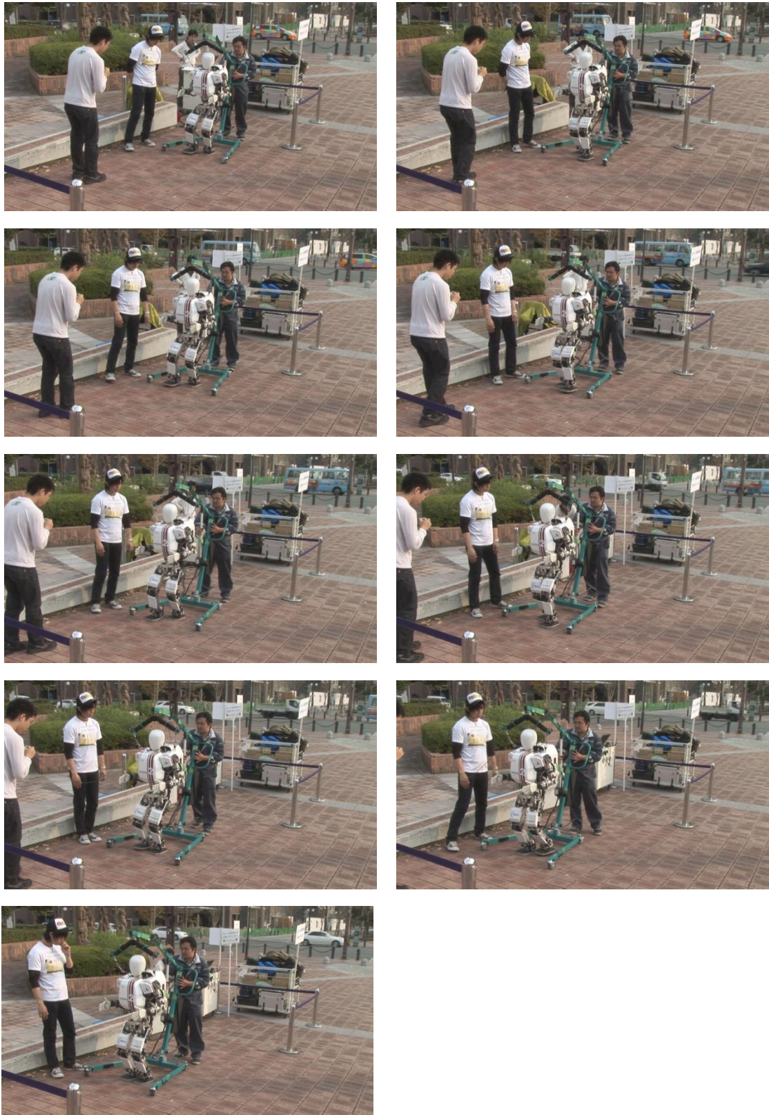
Figure 4.19 ⑤Walking experiment on flat → slope of 5[deg].
