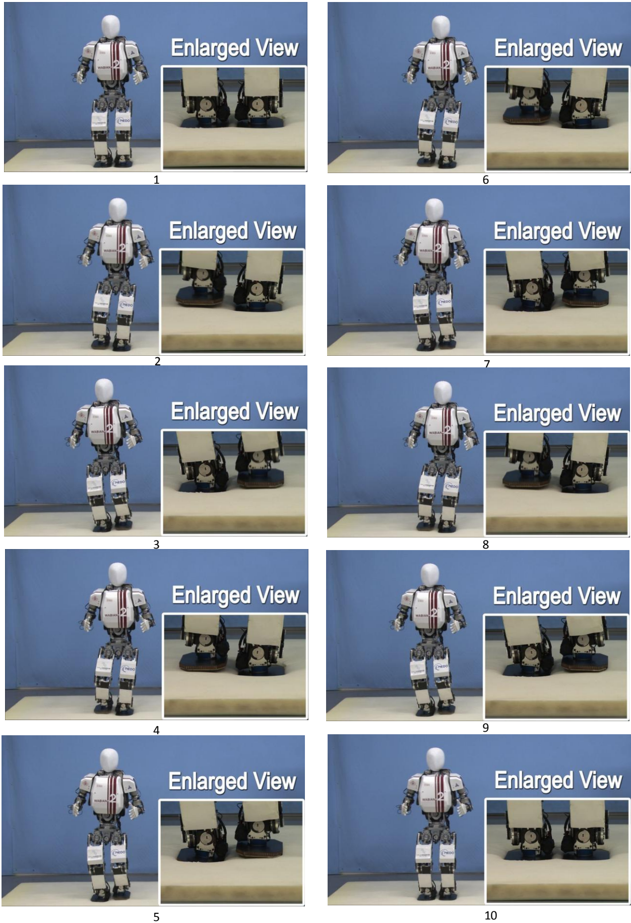
Figure 7.28 Walking experiment on a soft ground with a density of 22 \pm 2 \text{ kg/m}^3
