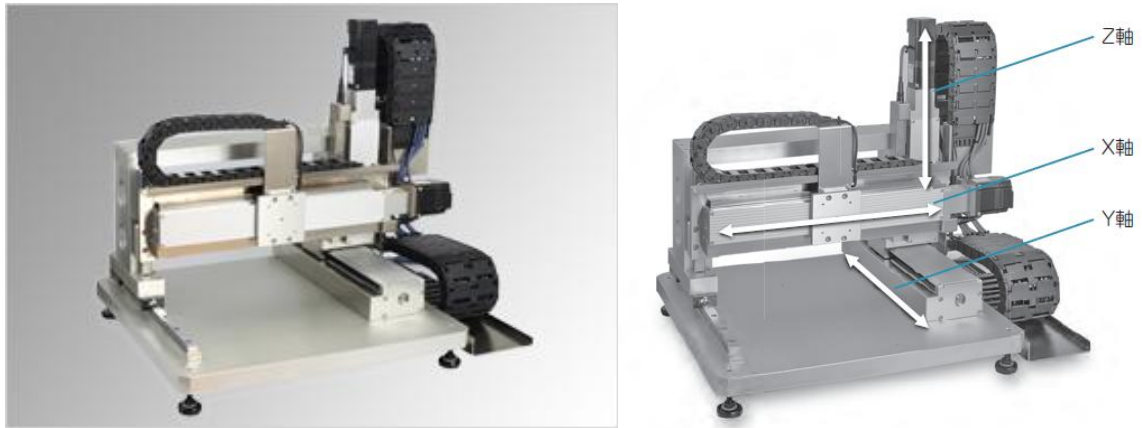
Figure 3.2 Gantry robot (GR-1750 series [Hirata corporation]).
