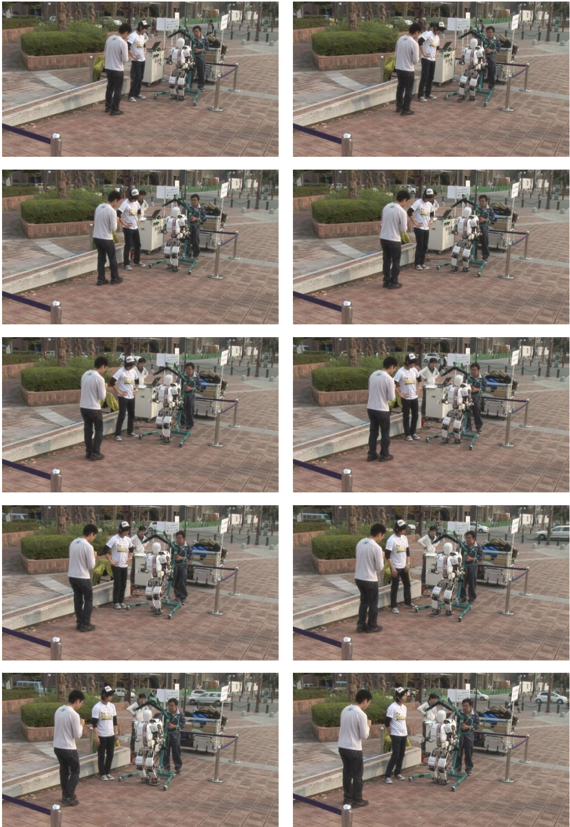
Figure 4.17 ⑤Walking experiment on flat → slope of 5[deg].
