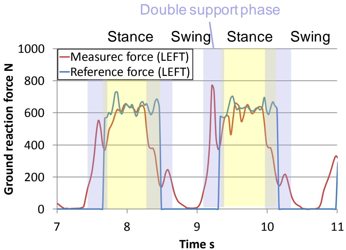
Figure 7.32 Grand reaction force without walking stabilization control
