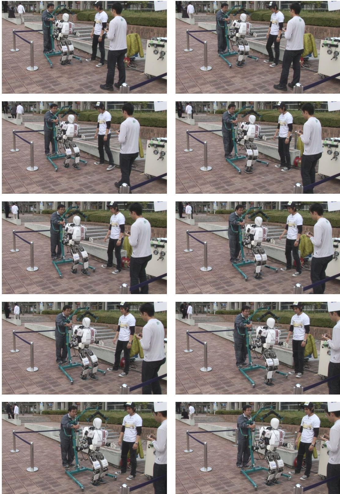
Figure 4.15 ④ Walking experiment on slope of 5[deg] →flat.
