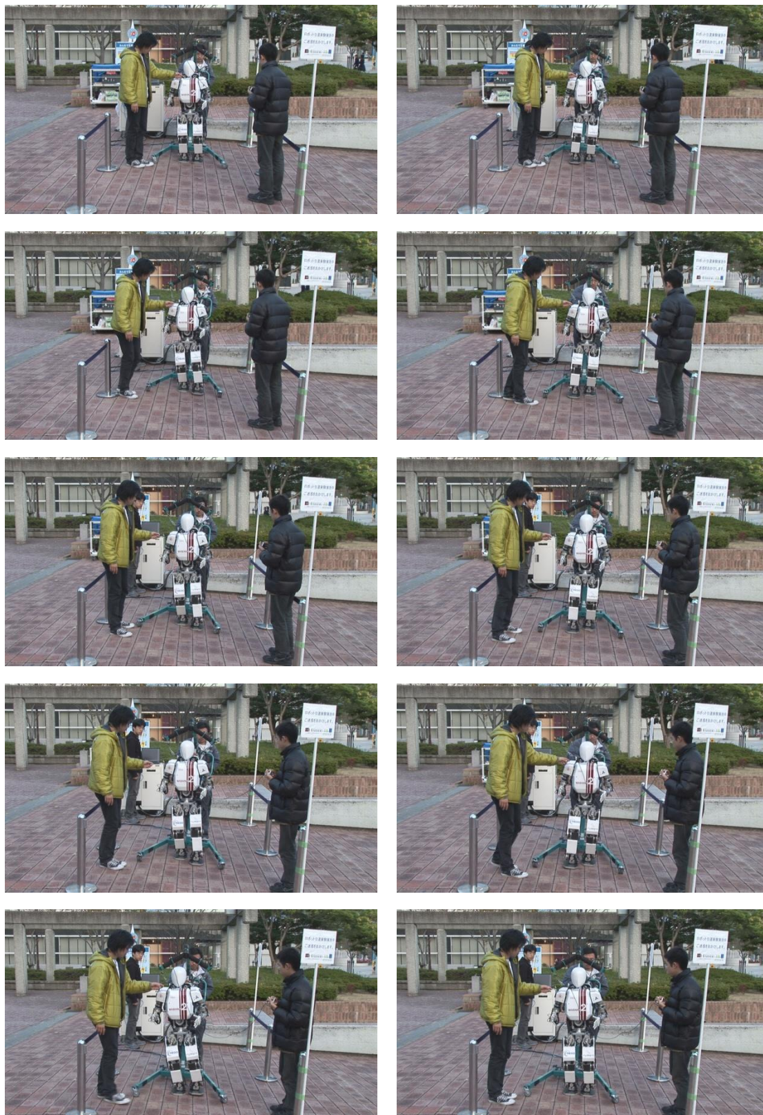
Figure 4.11 ②Walking experiment on slope of 3[deg].
