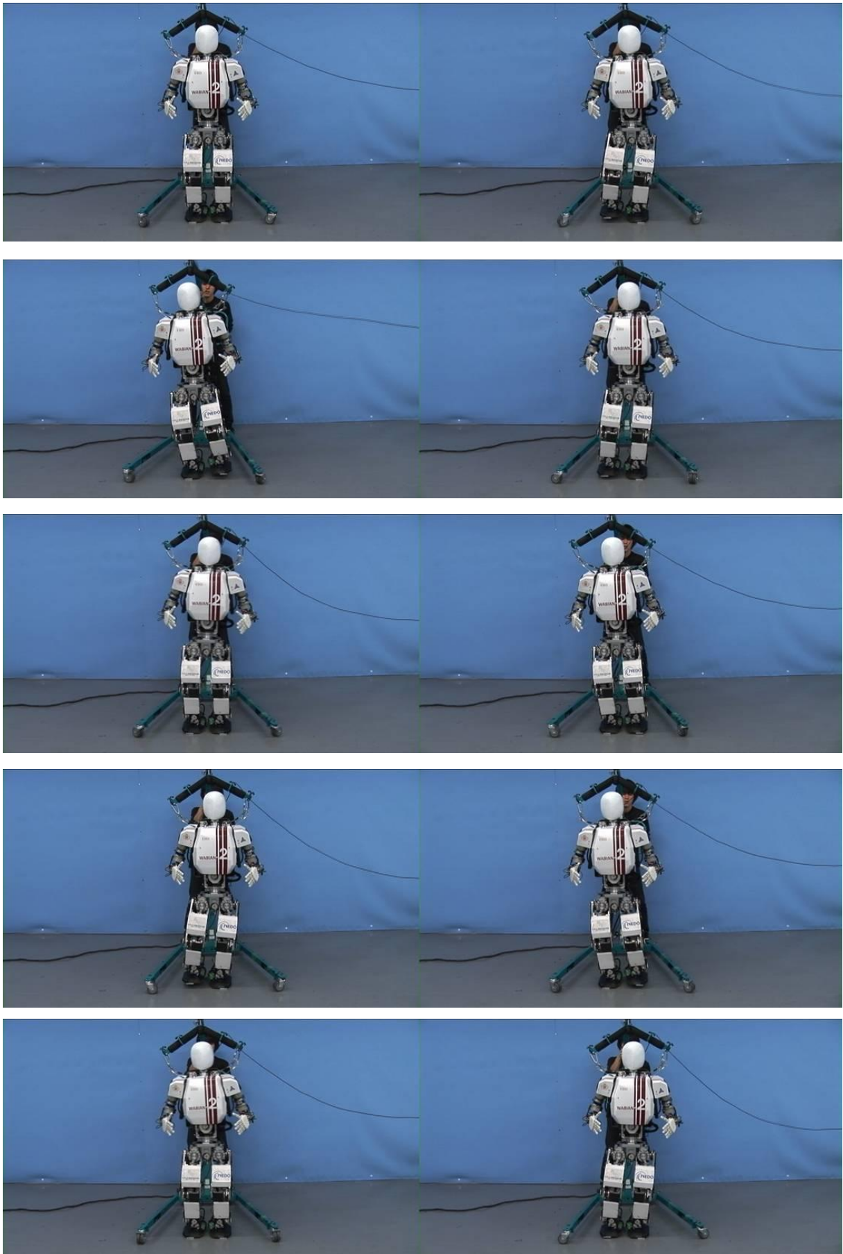
Figure B.10 Walking experiment with narrow foot (width of 30mm)
