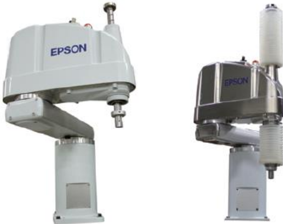
Figure 3.3 Scalar robot G-series [Seiko Epson corporation].
