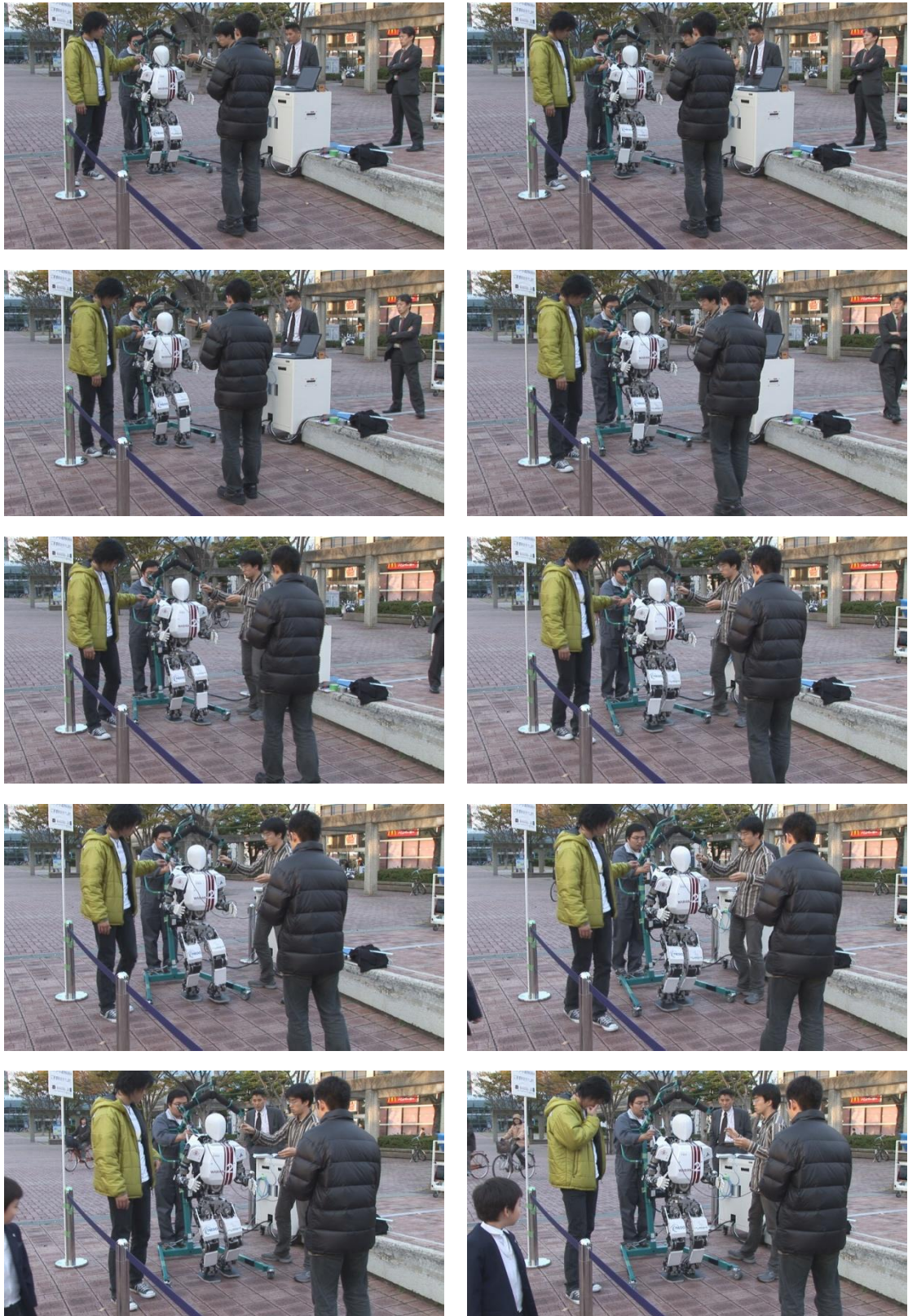
Figure 4.13 ③Walking experiment on flat →slope of 3[deg].
