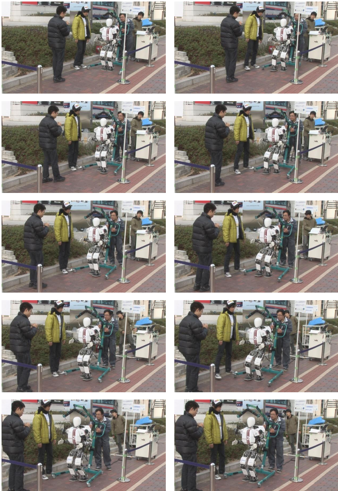
Figure 4.27 ⑨Walking experiment on flat ground.
