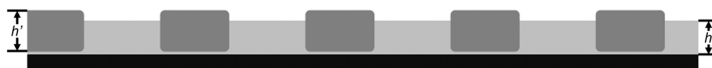
Figure 2-8. Illustration of cross section of an as-cast ultrathin polymer blend film (PS: dark gray; PMMA: light gray).
