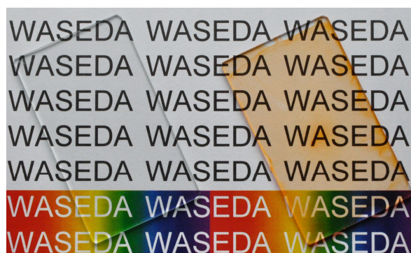
Figure 11. Photograph of the spin-coated film on a glass substrate (left) and the film after adsorption of Orange II (right). The sizes of the substrates are 28 mm \times 48 mm.
