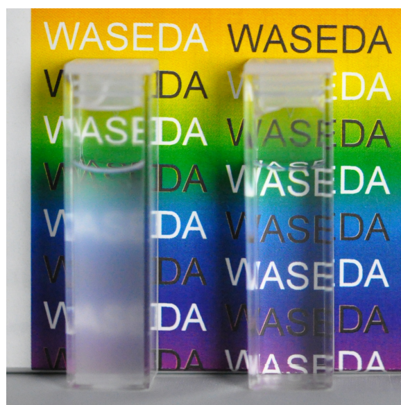
Figure 2. Photograph of the aqueous suspensions of Bim-Oct before (left) and after (right) ultrasonication.
