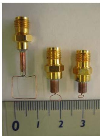
Fig.1.11 Magnetic field probes: MP3, MP2 and MP1
