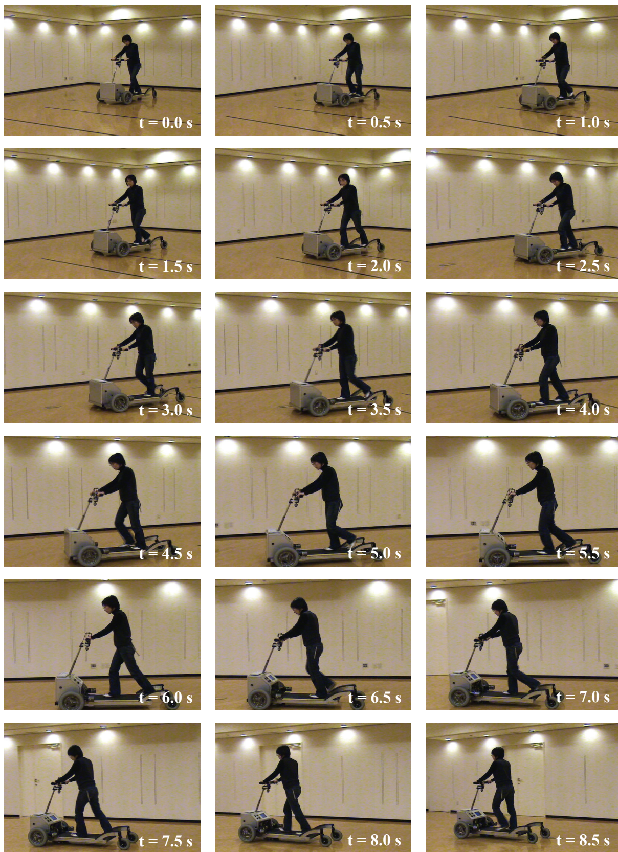
Fig. 5.8 The vehicle moves to the velocity where it walks by twice the velocity(forward)
