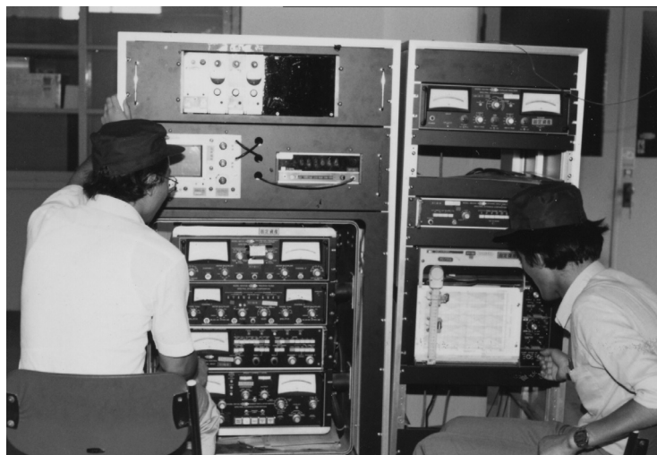
Figure A2.1 An analog frequency response function analyzer designed and offered by Spectral Dynamics, Inc. in 1961
