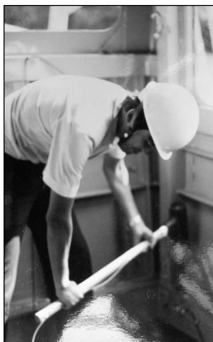
(b) Frequency response function estimation on an electric locomotive
