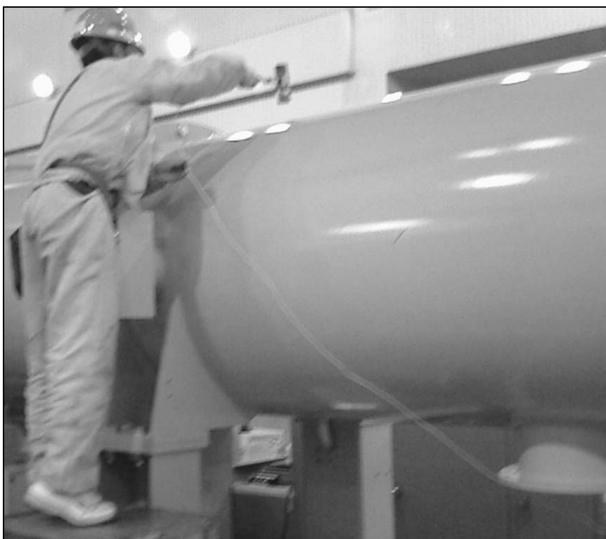
Modal testing on a gas insulated switch gear tank
