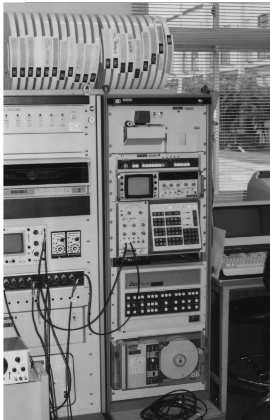
Figure A2.2 A digital frequency response function analyzer, Type 5451 by Hewlett-Packard Company in 1972
