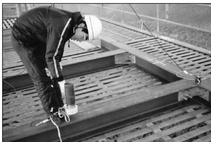
(b) Frequency response function estimation on antenna base
