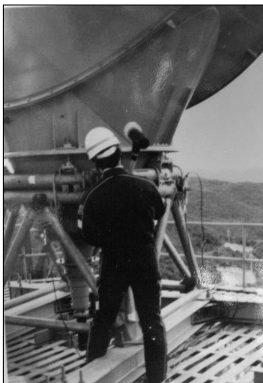
(a) Modal testing on an antenna set up at a steel tower
