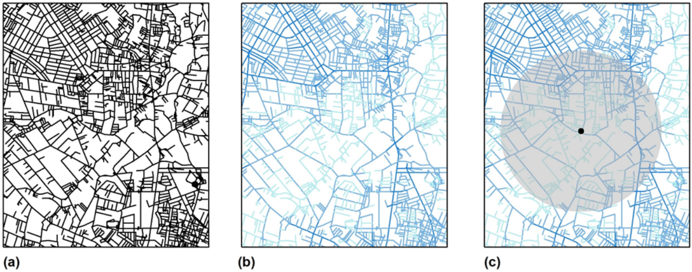
Figure 3. Process of calculating space syntax measures: (a) street centerlines (base map); (b) space syntax measure of integration calculated for each street segment (darker lines are more integrated), (c) area-level measures calculated by aggregating integration values within a buffer area from participant's home.
