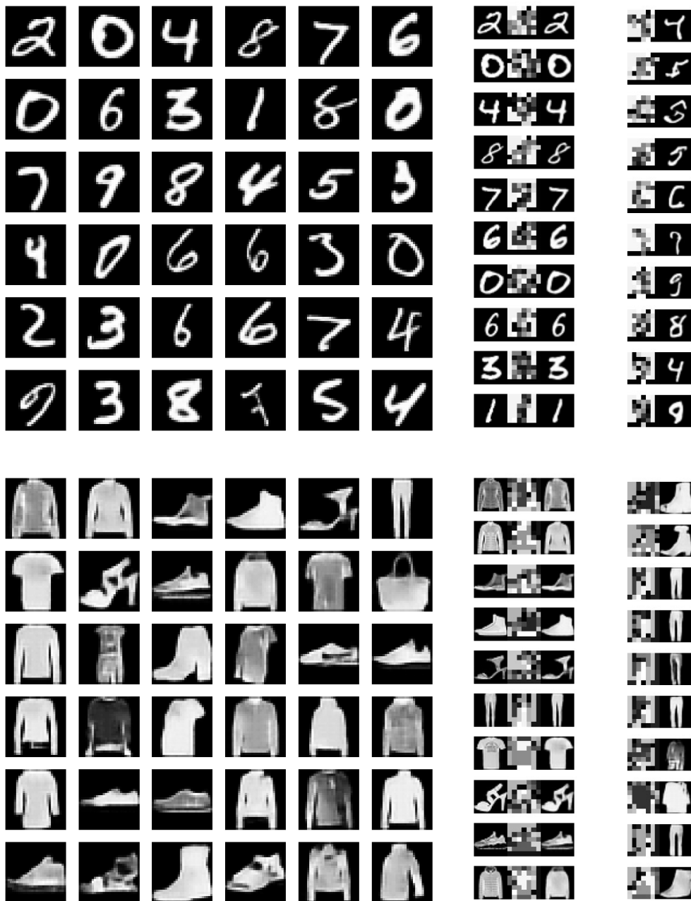
Figure 4.7. Rendering latent space for the implementation of the VQ-VAE model with the DP in the VTF for grayscale datasets like the MNIST of the upper part and Fashion-MNIST of the lower part in both reconstruction and sampling. The left column is the input, and the middle column is a combination of input, latent space, and reconstructed images. The right column is the combination of latent space and sampled images.
