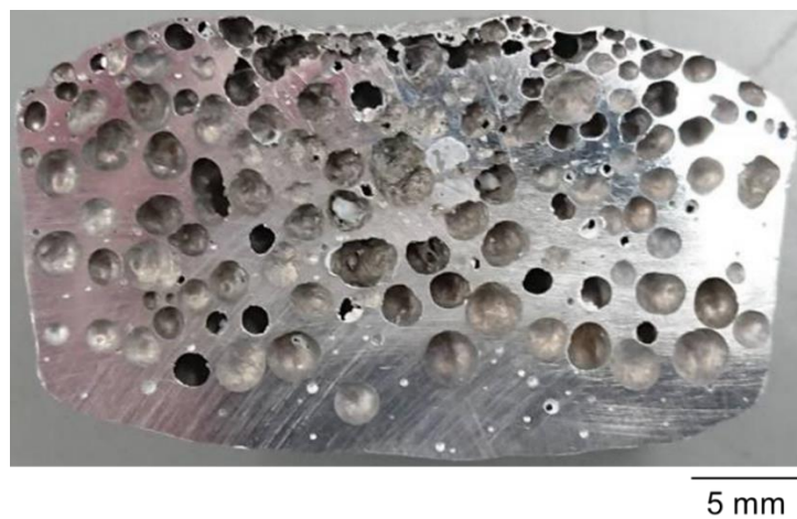
Figure 2-9 Cross section of fabricated aluminum alloy foam through the semi-solid route.
