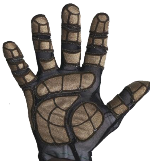
Fig 2.4 Multi modal tactile sensing glove
