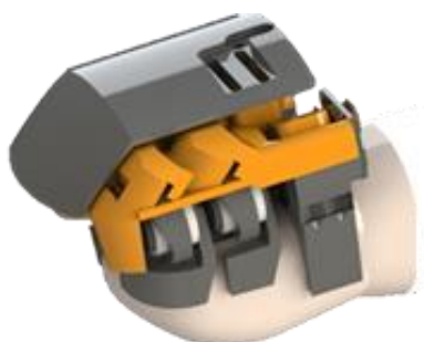
Fig 2.7 Wearable tactile sensor for human fingertips (Sugano Lab research)
