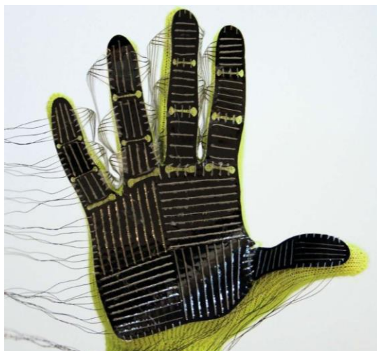
Fig 2.5 Scalable Tactile Glove (STAG)
