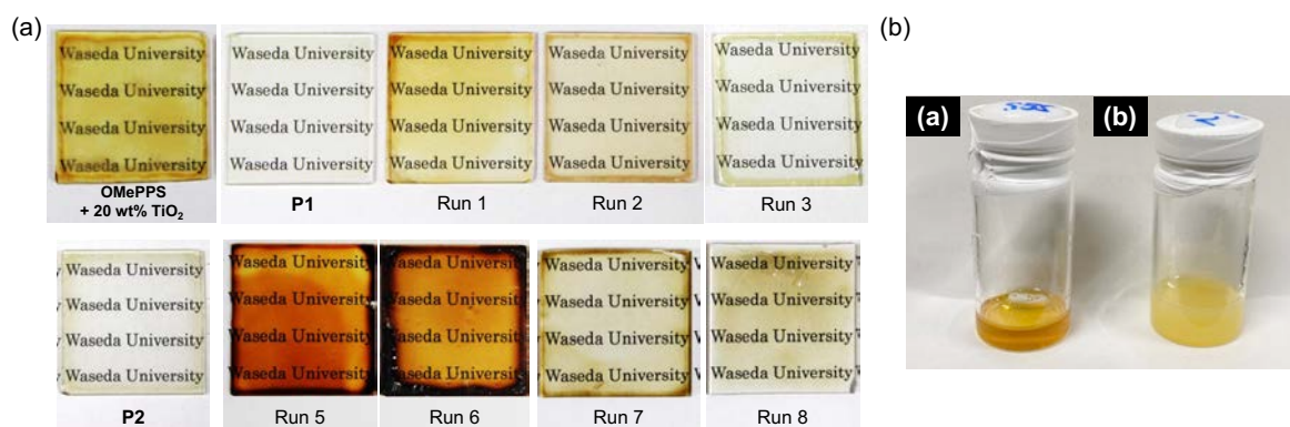
Figure 2.14. (a) Thin films of OMePPS with 20 wt% \text{TiO}_2 , P1 and its hybrid films (Runs 1-3 in Table 2.4), and P2 and its hybrid films (Runs 5-8 on glass substrates. (b) Precursor solution for P1 with (a) 10 wt% \text{ZrO}_2 hybrid (Run 3 in Table 4) and (b) 30 wt% \text{ZrO}_2 hybrid (Run 4 in Table 4) after stirring at r.t.
