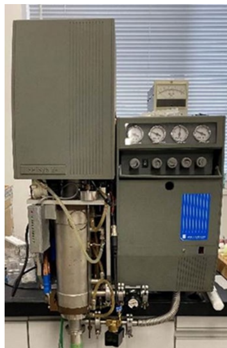
Figure 1.15. Differential thermal analysis machine SETARAM SETSYS-24 used at NIMS.
