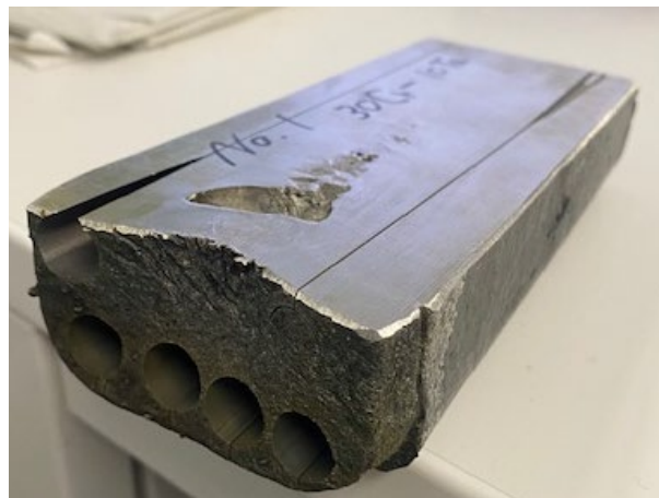
Figure 1.17. Bulk (3.5 kg) of CoCrTa after cutting cylinders for tensile tests via EDM.
