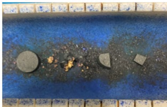
Figure 3.13. Appearance of samples after 20 one-hour cycles at 1200 °C in air.
