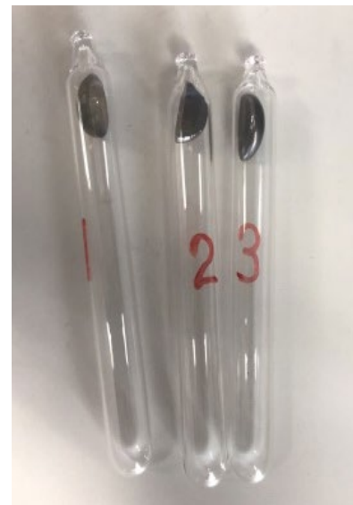
Figure 1.12. Samples sealed in quartz ampoule with argon gas.
