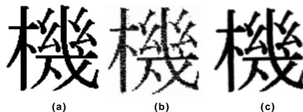
Fig. 15 Original bit image (a), first (b) and second (c) stage print sample.
