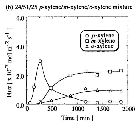
Fig. 7. Pervaporation results for xylene isomers at 303 K through MFI-type zeolitic membrane.
