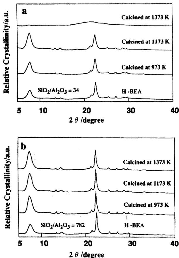
Fig. 5. X-ray diffraction pattern of H-forms of BEA-30-1 (a) and BEA-730-1 (b) calcined at different temperatures (indicated in the figure).
