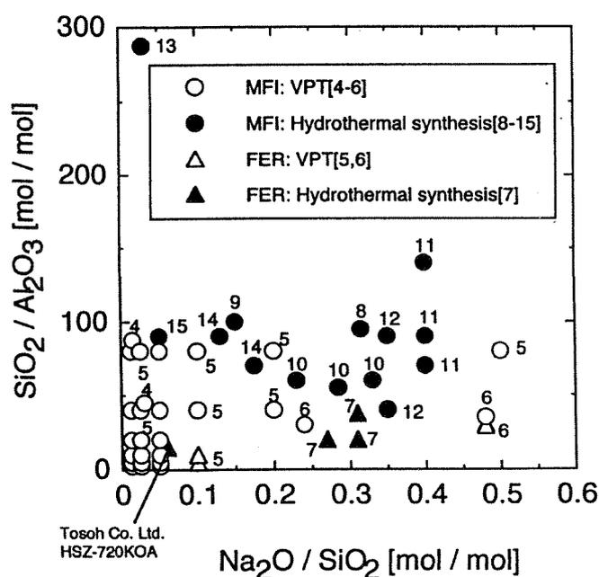
Figure 2. Compositions of parent gels for synthesis of MFI and FER. Figures given in the neighborhood of each plot correspond to the reference numbers.
