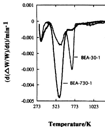
Fig. 4. DTG patterns of  $\text{TEA}^+$  ions occluded in as-synthesized BEA-30-1 and BEA-730-1 in a stream of  $\text{N}_2$ .
