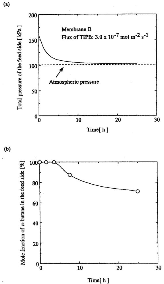
Fig. 7. Time course of (a) the total pressure of feed side and (b) the mole fraction of *n*-butane in the feed side with membrane B. Temperature: 375 K.
