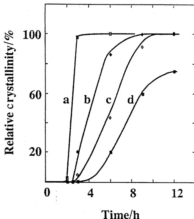
Figure 4. Crystallization curves of BEA with different chemical compositions at 453 K.  $\text{SiO}_2/\text{Al}_2\text{O}_3$ ,  $\text{SiO}_2/\text{Na}_2\text{O}$  and  $\text{SO}_4^{2-}/\text{SiO}_2$  ratios: (a) 30, 23.8 and 20.9; (b) 380, 23.8 and 528; (c) 730, 10.9 and 10; (d) 730, 23.8 and 0, respectively.
