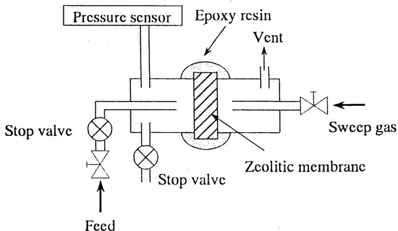
Fig. 1 Schematic diagram of experimental apparatus for permeation measurements.
