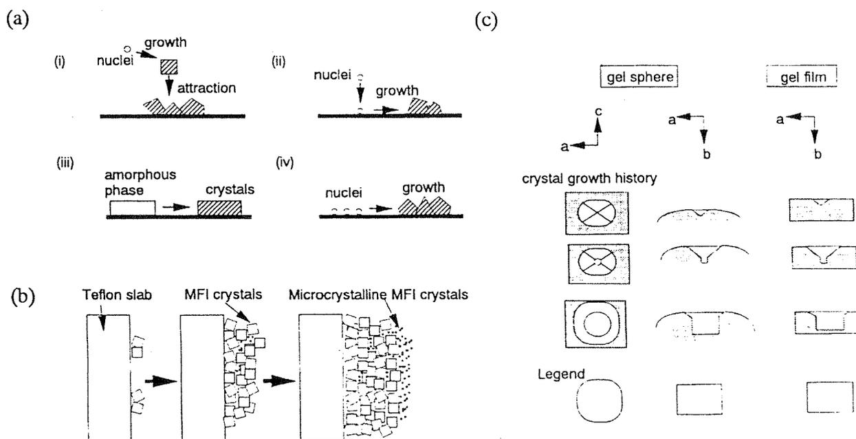
Fig. 1. Proposed growth mechanisms of zeolitic membranes. a) Sano et al.,<sup>21</sup> b) Myatt et al.,<sup>44</sup> and c) Jansen et al.<sup>45</sup>
