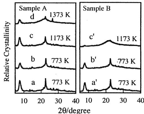
Figure 3. XRD patterns of sample A and B calcined at temperatures indicated in figure. A and a', Na-Beta; b-d and b' and c', H-Beta.
