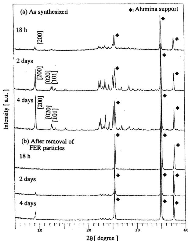
Fig. 2. XRD patterns for FER membranes (a) as synthesized and (b) after removal of FER particles on the alumina support.
