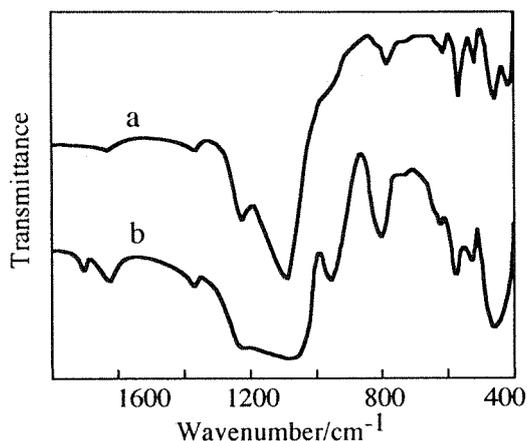
Figure 5. FTIR spectra of Ti-Beta.
