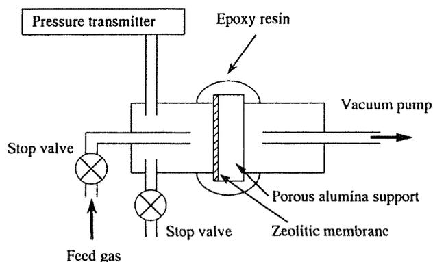
Fig. 2. Schematic diagram of gas permeation measurements.
