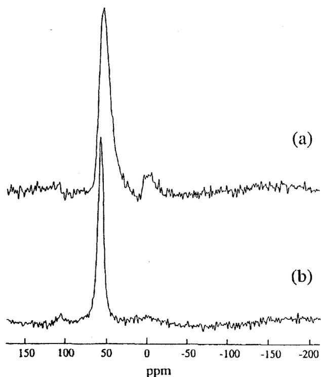
Fig. 6.  $^{27}\text{Al}$  MAS NMR spectra for dry gels. The chemical shift was calibrated by using aqueous 1 N  $\text{Al}_2(\text{SO}_4)_3$ .  $\text{Al}_2\text{O}_3$  source: (a)  $\text{Al}_2(\text{SO}_4)_3$ , (b)  $\text{NaAlO}_2$ .
