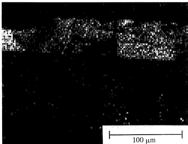
Fig. 5. (a) SEM and (b) EDX elemental images for the cross-section of alumina support coated with aluminosilicate gel. White dots: Si.
