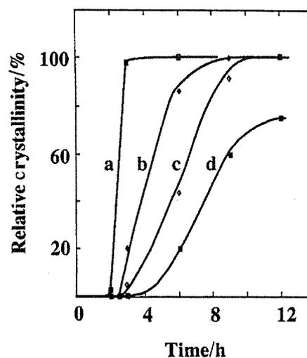
Fig. 3. Rate of crystallization of BEA with different chemical compositions.  $\text{SiO}_2/\text{Al}_2\text{O}_3$ ,  $\text{SiO}_2/\text{Na}_2\text{O}$  and  $\text{SiO}_2/\text{SO}_4^{2-}$  ratios: a, 30, 23.8 and 20.9; b, 380, 23.8 and 528; c, 730, 10.9 and 10; d, 730, 23.8 and 0, respectively.
