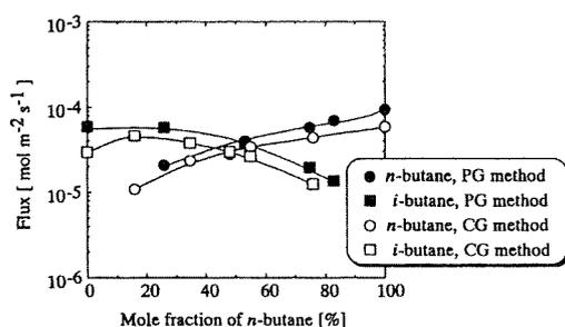
Fig. 8. Fluxes of butane isomers through MFI membranes as a function of mole fraction of *n*-butane in the feed. Temperature: 375 K; closed key: PG method; open key: CG method.
