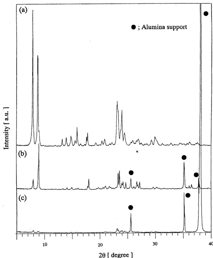
Fig. 3. XRD patterns for (a) MFI powder, (b) as-synthesized membrane and (c) MFI membrane after removal of the top layer.
