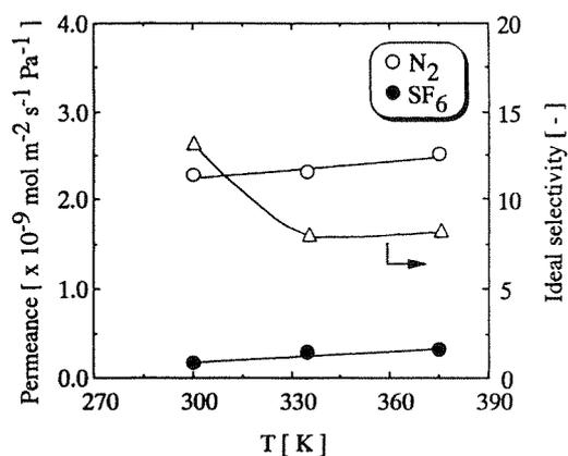
Fig. 5. Permeances of  $N_2$  and  $SF_6$  through an MFI membrane and ideal selectivities of  $N_2/SF_6$  as a function of temperature.
