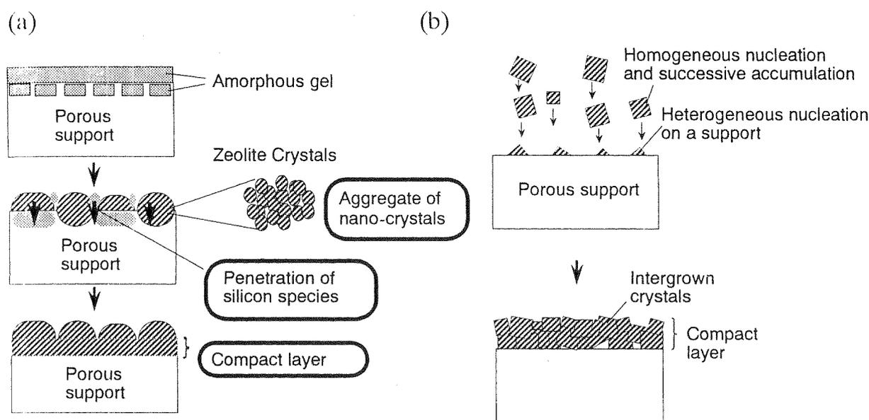
Fig. 6. Plausible formation mechanism of zeolitic membranes (a) by vapor-phase transport method and (b) by hydrothermal synthesis.
