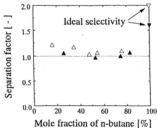
Fig. 2 Flux of butane isomers through MFI-type zeolitic membranes A and B as a function of mole fraction of n-butane in the feed. Temperature: 375 K. Closed key: PG method. Open key: CG method.
