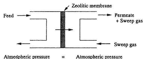
Fig. 3. Schematic diagram of gas permeation measurements.
