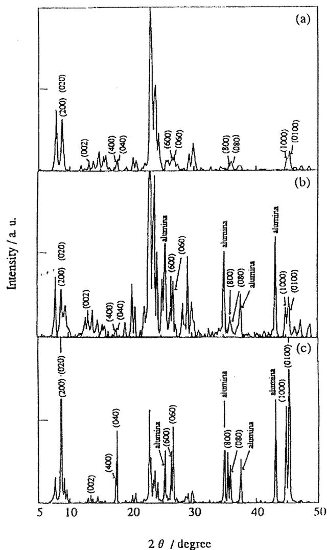
Fig. 2. XRD patterns of zeolites formed on alumina support and powder ZSM-5. (a) Powder ZSM-5 ( $\text{SiO}_2:\text{Al}_2\text{O}_3=23.8$ ). (b) MFI on alumina support prepared using  $\text{Al}_2(\text{SO}_4)_3$ . (c) MFI on alumina support prepared using  $\text{NaAlO}_2$ . Dipping temperature: 293 K, drying condition: 293 K for 3 days followed by 373 K for 2 h.
