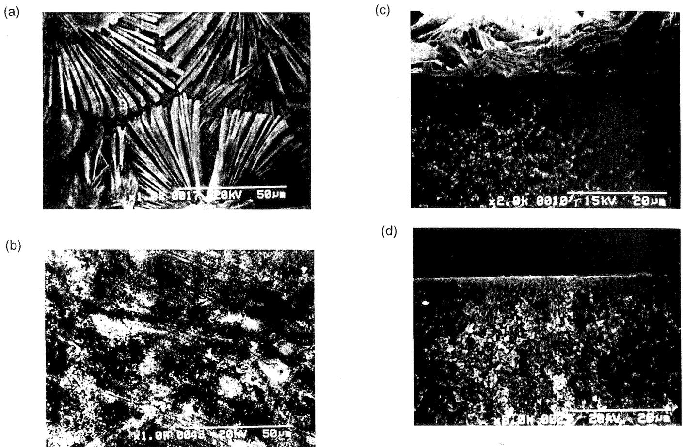
Fig. 2. SEM images for the top views of FER membranes (a) before and (b) after removal of FER particles on alumina support, and the cross-sectional views of FER membranes (c) before and (d) after removal of FER particles on alumina support
