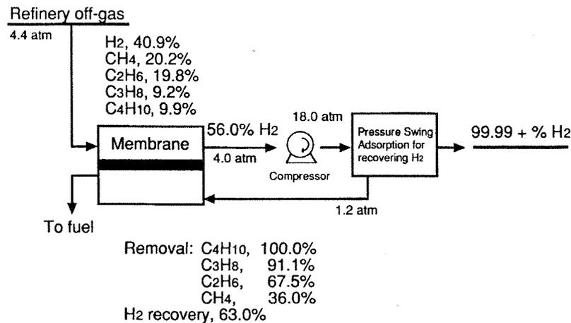
Fig. 2 Mass Balance of H<sub>2</sub> recovery process from refinery waste with SSF membrane.
