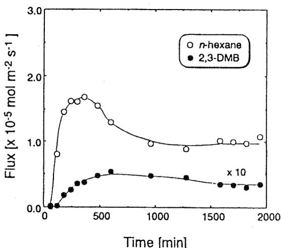
**Figure 4.** Transient profile of fluxes of *n*-hexane and 2,3-dimethylbutane (2,3-DMB) in the pervaporation at 303 K.
