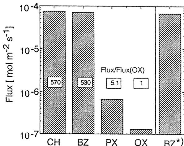
Fig. 14. Pervaporation results for single liquid components using FER membrane. ( $T = 303$  K) CH: cyclohexane, BZ: benzene, PX: *p*-xylene, OX: *o*-xylene. \*) After permeation test for 1,3,5-trisopropylbenzene.
