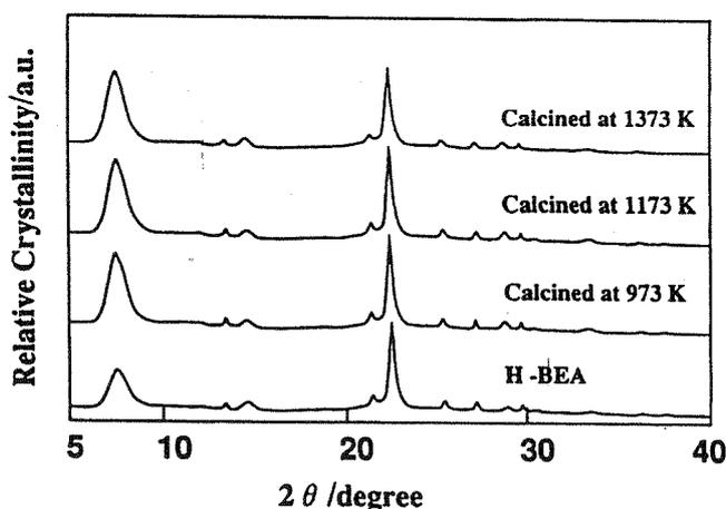
Figure 6. X-ray diffraction patterns of H-exchanged BEA with  $\text{SiO}_2/\text{Al}_2\text{O}_3$  ratio = 782 [23]. Calcination was carried out in air for 2 h.
