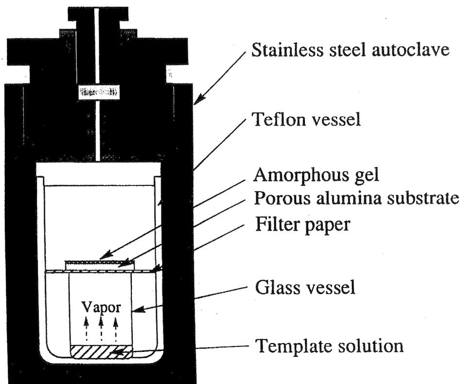
Fig. 1. Schematic illustration of the autoclave used for synthesizing zeolitic membranes by the vapor-phase transport method.
