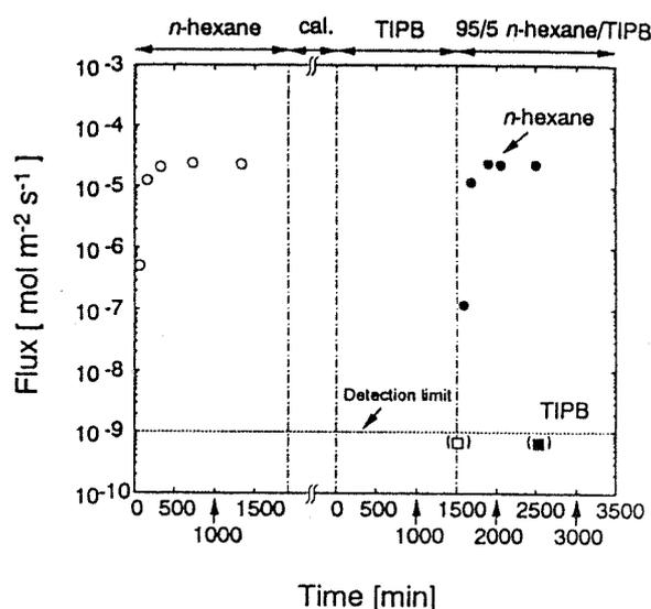
Figure 2. Pervaporation tests for the compactness of MFI membranes: cal, calcination.
