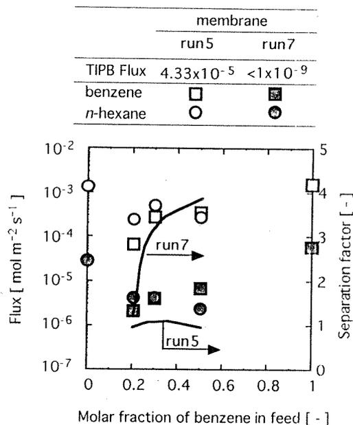
Figure 4 Separation results of benzene/hexane mixtures by pervaporation at 303 K.
