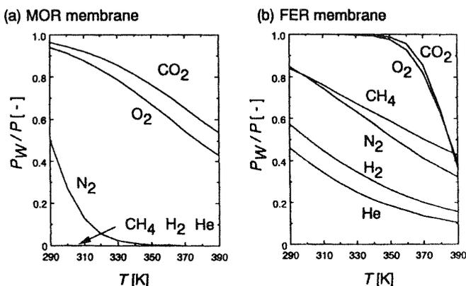
Figure 6. Temperature dependence of *P<sub>w</sub>*/*P*.
