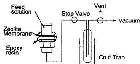
Figure 1. Schematic diagram of experimental apparatus for pervaporation.
