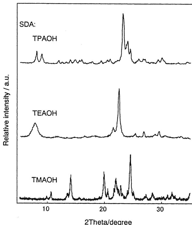
Figure 1. XRD patterns of products obtained by DGC method, using TMAOH, TEAOH, and TPAOH as structure-directing agents.
