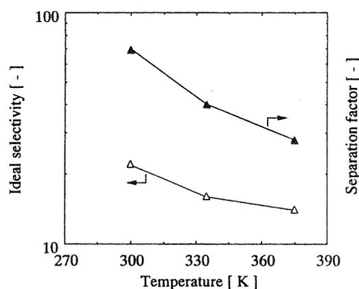
Fig. 6. Permeation results of butane isomers through MFI membrane. Open key: unary system. Closed key: 52/48 *n*-butane/*i*-butane mixed-gas system.
