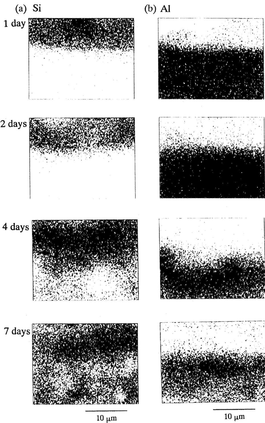
Fig. 3. EDX elemental cross-sectional images of FER membranes crystallized for 1, 2, 5 and 7 days. Black dots: (a) Si and (b) Al.
