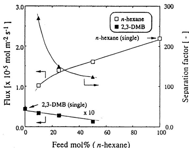
**Figure 5.** Effect of *n*-hexane feed concentration on the fluxes of *n*-hexane and 2,3-DMB and the separation factor of *n*-hexane/2,3-DMB mixtures using an MFI membrane.
