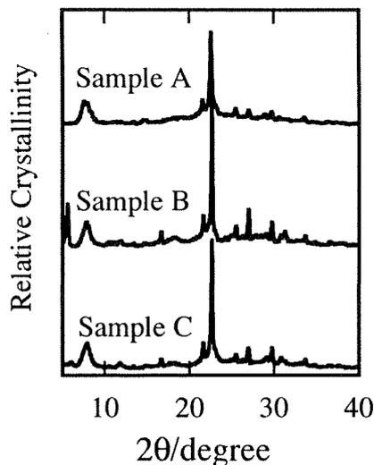
Figure 1. XRD patterns of as-synthesized pure silica Beta and Al-free Ti-Beta.
