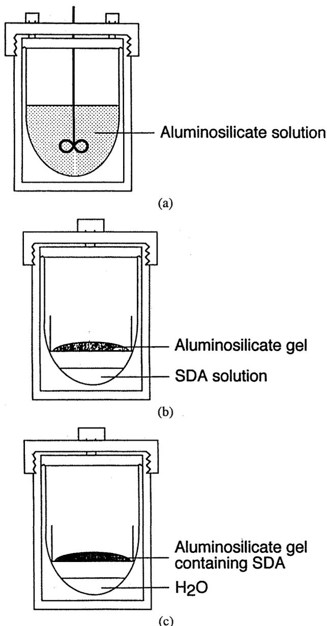
Figure 1. Schematic diagram of the methods for microporous crystal synthesis. (a) Hydrothermal method, (b) vapor-phase transport (VPT) method, and (c) steam-assisted crystallization (SAC) method. The latter two are the dry gel conversion (DGC) methods.
