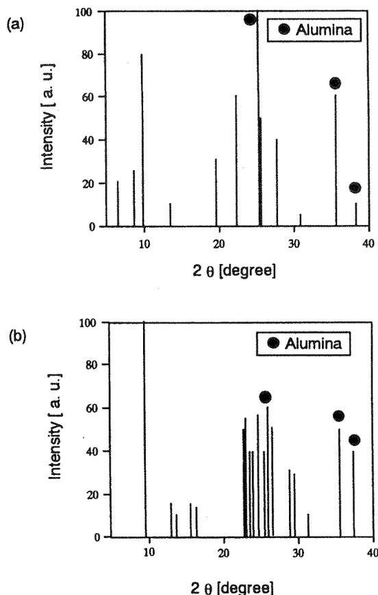
Figure 1. XRD patterns for (a) MOR and (b) FER membranes.
