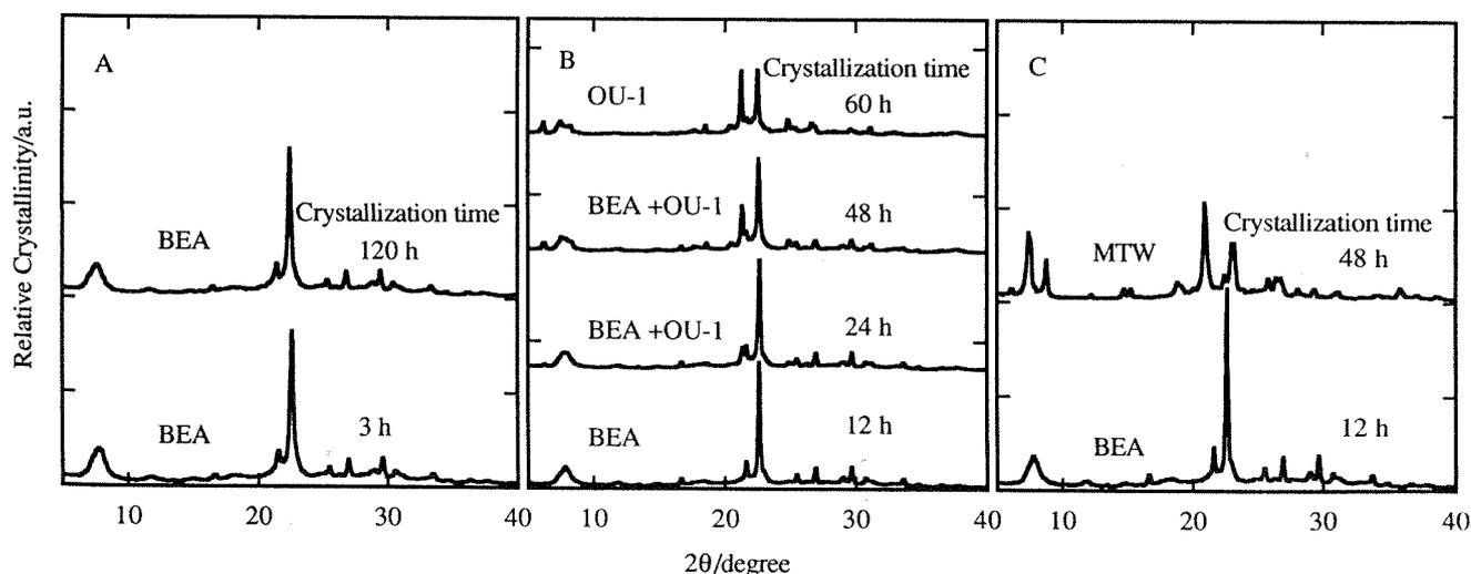
**Figure 1.** Effect of gel composition and crystallization time on zeolite product. SiO<sub>2</sub>/Al<sub>2</sub>O<sub>3</sub> and Na<sub>2</sub>O/SiO<sub>2</sub> ratios : A, 30 and 0.042; B, 380 and 0.042; C, 730 and 0.094, respectively.
