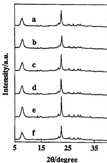
Fig. 4. X-ray diffraction patterns of calcined BEA with different  $\text{SiO}_2/\text{Al}_2\text{O}_3$  ratios.  $\text{SiO}_2/\text{Al}_2\text{O}_3$  ratios: a, 30; b, 100; c, 200; d, 380; e, 480; f, 730.
