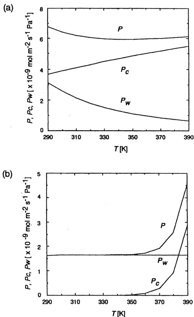
Figure 5. *P*, *P<sub>c</sub>*, and *P<sub>w</sub>* for (a) He and (b) CO<sub>2</sub> through FER membrane.
