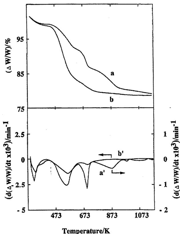
Fig. 7. TG-DTG patterns of BEA samples treated in the stream of air. a and b: TG patterns for BEA with SiO<sub>2</sub>/Al<sub>2</sub>O<sub>3</sub> ratios 30 and 730, respectively; and a' and b': DTG patterns for BEA with SiO<sub>2</sub>/Al<sub>2</sub>O<sub>3</sub> ratios 30 and 730, respectively.
