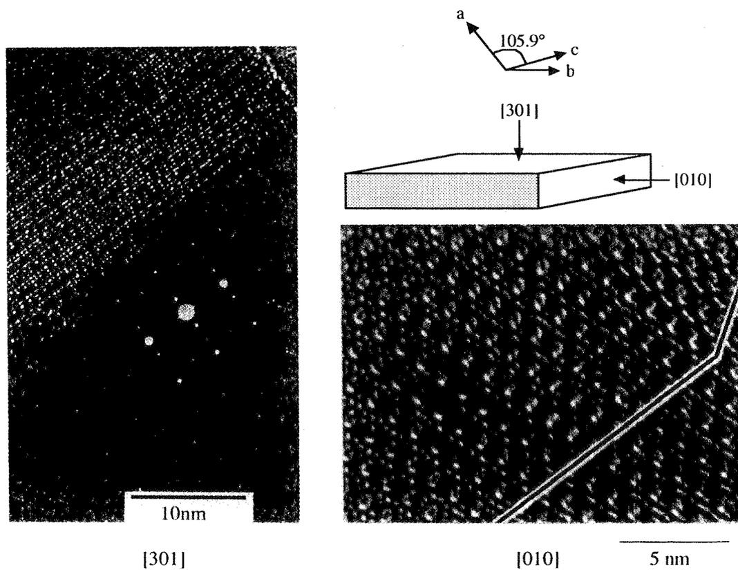
Fig. 4 HRTEM images for OU-1 observed along  $[301]$  and  $[010]$  directions which are indicated in figure.
