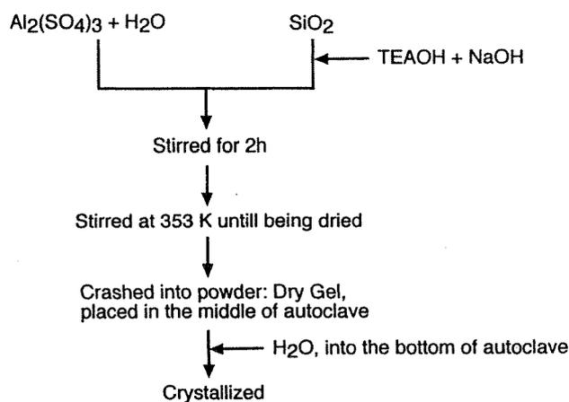
Figure 3. Typical synthetic method of zeolite BEA by the SAC method.
