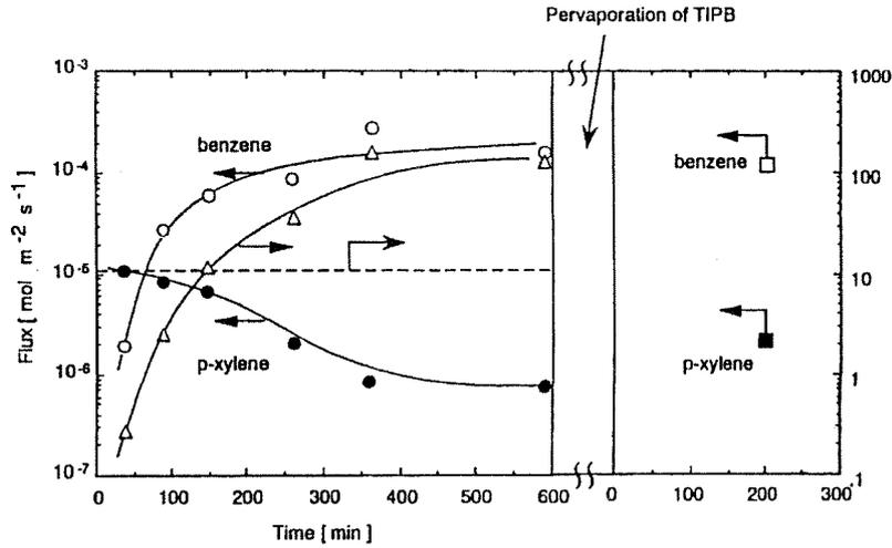
Fig. 3 Pervaporation results for a benzene/p-xylene mixture through a MOR membrane at 295 K.
