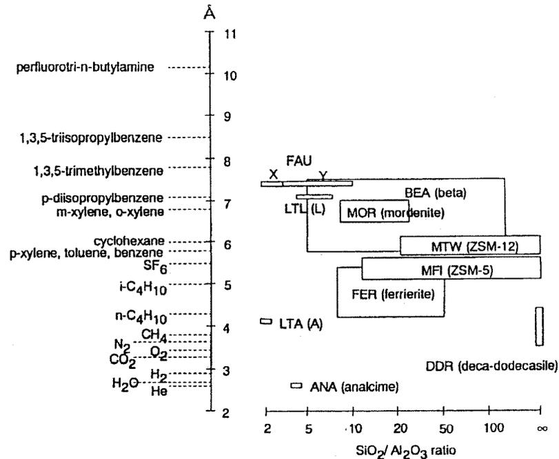
Fig. 1 Relation between micropore size of zeolite and molecular diameter.
