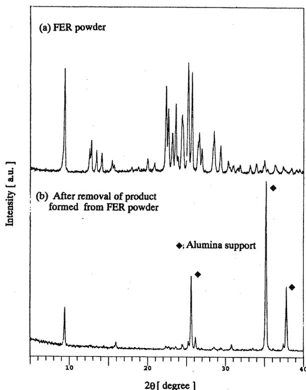
Fig. 7. XRD patterns for (a) FER powder and (b) after removal of the product formed from FER powder placed on the support using the VPT method.
