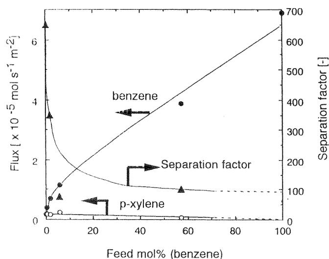
Fig. 7. Effect of benzene feed concentration on flux of benzene and *p*-xylene and separation factor in pervaporation of benzene/*p*-xylene mixtures. ( $T=303 \text{ K}$ ) ●, flux of benzene, ○, flux of *p*-xylene, ▲, separation factor.
