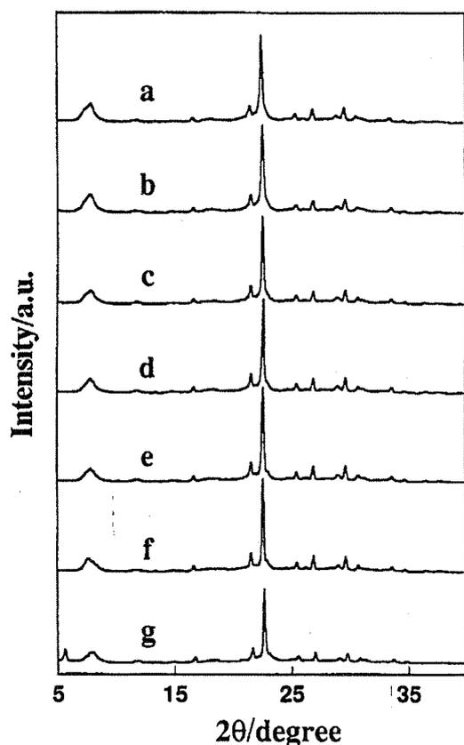
Fig. 2. X-ray diffraction patterns of as-synthesized BEA with different  $\text{SiO}_2/\text{Al}_2\text{O}_3$  ratios.  $\text{SiO}_2/\text{Al}_2\text{O}_3$  ratio: a, 30; b, 100; c, 200; d, 380; e, 480; f, 730; g, infinity.
