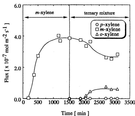
Fig. 8. Pervaporation results of a ternary mixture of xylene isomers after the permeation measurement of *m*-xylene. Composition of ternary mixture: *p*-xylene, 24 mol%; *m*-xylene, 51 mol%; *o*-xylene, 25 mol%.
