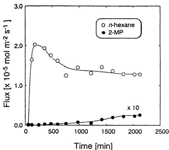
**Figure 3.** Transient profile of fluxes of *n*-hexane and 2-methylpentane (2-MP) in separating the 50/50 *n*-hexane/2-MP binary mixture at 303 K.
