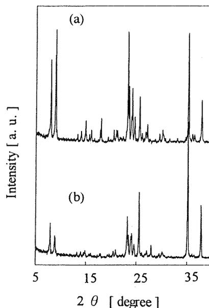
Figure 1 XRD patterns (a) for the as-synthesized membrane (Run 7) and (b) the membrane (Run 7) after removing the top layer.
