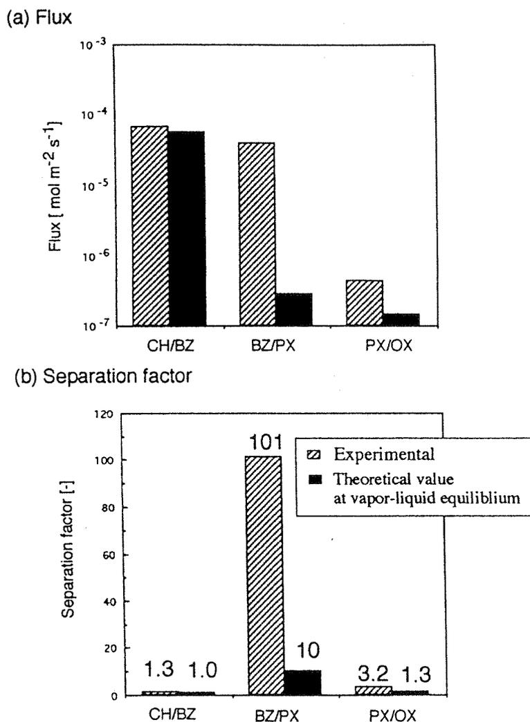
Fig. 15. Pervaporation results for mixtures using FER membrane at 303 K. CH: cyclohexane, BZ: benzene, PX: *p*-xylene, OX: *o*-xylene. Feed mole ratios of CH/BZ, BZ/PX, and PX/OX were 0.95, 1.34, and 0.96, respectively.
