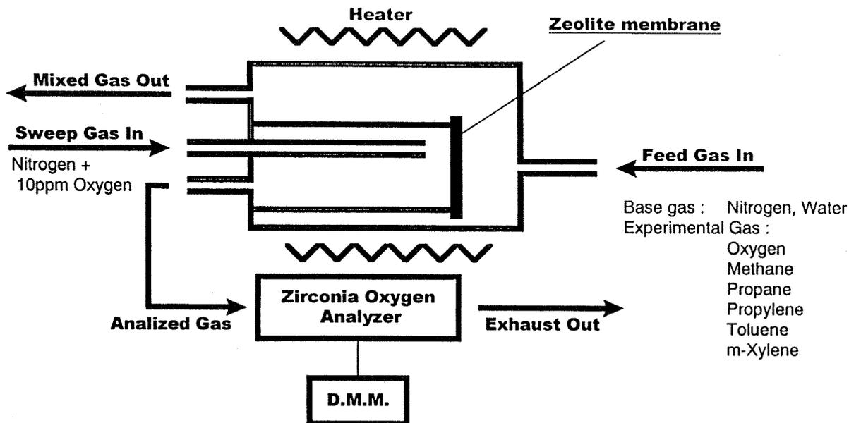
Figure 1. Schematic representation of experimental apparatus for gas permeation.
