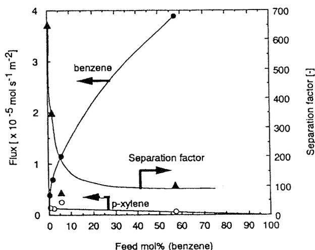
Fig. 16. Effect of benzene feed concentration on the fluxes of benzene and *p*-xylene and separation factor in pervaporation of benzene/*p*-xylene mixtures using FER membranes. Temperature: 303 K, ●: flux of benzene, ○: flux of *p*-xylene, △: separation factor.
