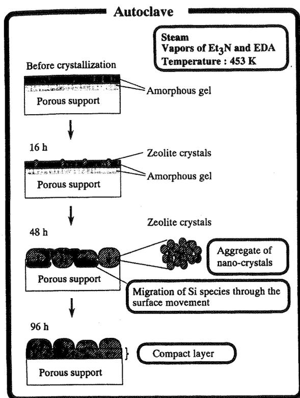
Fig. 9. Plausible formation process of FER membranes by the vapor-phase transport method.
