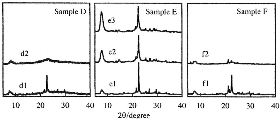
Figure 4. Comparison of thermal stability of samples D, E and F. D1, e1 and f1, as-synthesized; d2, e2 and f2, calcined at 723 K; e3, calcined at 1373 K.
