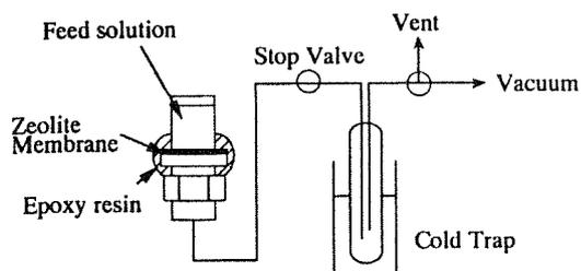
Fig. 1. Schematic diagram of the experimental apparatus for pervaporation.
