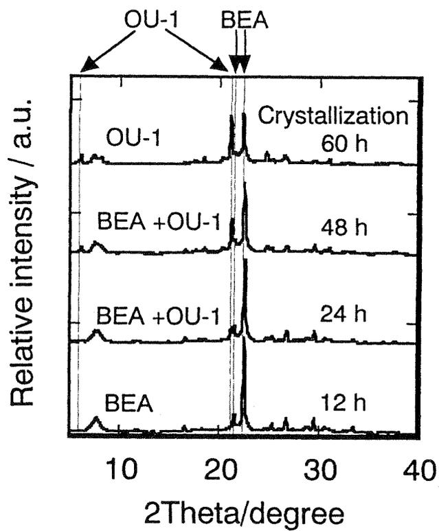
Figure 2. XRD patterns during phase transformation of BEA into OU-1.
