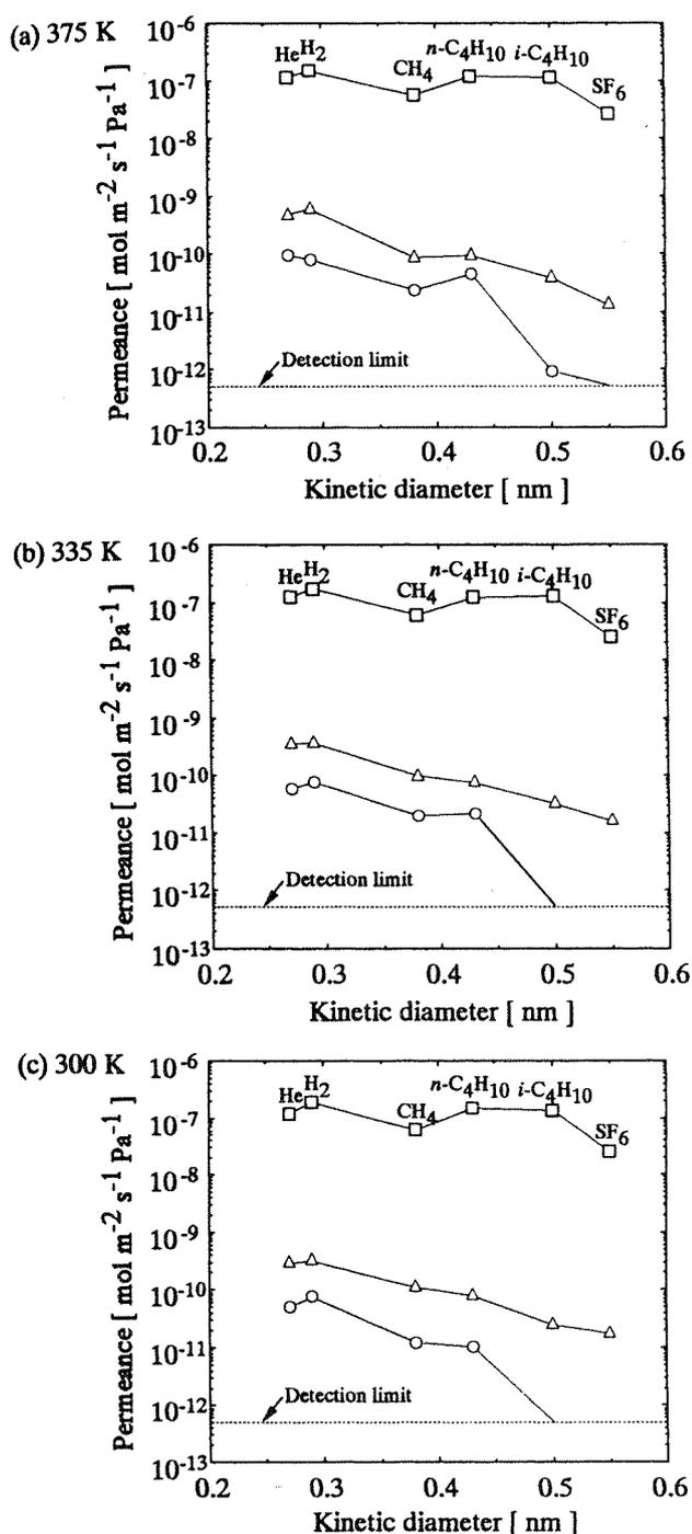
Fig. 1. Pure gas permeances through FER membranes as a function of the kinetic diameter of the molecules: ○: membrane A, △: membrane B, □: membrane C.
