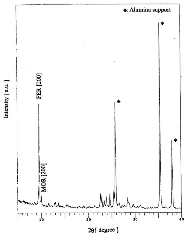
Fig. 5. XRD patterns for the product formed from gel powder on the support by the VPT method.
