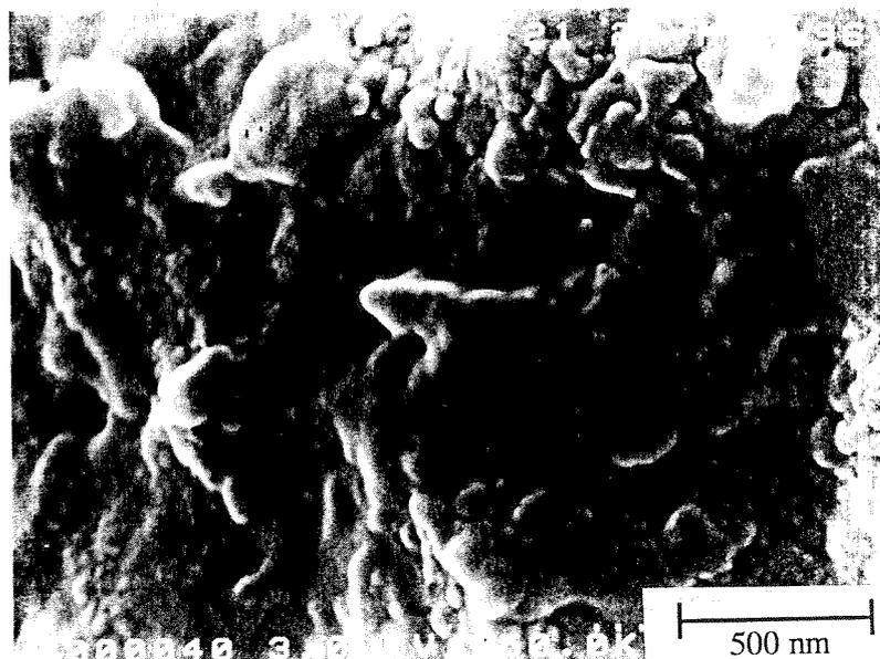
Fig. 3. FE-SEM images for the cross-section of (a) porous alumina support and (b) FER membrane.
