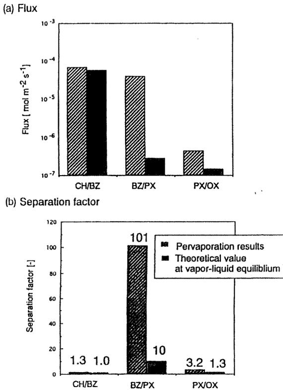
Fig. 4 Pervaporation results for mixtures using an FER membrane at 303 K.
