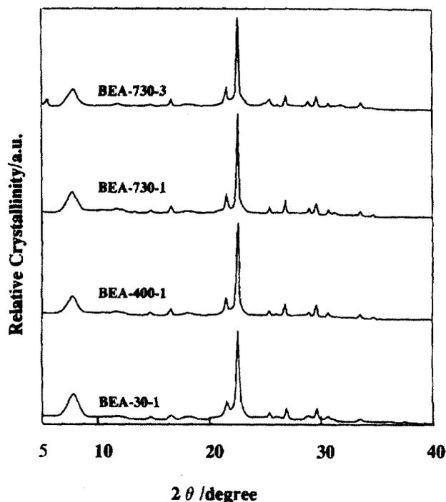
Fig. 1. X-ray diffraction patterns of as-synthesized BEA.
