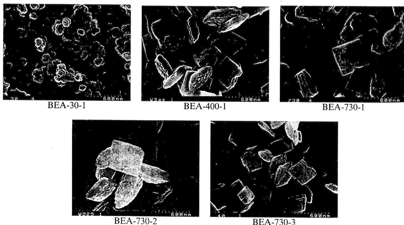
Fig. 2. FE-SEM images for BEA crystallized from gels having different compositions and at different temperatures.
