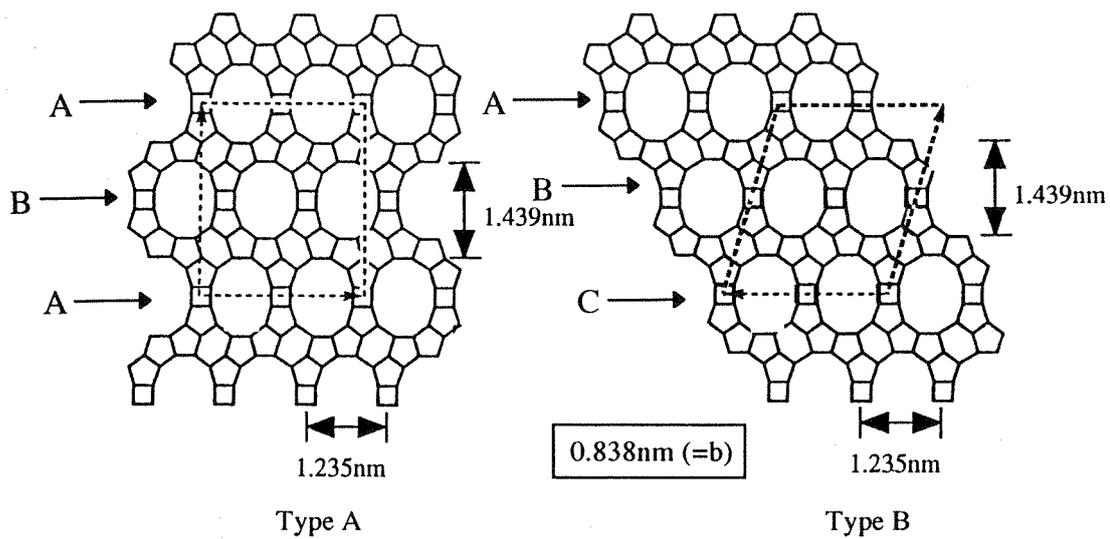
Fig. 3 Framework structures of OU-1.
