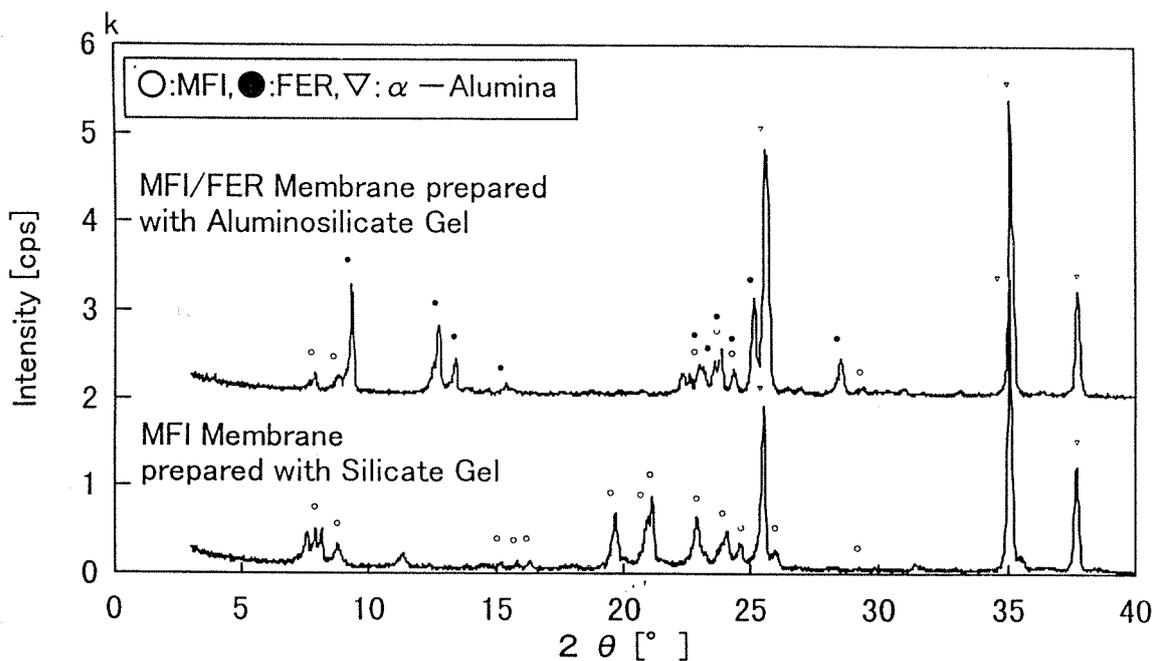
Figure 2. XRD Peak patterns of membranes formed on  $\text{Al}_2\text{O}_3$  substrate.
