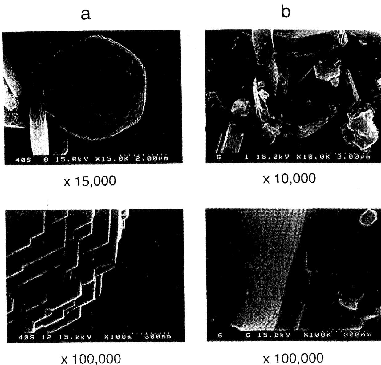
Figure 10. Field emission-SEM images for EMT synthesized by (a) the hydrothermal method and (b) the SAC method.
