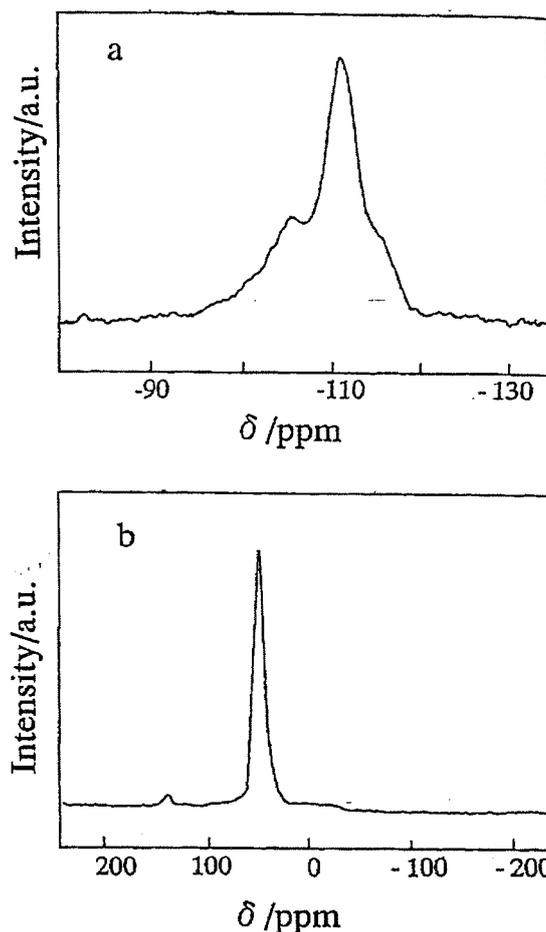
Fig. 5.  $^{29}\text{Si}$ -NMR (a) and  $^{27}\text{Al}$ -NMR (b) spectra of BEA with  $\text{SiO}_2/\text{Al}_2\text{O}_3 = 30$ .
