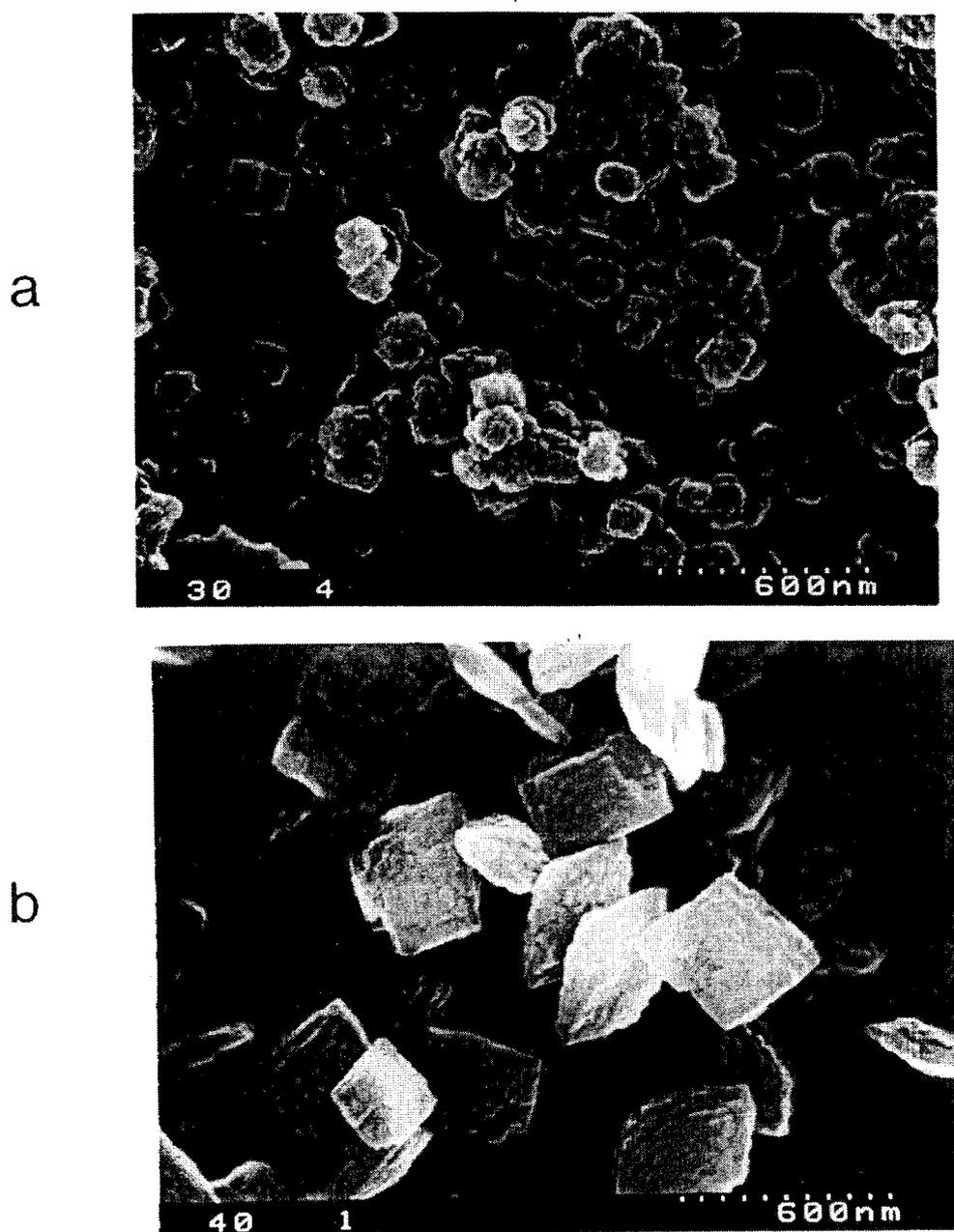
Figure 5. Typical SEM images for BEA synthesized via the SAC method.  $\text{SiO}_2/\text{Al}_2\text{O}_3$  ratio: (a) 30; (b) 730.
