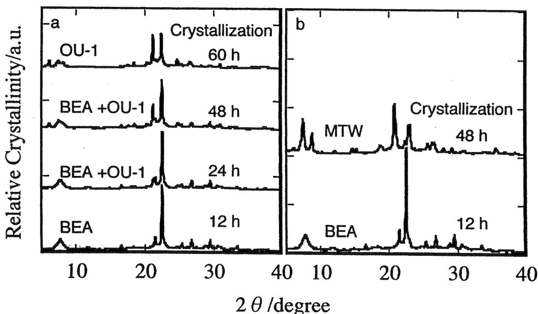
Figure 7. Phase transformation of BEA with prolonged crystallization at 453 K.  $\text{SiO}_2/\text{Al}_2\text{O}_3$  and  $\text{Na}_2\text{O}/\text{SiO}_2$  ratios: (A) 380 and 0.042; (B) 730 and 0.094.
