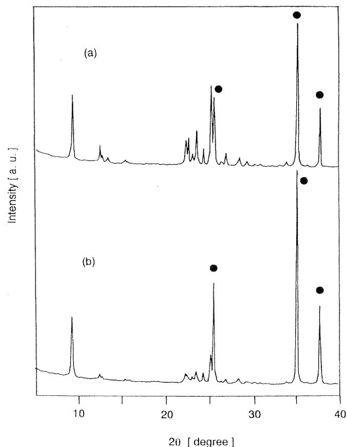
Fig. 1. XRD patterns for FER membranes (a) before and (b) after removal of FER particles on alumina support. Solid symbol, alumina.
