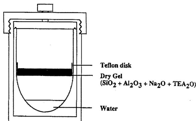
Fig. 1. Schematic diagram of the autoclave used in crystallization of BEA.
