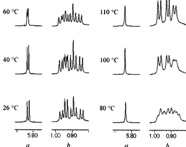
Figure 3. <sup>1</sup>H NMR spectrum of the quinone (**15**) in  $\text{DMSO-}d_6$  at various temperatures: (a) H6'; (b) H7', 8', and 9'.
