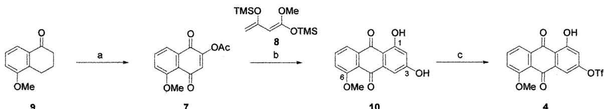
**Scheme 2.** Synthesis of anthraquinone 4. Reagents and conditions: (a) O<sub>2</sub>, *t*-BuOK, *t*-BuOH, rt, 45 min, then Ac<sub>2</sub>O, rt, 2 h, 47%; (b) 8, toluene, 110 °C, 23 h, then pyridine, DMAP, 110 °C, 1.5 h, 70%; (c) TfCl, NaHMDS, HMPA, THF, 0 °C, 5 min, 74%.
