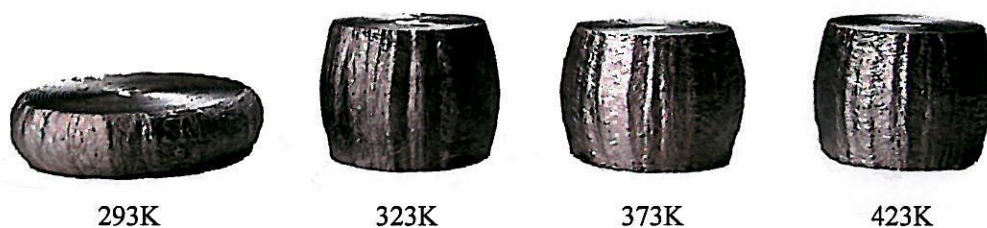
Fig.39 Zn barrel deformation on each temperature
