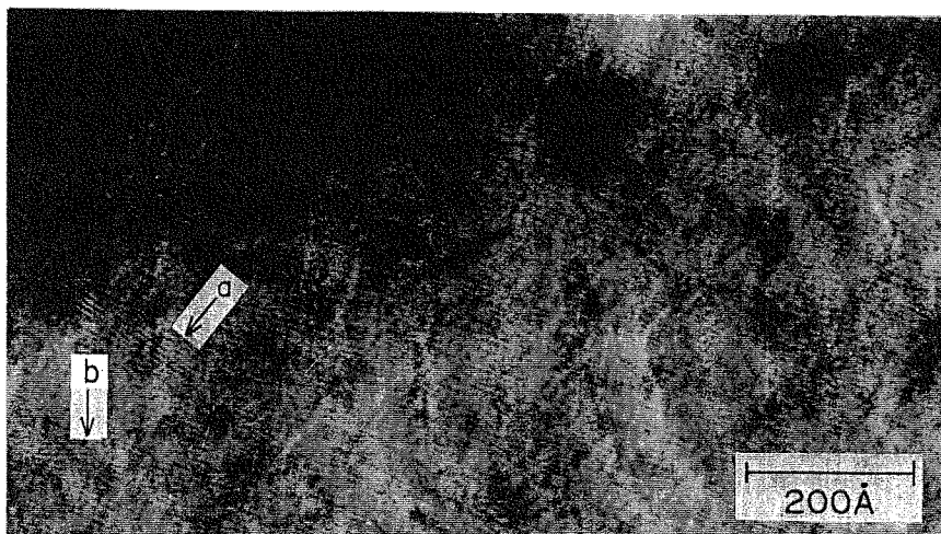
Fig. 9. Typical example of TEM bright field image for electroless-plated CoB film of 50 nm thick. (a) Region of moiré's junction; (b) region of moiré's disappearance.
