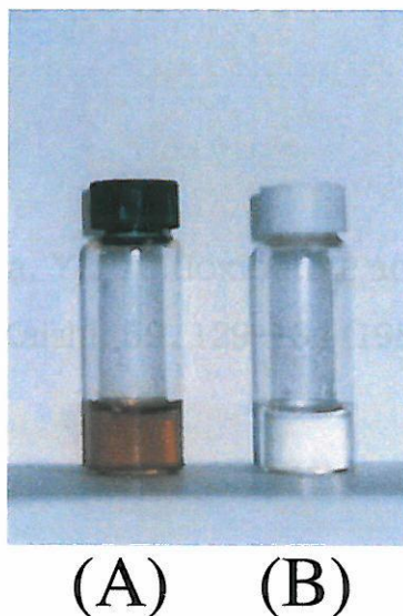
Fig. 1.6. Stability of (+)-catechin and \alpha -C-G in solution. (+)-Catechin and \alpha -C-G were dissolved in 10 mM citrate-10 mM \text{Na}_2\text{HPO}_4 buffer (pH 7.0). After 24 h in contact with air at 20°C, the solution containing (+)-catechin (A) turned brown, whereas the one containing \alpha -C-G (B) did not.
