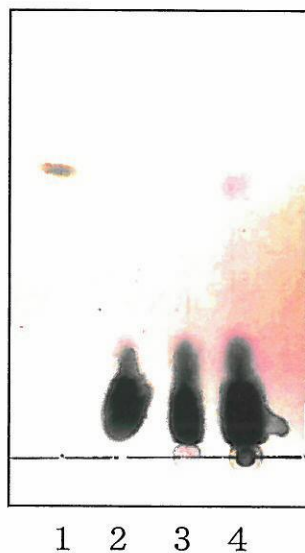
Fig. 6.1. Thin-layer chromatogram of the reaction products. Lanes: 1, 10 mM arbutin; 2, glucose and hydroquinone; 3, glucose and glucosidase; 4, glucose, hydroquinone and glucosidase.
