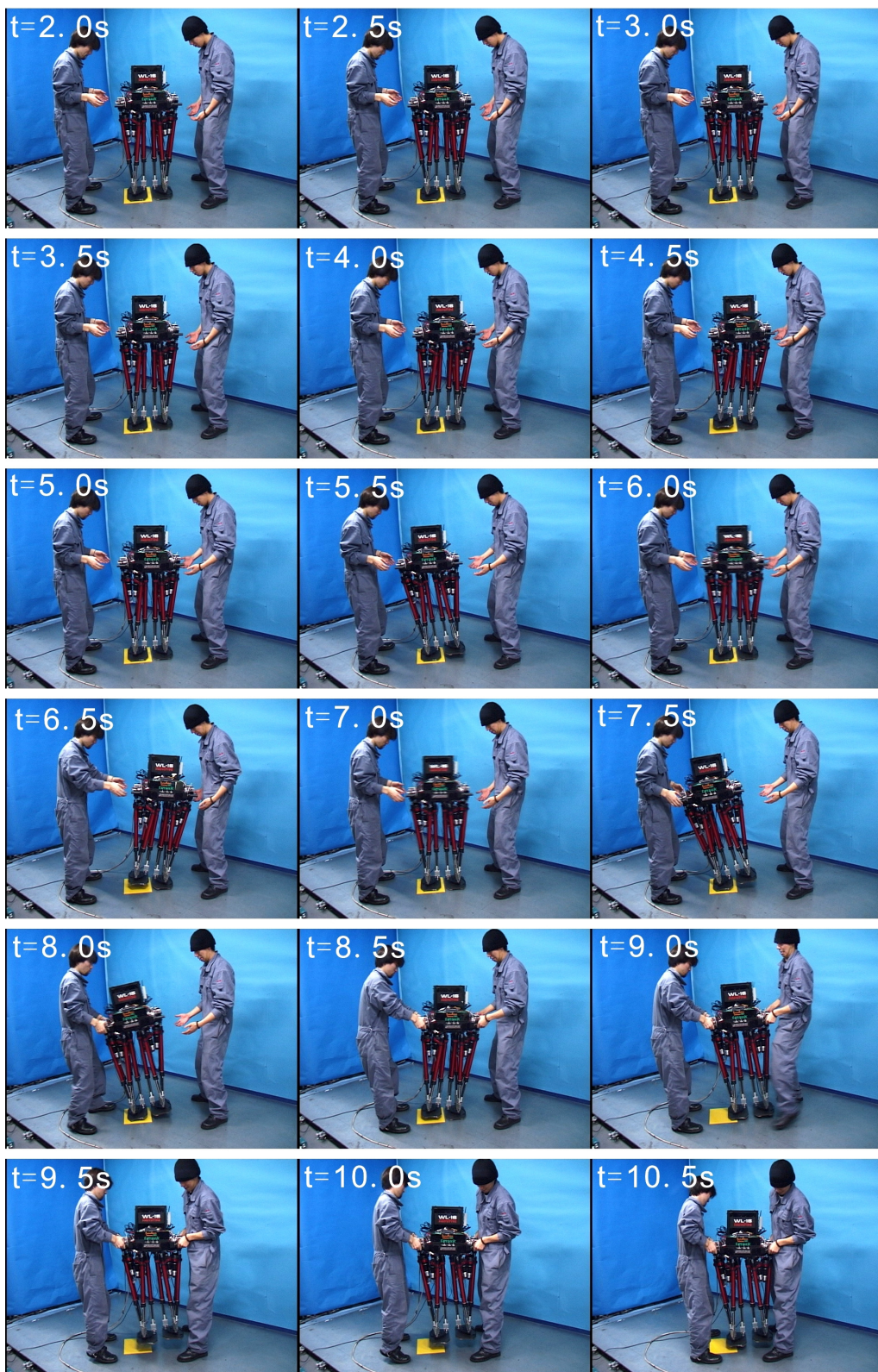
Figure 3.16 Stepping experiment of WL-16. (Stepping, walking cycle: 0.96 s/step, height of unevenness: 5 mm)
