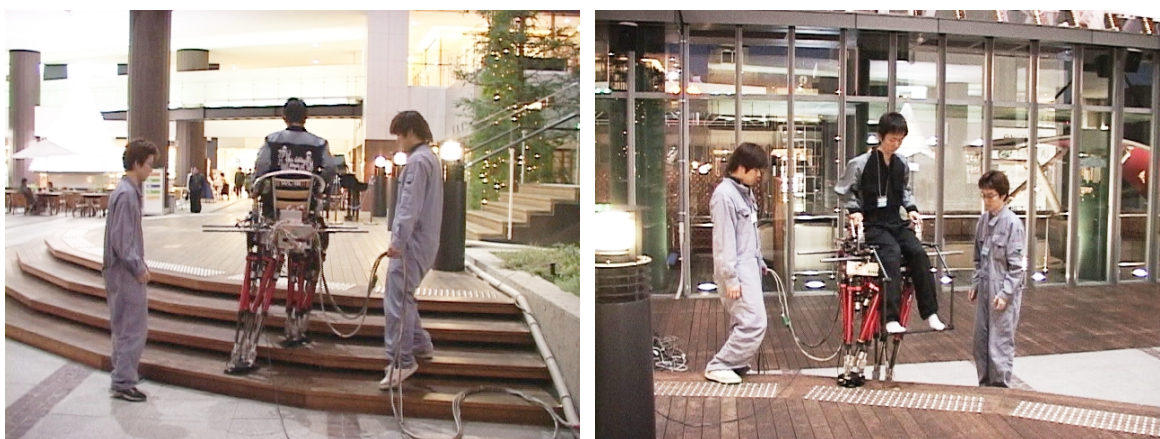
Figure 6.20 Walking experiment involving ascending the stairs of a shopping complex carrying a human.
