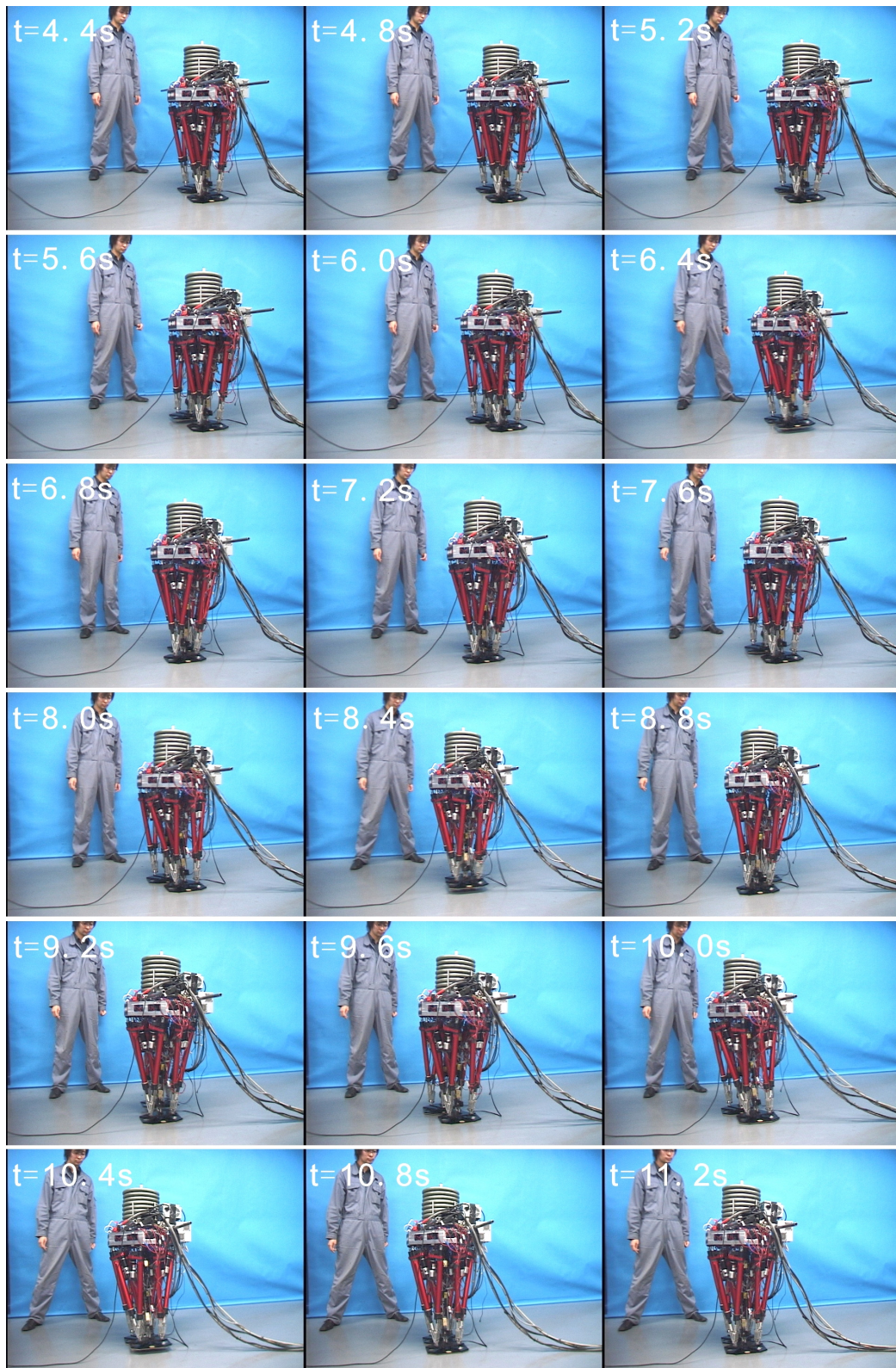
Figure 4.21 Walking experiment carrying a 80 kg load. (Walking forward, walking cycle: 0.96 s/step, step length: 100 mm/step, load: 80 kg)
