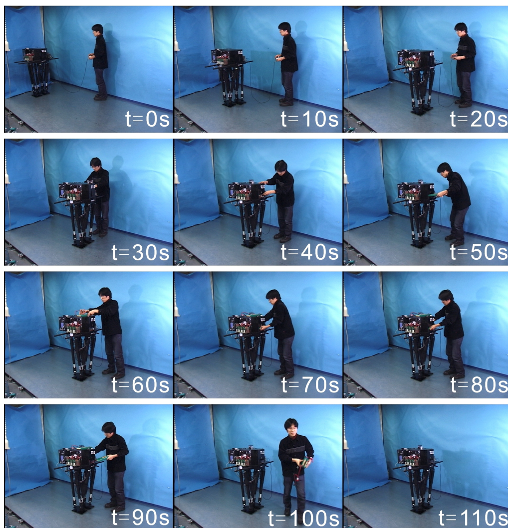
Figure 2.32 Posture holding experiment of WL-15 without power supply. (Walking forward, walking cycle: 0.96 s/step, step length: 100 mm/step)
