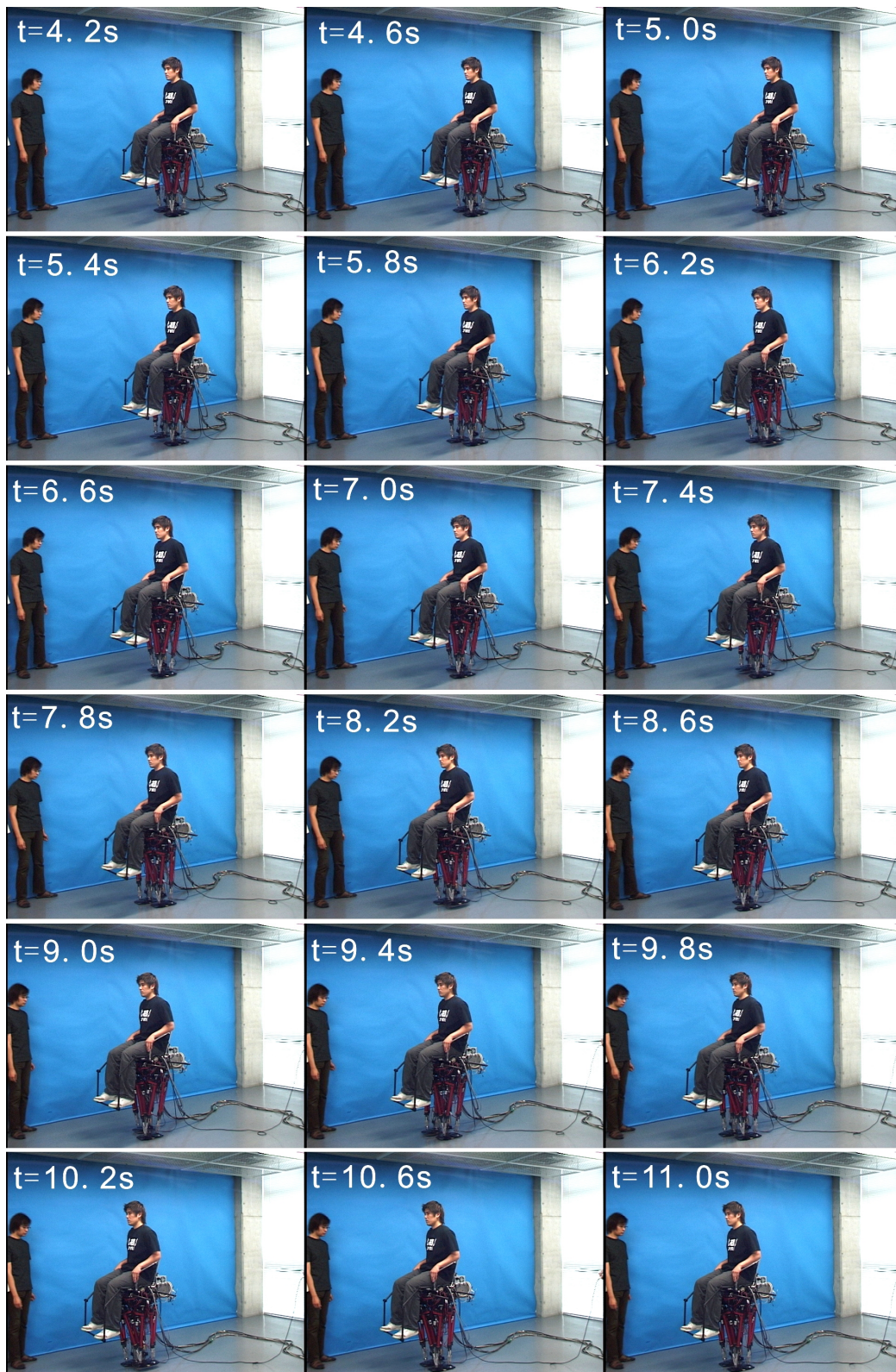
Figure 4.24 Walking experiment carrying a 94 kg adult man. (Walking forward, walking cycle: 0.96 s/step, step length: 100 mm/step, load: a 94 kg adult man)
