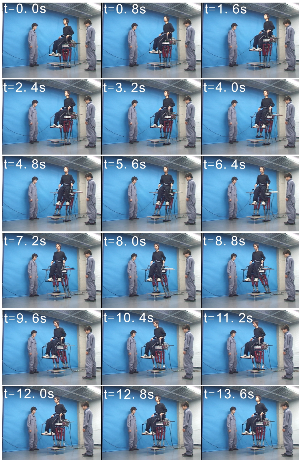
Figure 6.16 Walking experiment ascending a stair with a rise of 200 mm and pedal tread of 300 mm carrying a 60 kg adult man.
