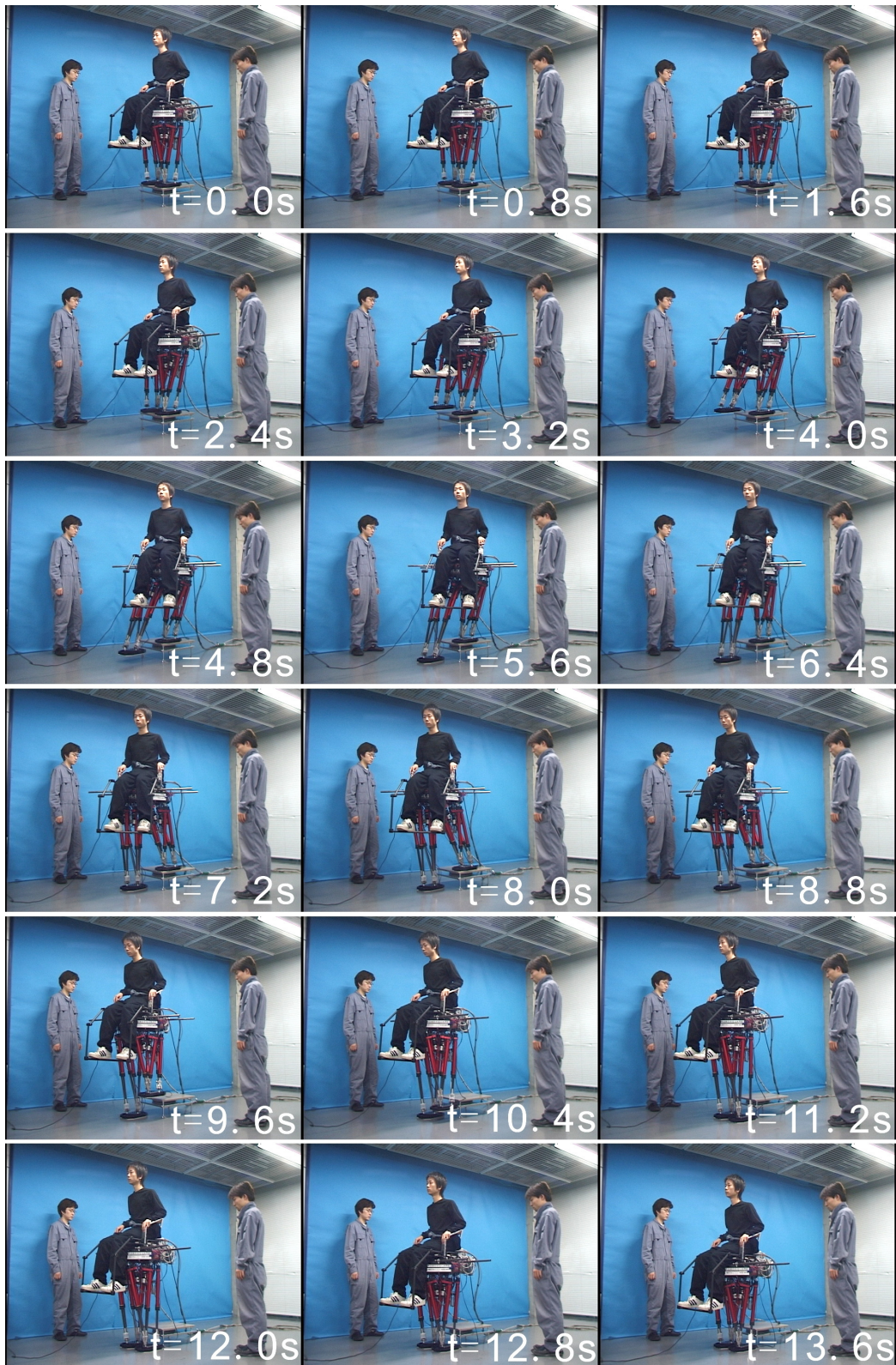
Figure 6.17 Walking experiment descending a stair with a rise of 200 mm and pedal tread of 300 mm carrying a 60 kg adult man.
