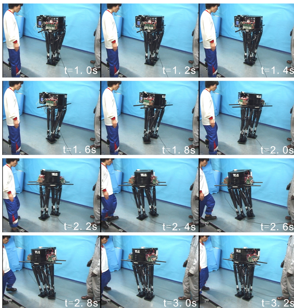
Figure 2.30 Turning experiment of WL-15. (90 deg in 2 steps)
