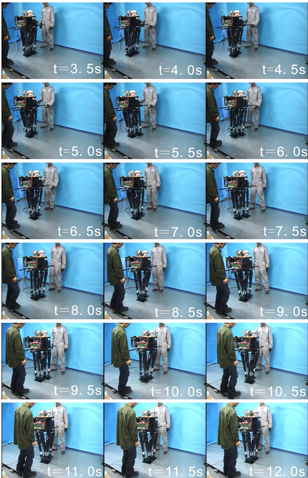
Figure 2.31 Walking experiment of WL-15 carrying 18 kg payload. (Walking forward, walking cycle: 0.96 s/step, step length: 100 mm/step, load: 18 kg)
