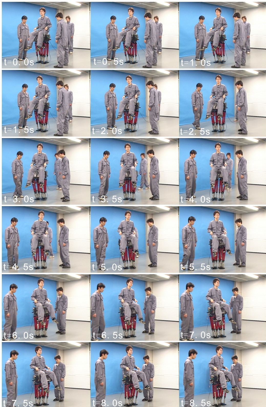
Figure 3.27 Walking experiment carrying a 60 kg adult man. (Turning walking, walking cycle: 0.96 s/step, load: a 60 kg adult man)
