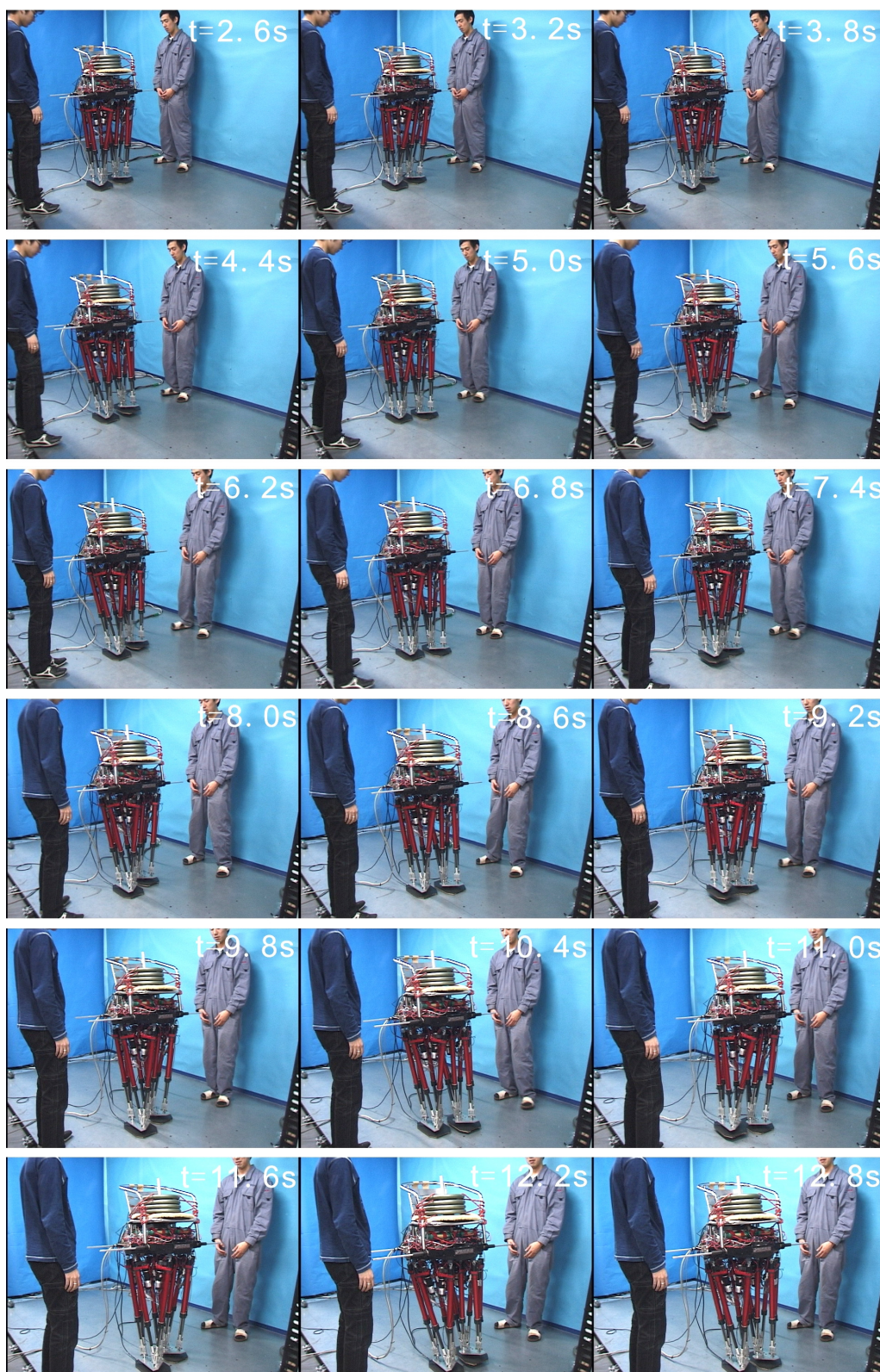
Figure 3.22 Walking experiment carrying 50 kg load.
