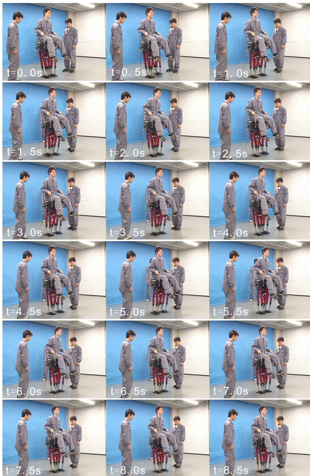
Figure 3.28 Walking experiment carrying a 60 kg adult man. (Walking leftward, walking cycle: 0.96 s/step, step length: 100 mm/step, load: a 60 kg adult man)
