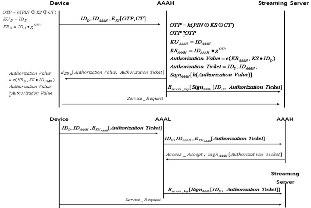
Figure 7.11 IPTV device authentication phase protocol in foreign network
