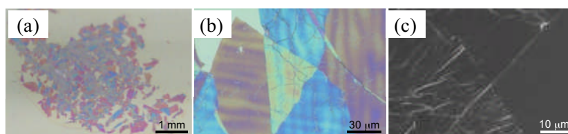
Fig. 5.9 Macroscopic (a) and microscopic (b,c) images of fragmented PLLA nanosheets adhered on the SiO 2 substrate obtained using a digital camera, a digital microscope, and a scanning electron microscope, respectively.
