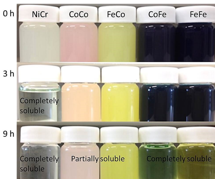
Figure 2.15. Dissolution test of solid NiCr nanocubes, solid CoCo nanocubes, solid FeCo nanocubes, solid CoFe nanocubes, and solid FeFe nanocubes.
