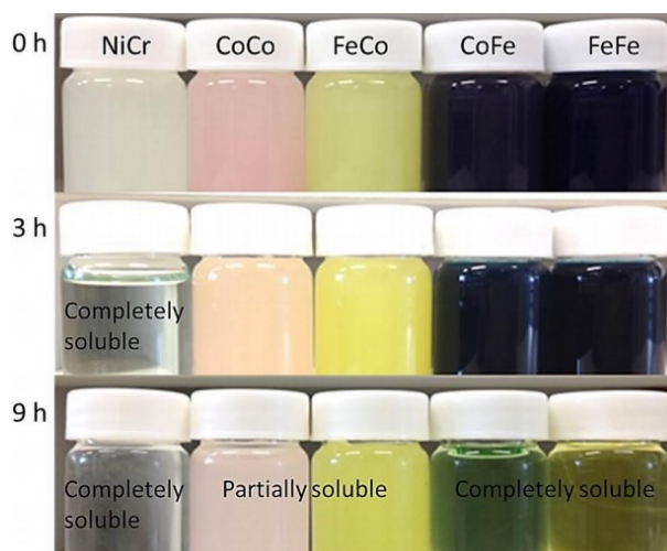
Figure 8.5. Dissolution test of solid NiCr nanocubes, solid CoCo nanocubes, solid FeCo nanocubes, solid CoFe nanocubes, and solid FeFe nanocubes.
