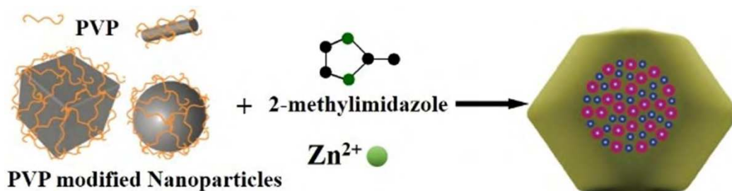
Figure 8.1 Metal nanoparticles encapsulated in an MOF. Reproduced with permission [12]. Copyright 2012, Nature Publishing Group.
