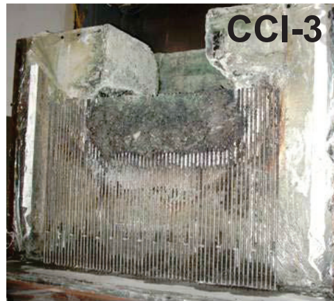
Fig. 1-6 Final cavities showing isotropic and anisotropic ablation patterns in CCI-2 and CCI-3 tests (Farmer et al. 2005)
