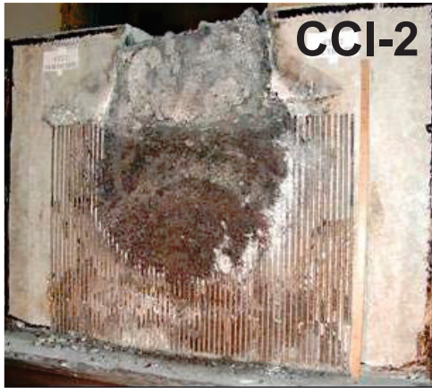
Fig. 1-6 Final cavities showing isotropic and anisotropic ablation patterns in CCI-2 and CCI-3 tests (Farmer et al. 2005)
