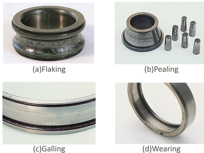
図 4.20 Damage by type: (a)Flaking, (b)Peeling, (c)Galling, (d)Wearing [67]
