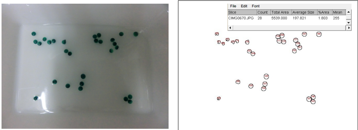
図 5.19 Capsules measurement by ImageJ
