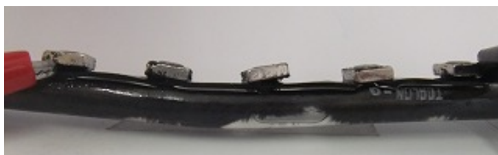
図 3.9 Self-repaired MPW (connected)
