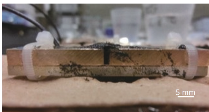
図 4.59 Fe powder trapped on damaged area of material
