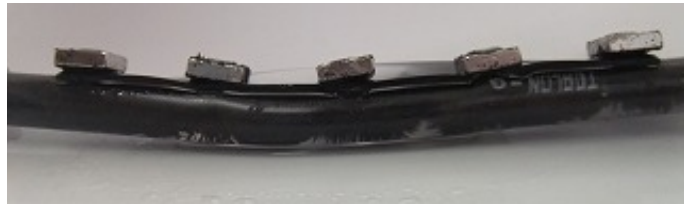
図 3.6 Magnet powdery wire with iron powders
