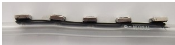
図 3.5 Magnet powdered wire without iron powder. Magnets of MPW are arranged with a spacing of approximately 2.5 [cm] and fixed on a tube with screws, which also have the role of electrodes.
